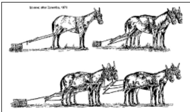
Fig. 3-38: Some harnessing options for horse-drawn carts involving (bottom) the use of front swingle trees. (Source: Barwell and Ayre, 1982)
