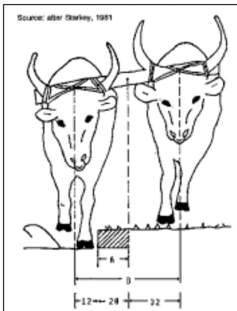
Fig 3-15: Illustration of relationship between yoke size, share size and line of draft.
