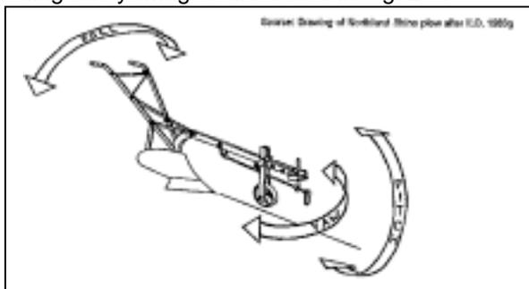
Fig. 2-8: Three possible rotations: rolling, yawing and pitching.
