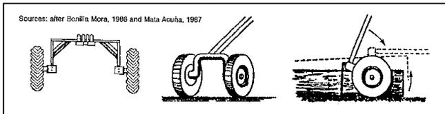
Fig. 9-42: Simple forestry sulkies for moving large logs with oxen in Cost Rica.
