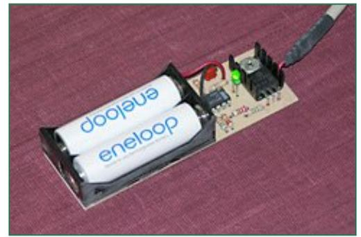
Eneloop cells can be charged in any standard Nickel Metal Hydride (NiMH) charger, including this do-it-yourself USB-powered one.
