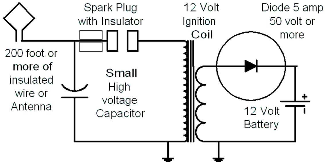
The description did not use a diode in the charging circuit, but did specify using an old model-T ford coil. When one uses a more commonly available ignition coil a low voltage diode is needed to keep from discharging the battery. If the coil is hooked up without the diode, flow would start immediately and soon discharge the battery. The diode limits flow in one direction to charge the battery.
