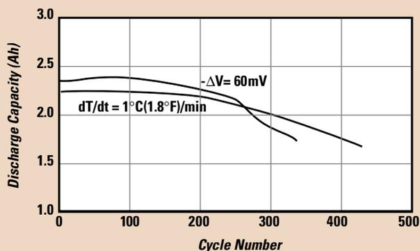
Cycle life and capacity of DURACELL DR30 Ni-MH batteries as a function of charge termination.
