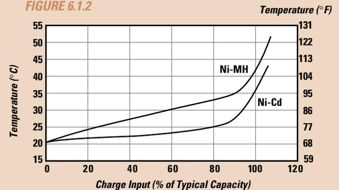
Typical charge temperature characteristics of Ni-MH and Ni-Cd batteries.
