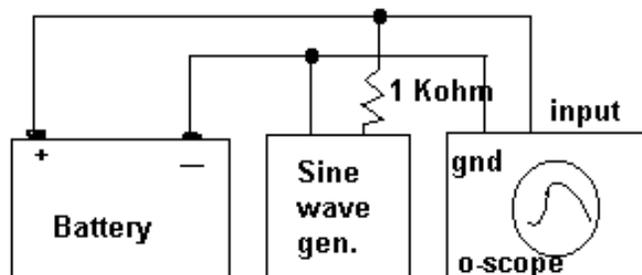
**Vary the sine wave source over a range of one to ten megahertz, and look for the peak in the response, showing electrolyte resonance.**
