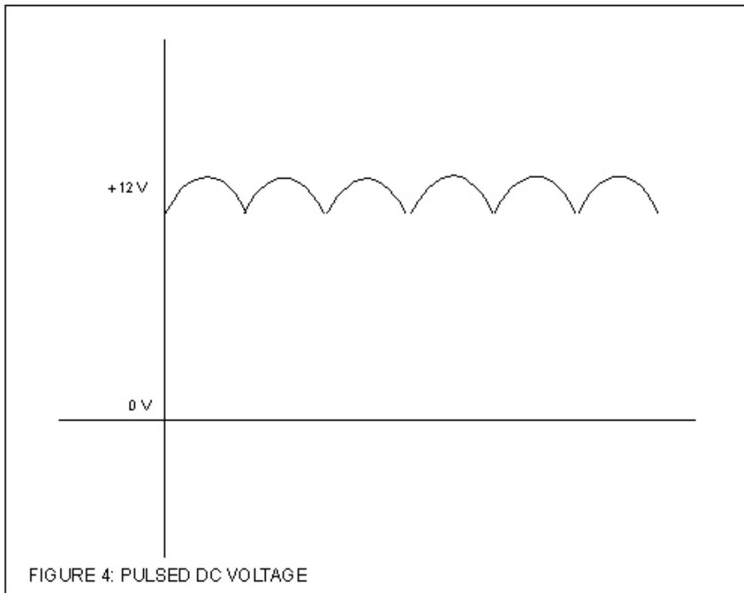
Surprisingly enough, the output of the alternator is not a pure D/C as one might expect, but a pulsating D/C. Because there are three windings, each with a positive and a negative half, by the time the voltage is passed through the diodes, there are six pulsations for each rotation of the rotor. This is close enough to D/C for most automotive components. Critical components, such as radios, have their own internal filtering circuits to further smooth out the waveform to a purer D/C.
