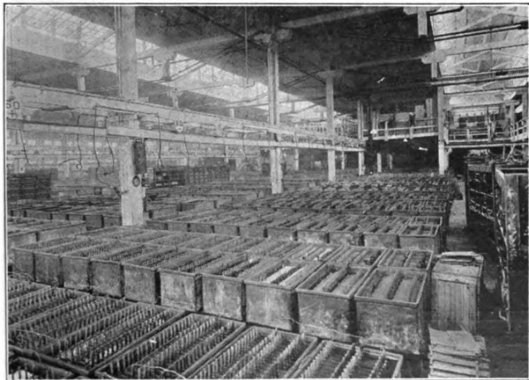
Fig. 41. Forming Room in the Willard Storage Battery Co. Factory
