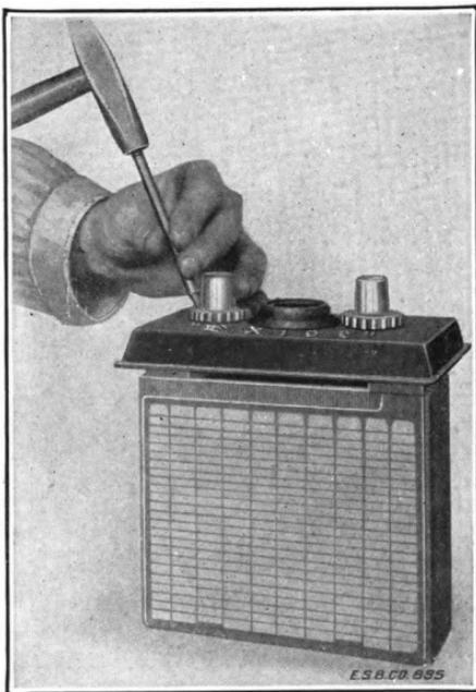
Fig. 179. Locking Sealing Nut
