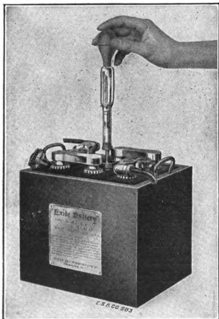
Fig. 33. Taking a Specific Gravity Reading
