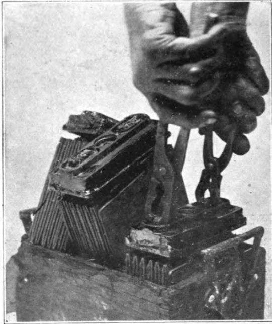
**Fig. 165. Lifting Elements Out of Jars, and Resting on Edge of Case to Drain.**
