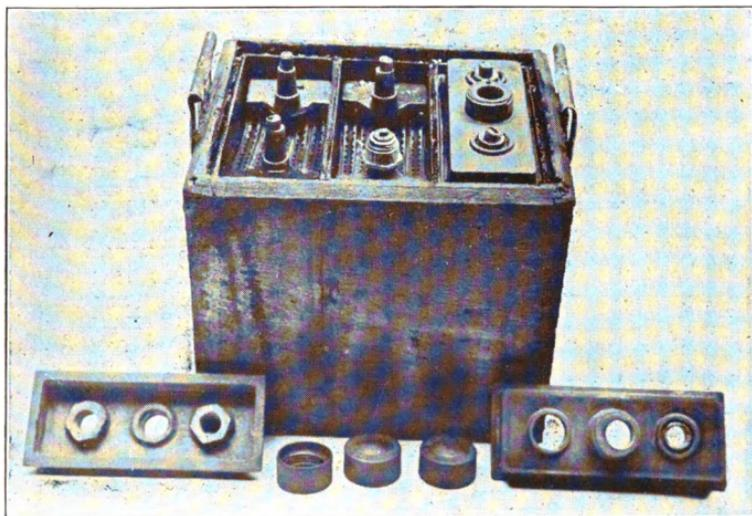
**Fig. 181. Prest-O-Lite Battery, Showing Parts and Construction**
