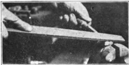
Fig. 154. Rasping Terminals and Connecting Links Before Burning In
