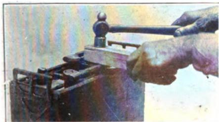
Fig. 129. Tapping Connectors in Place, Preparatory to Charging after Battery has been Opened and Shorts Removed
