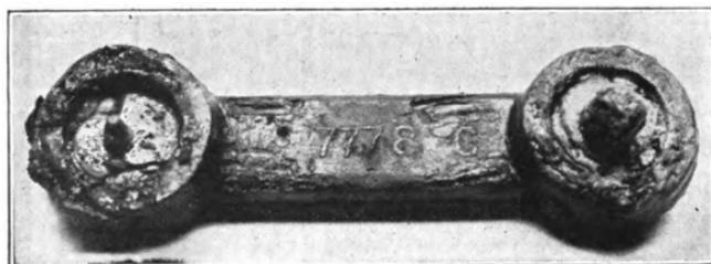
**Fig. 185. Under Side of Link Shown in Previous Figure. Note that Holes were Bored with a Wood-Bit**
