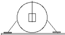
End view of the ammeter with the magnets aligned with the Earth's magnetic field.
