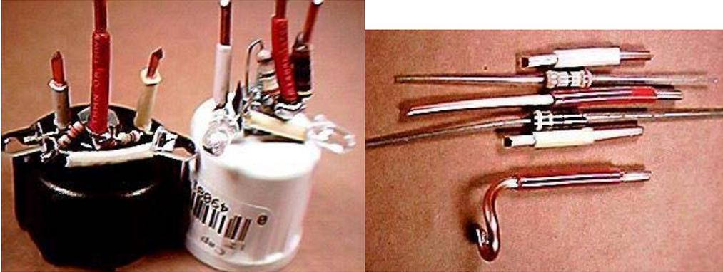
The positive and negative ends when finished then look like the following. Silicon rubber sealer was used to encapsulate the ends to add strength and durability in wet environments. Note the spiral spring in the negative cap. This came from an old battery pack.
