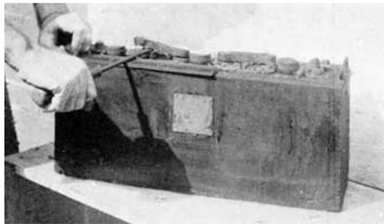
Fig. 193. Prying Off Cell Connector
