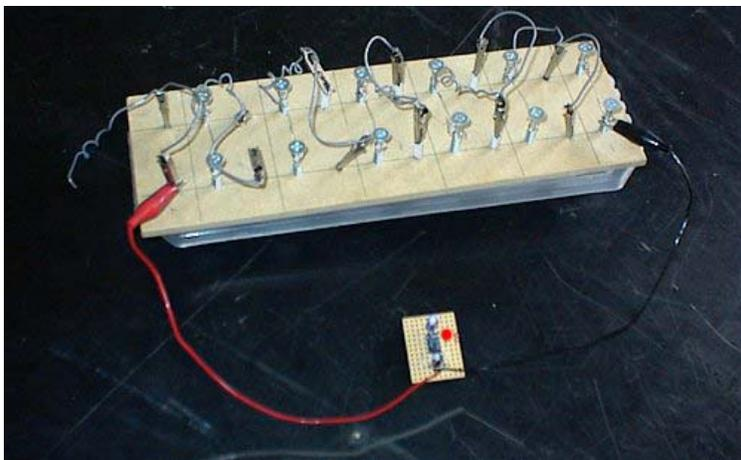
**Figure 3. The complete 'high' voltage, 'low' current sea water battery connected to an LED flasher circuit**
