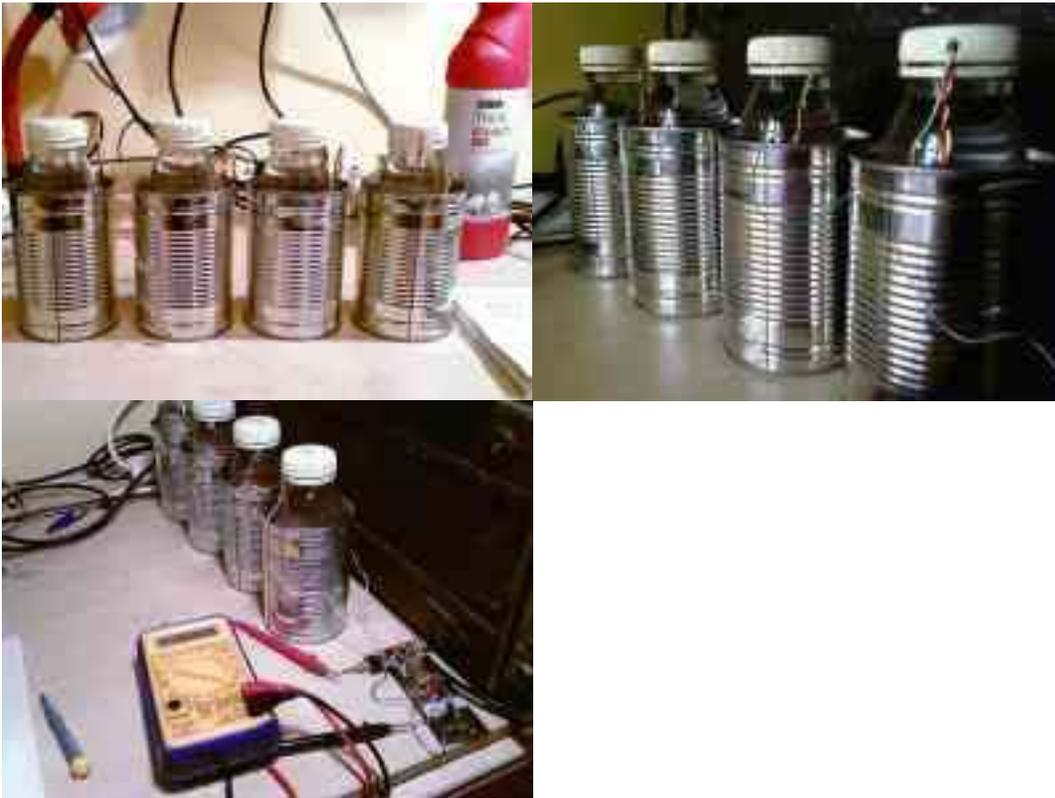
I built FOUR of these baked bean can cells, and connected them in series. One 750ml bottle of ASDA thick bleach costs 60 or 70 pence and is more than enough to fill all four cells and clean the toilet too. The voltage of the four cells is more than 3V. I connected the homebrew battery up to my [40m QRSS transmitter](#) - it's the circuit in the bottom right corner of the photo, 3'rd from left. That circuit is built on a baked bean can tin substrate too!
