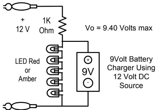
9 Volt Alkaline, NiMH and NiCD efficient Charger
