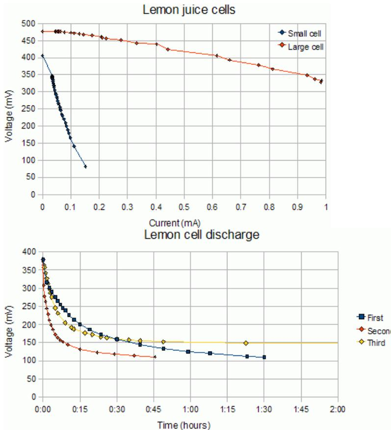
The first graph (above left) shows the voltage vs current of both the small lemon juice cell (see above) and my larger cell (this section). The large cell shows a massive improvement. It can cope with a 1mA current draw, and the voltage drops only to 324mV. This is a power production of 322uW, which is 19 times better than the small lemon juice cell!
