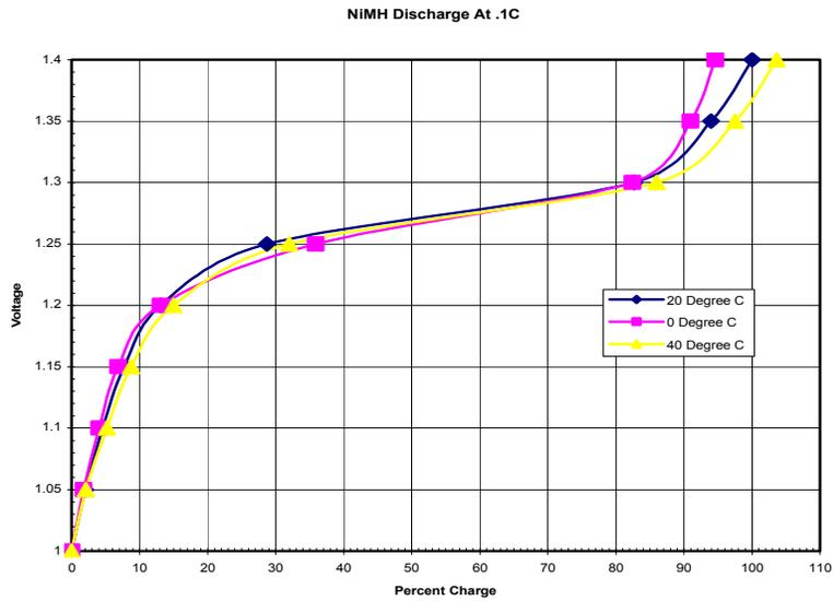
Typical NiMH C/5 room temperature discharge curves
