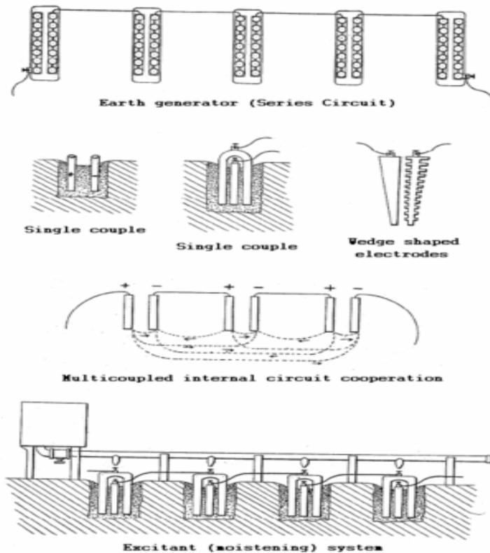
M. Emme, "U.S. Patent 495582 Ground generator of electricity".
