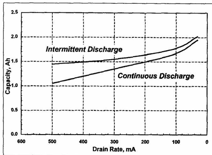
The above shows the Initial Capacity of RAM AA Cells as Function of Discharge Rate.
