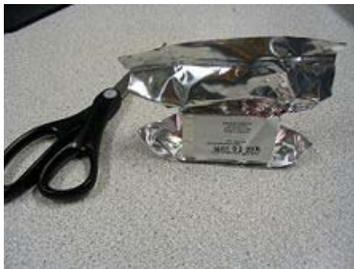
Radiosonde battery still in protective wrapper
