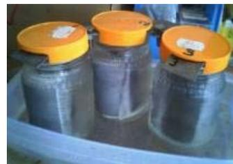
So back to charging.... I am not getting very much charging current... the positive should go rust coloured from  $\text{PbO}_2$  formation. Perhaps this is due to the lack of spongy lead which will hopefully form after repeated charge/discharge cycles (thereby hugely increasing the surface area).
