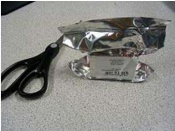
Radiosonde battery still in protective wrapper
