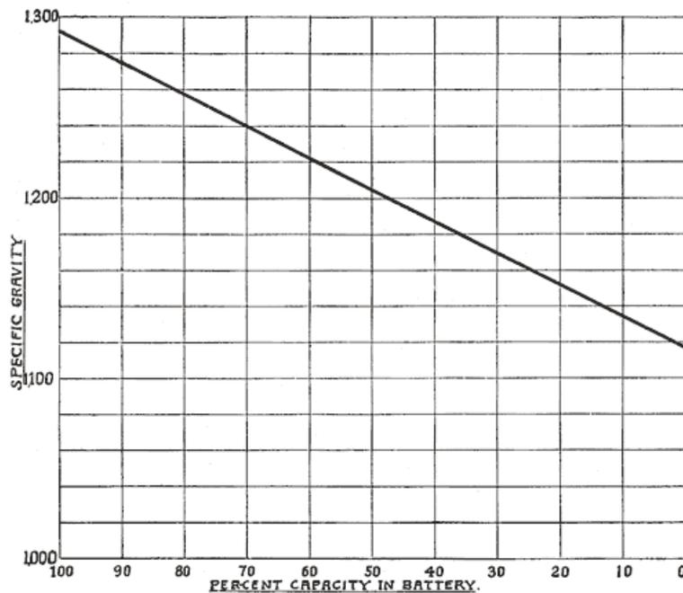
Fig. 23. Variation of Capacity with Specific Gravity
