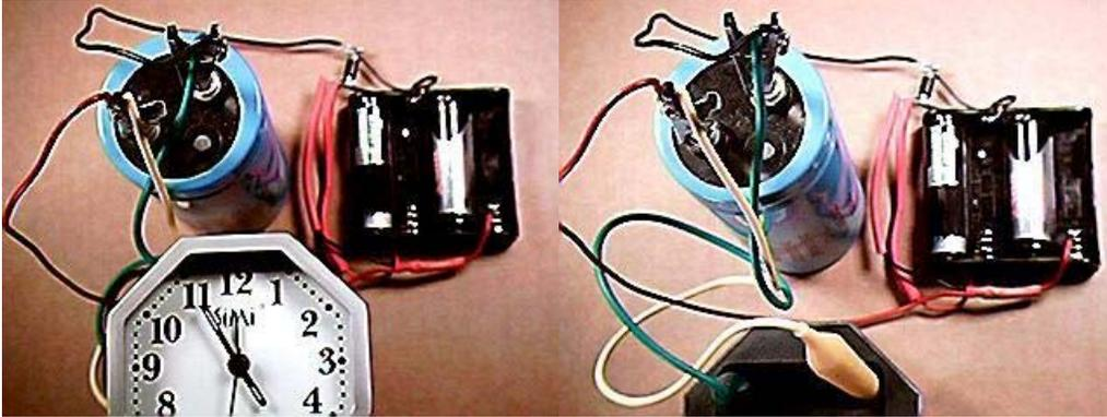
The cell with the black tape around it in the above picture is the helper source cell. The one being tested is next to that. The holder will work with AA or AAA cells being tested. Determine measured capacity “C” from measured discharge time and R1 the load resistor.
