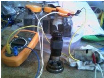
Hmm, the same cell cell shorted itself out again (voltage drops to zero almost immediately charging voltage is removed). I unwrapped it again, and it seems the glass fibre mat is not a good separator. It had
