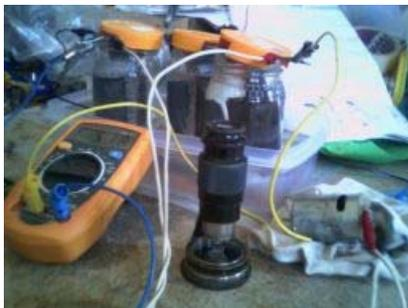
Hmm, the same cell shorted itself out again (voltage drops to zero almost immediately charging voltage is removed). I unwrapped it again, and it seems the glass fibre mat is not a good separator. It had
