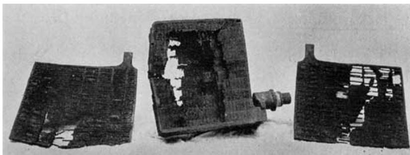
Fig. 210. Disintegrated Positives
