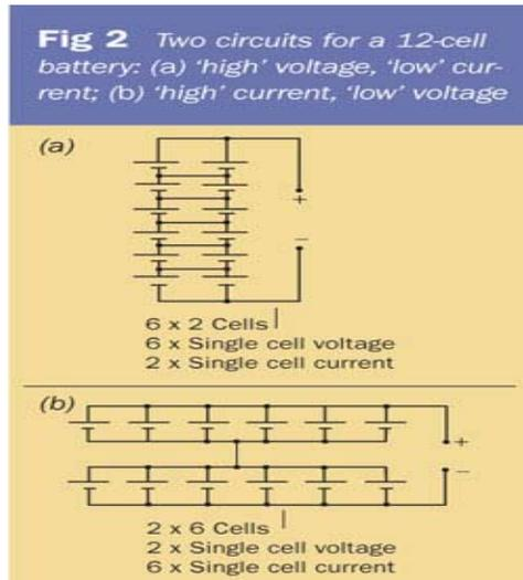
The battery circuit in *Fig 2(b)* will work well for devices that need a 'high' current but not a particularly large voltage. A good example would be a low-voltage 'solar cell' motor that will run on about 1 V, but needs >10 mA to turn. *Figure 3* shows a flashing LED circuit wired to the battery. This circuit requires about 3 V, at only 1 or 2 mA, to work.
