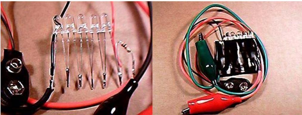
The leads are soldered as show above. Electrical tape is then wrapped around the bare leads. Out of about 10 Cells repeatedly charged and discharged on the average about 3 or 4 times. I had two that would not hold a charge after a short period of use. Both were the same brand Toshiba Alkaline. Duracell and Fuji both worked much better. Brand and possibly batch has a lot to do with rechargeablity of Alkaline cells.
