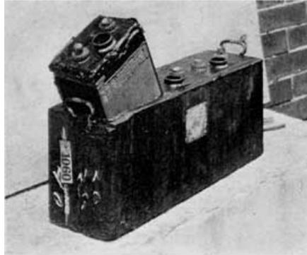
Fig. 197. Resting Element on Jar to Drain
