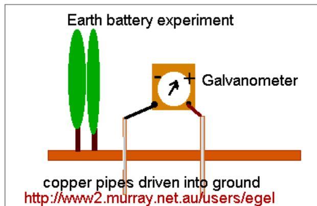
If you want to try it then get two copper rods or pipe and drive them into the ground and then connect a galvanometer(place them near a tree for better results.) apparently the needle always points positive although it may take time for the current and voltage to build up.
