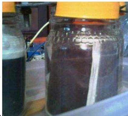
2 was weak, so I replaced the plate with a fresh sheet of lead. While busy, I couldn't resist jabbing holes in both sides of the plates with a clean compass point, and also scratching crossed diagonal lines into both sides. Hopefully this will increase the initial surface area, and allow the sponge-forming to penetrate more deeply.
