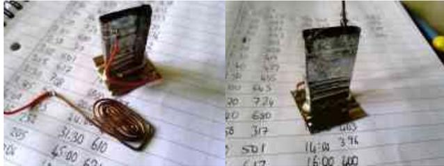
To construct the other electrode, I used about 25cm of copper wire, wound into a flat spiral. The copper wire is household lighting cable, with the insulation stripped off. To keep the electrodes apart, I wrapped the copper spiral in a piece of kitchen tissue. Then poured in lemon juice squeezed directly from a lemon. The idea here, is to increase the surface area of the electrodes and decrease the distances involved, to reduce the internal resistance of the battery.
