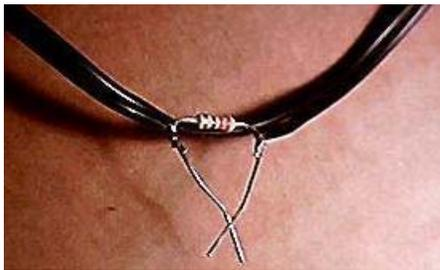
When fast charging is needed the resistor leads are connected together and the resistor is effectively taken out of the circuit. In the above example we used a 220 ohm resistor. One way to find the right value of resistance is to temporarily hook up a digital amp meter and a variable resistor (pot) and adjust the flow to be about 100 times less current than what is measured when the pot is zero ohms. Then measure the resulting resistance using a digital ohm meter.
