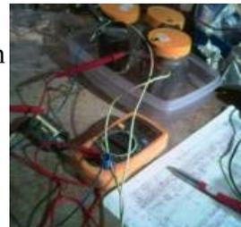
So following a sort-of pattern of allowing the charge voltage to rise to over 8V, and then running the motor, then charging again gave the following results. Sometimes I shorted the battery out after the motor stopped. In all cases, the positive plate stays much darker than the negative, meaning PbO<sub>2</sub> remains on the positive plate. To get maximum surface area, should all the PbO<sub>2</sub> be converted to PbSO<sub>4</sub> after discharge? [Any ideas or suggestions?](#)
