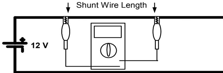
If an analog meter is used that is close to 1 ma full scale (meter movement about 81 ohms) and planned to be used to measure 20 amps full scale instead of a digital meter, then multiply the length found above by a factor of 4. For other configurations see: <http://www.uoguelph.ca/~antoon/gadgets/shunts/shunts.html>
