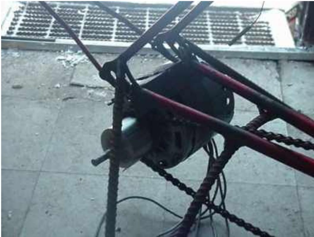
The sprocket was welded to a hub which fit the shaft of the generator. A design improvement would probably be to have a flywheel on the same shaft as the generator. The generator fit into a bracket which we welded near the back of the bike (approx where the rear wheel was). We welded "feet" together out of some re-bar left over from a concrete project. Another design improvement would be more rigid feet. The feet were welded to the back of
