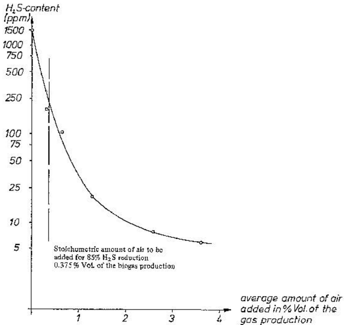
b) H<sub>2</sub>S reduction from initially 1500 ppm as a function of added air.
