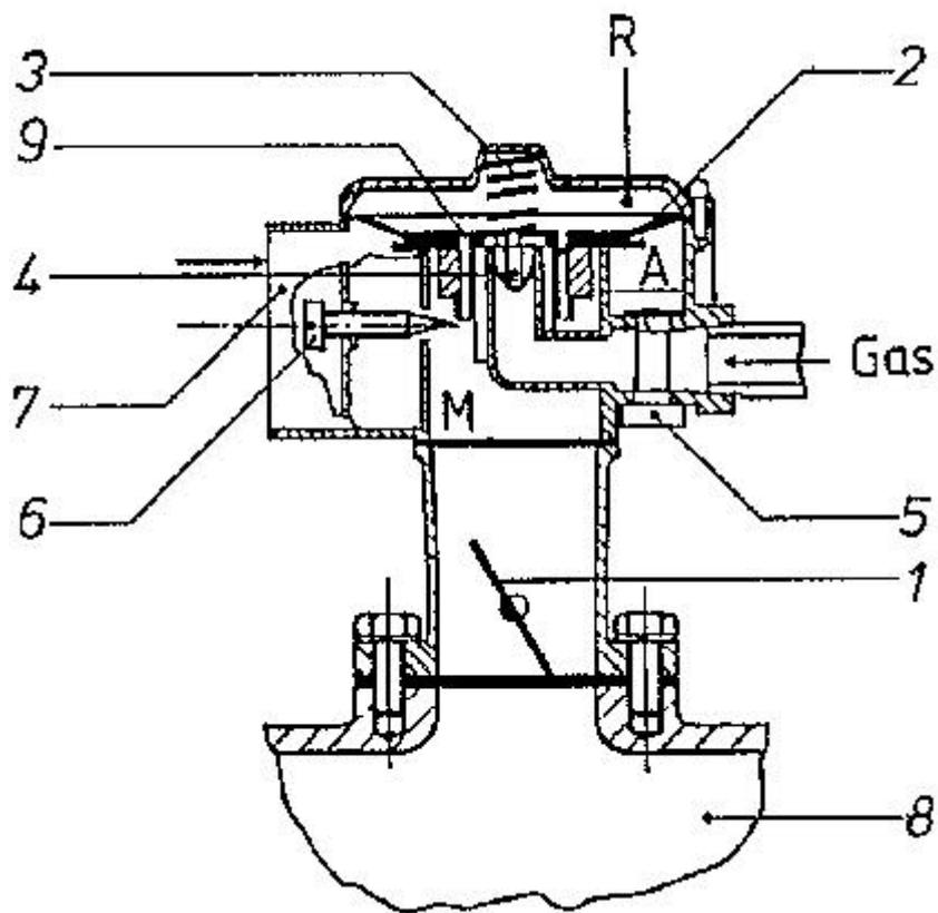
Fig. 6.6: Cross-sectional view of gas mixing valve.
