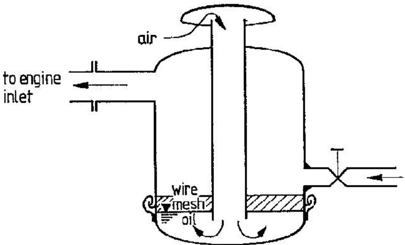
Fig. 5.3: Air filter modified into mixing chamber
