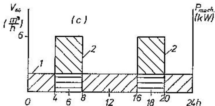
Fig. 7.5: Daily production and demand profiles for the example. - biogas production directly consumed. /// excess biogas production for storage, \biogas drawn from store to cover for actual shortage.
