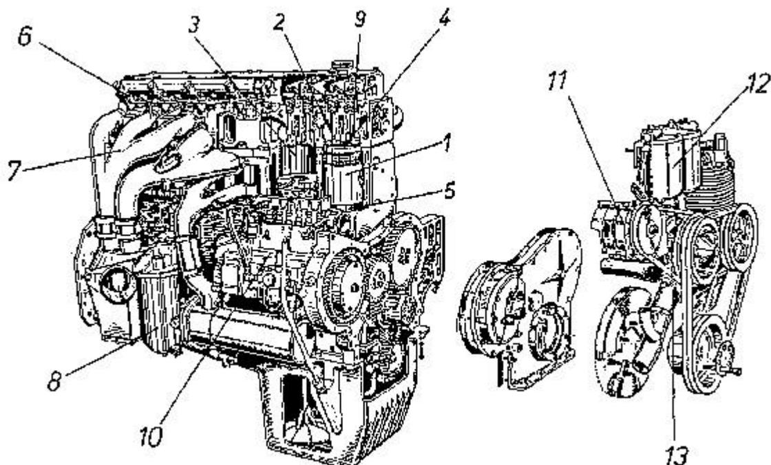
Fig. 3.7: 6-cylinder diesel engine, partly opened (MAN).
