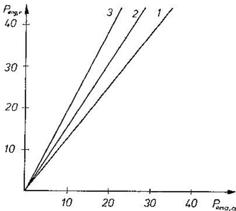
Fig. 7.8: Relation of rated power of engine (before modification),  $P_{eng,r}$  and its actual power output  $P_{eng,a}$  at optimal economic conditions with biogas. Operational speed = 0.8 X max. speed. 1 diesel gas (dual fuel) engine operating short periods only, 2 as 1 but operating continuously, 3 Otto biogas engine, continuous operation.
