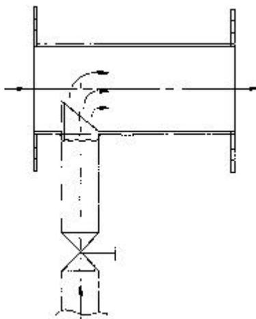
Fig. 5.4: T-joint mixer with oblique, protruding gas inlet
