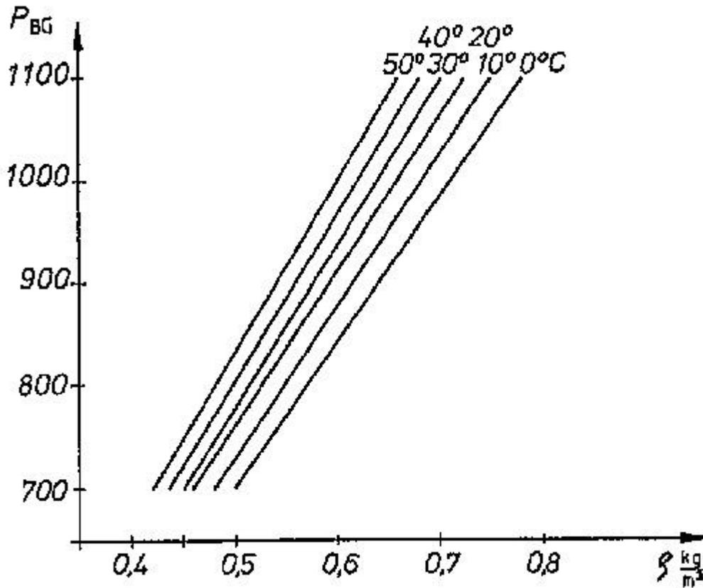
Fig. 4.1: Density  $r$  of  $CH_4$  as a function of biogas pressure and temperature
