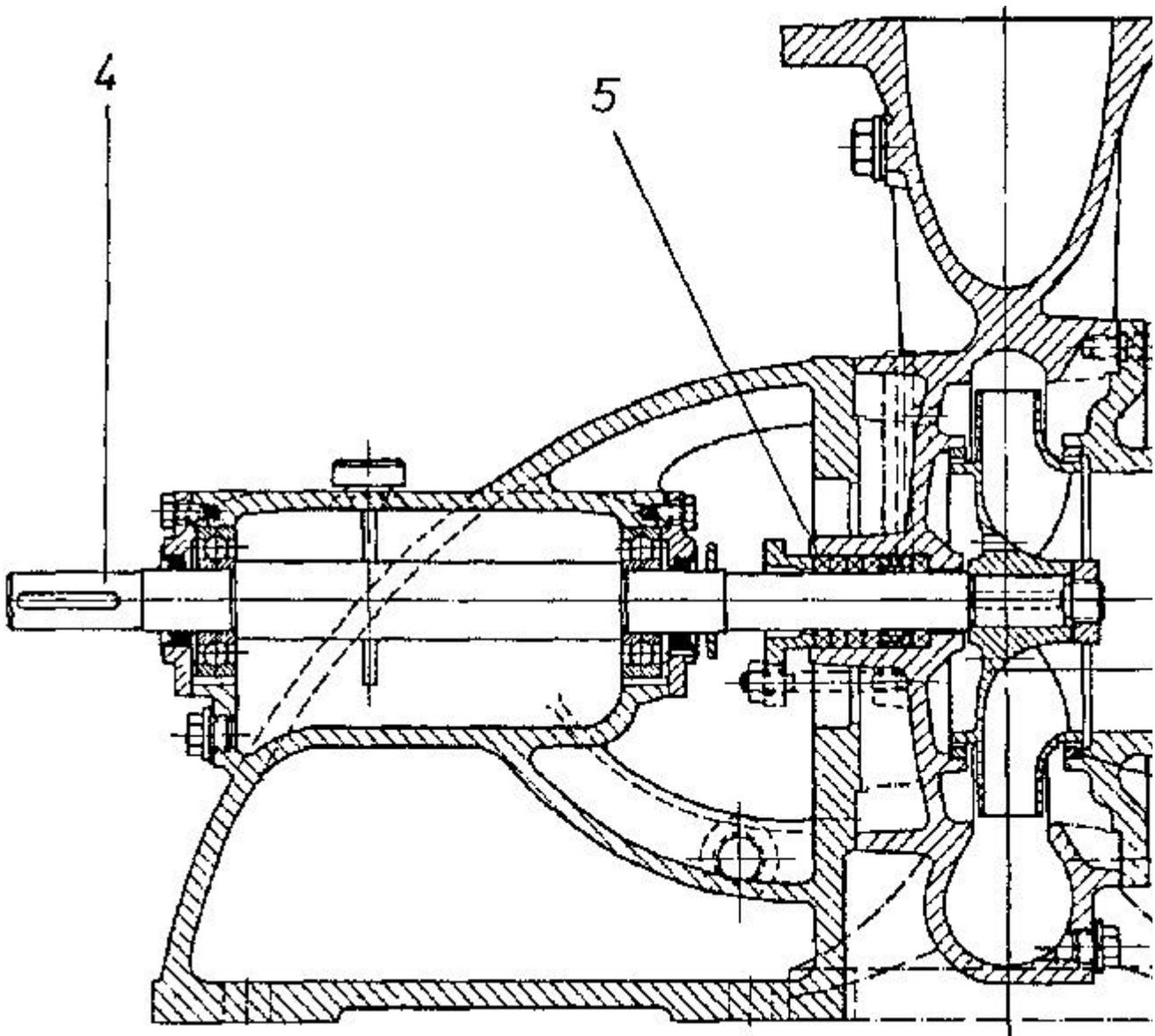
Fig. 7.11: Cross-sectional view of single-stage centrifugal pump (KSB).
