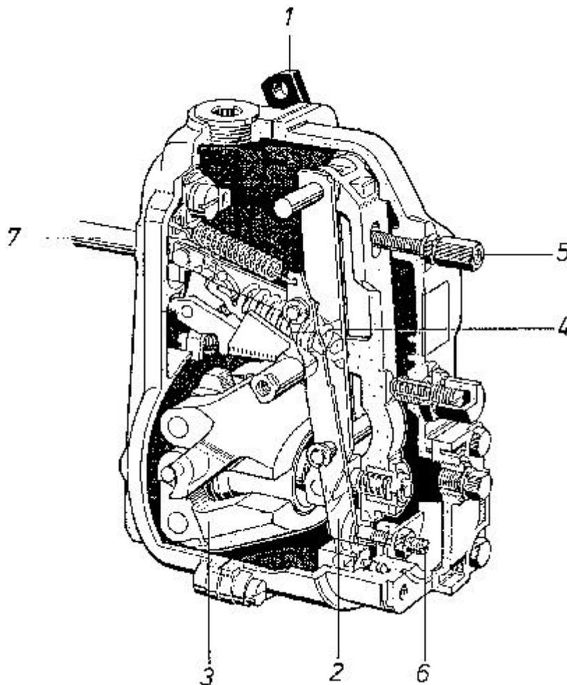
Fig. 5.8: Governor for diesel fuel injector pump (Bosch).
