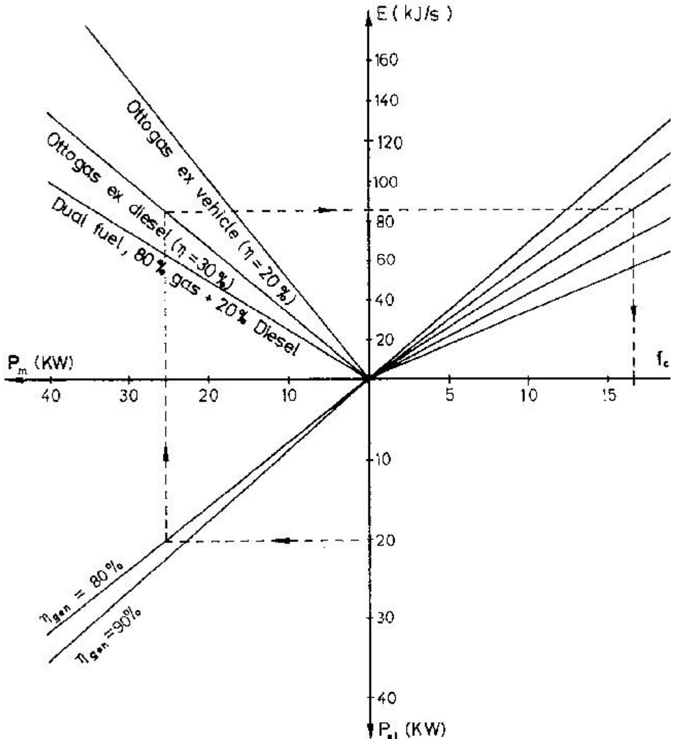
Fig. 7.9: Nomogram for the relation of fuel consumption/fuel demand  $f_c$ , biogas quality  $\text{CH}_4\%$ , fuel energy flow  $E$ , type of engine used, mechanical power output  $P_m$ , electric generator efficiency  $\eta_{gen}$ , and electric power output  $P_{el}$ . Basic gas data assumed: temperature  $25^\circ\text{C}$ , pressure 960 mbar, ref. humidity 100%.
