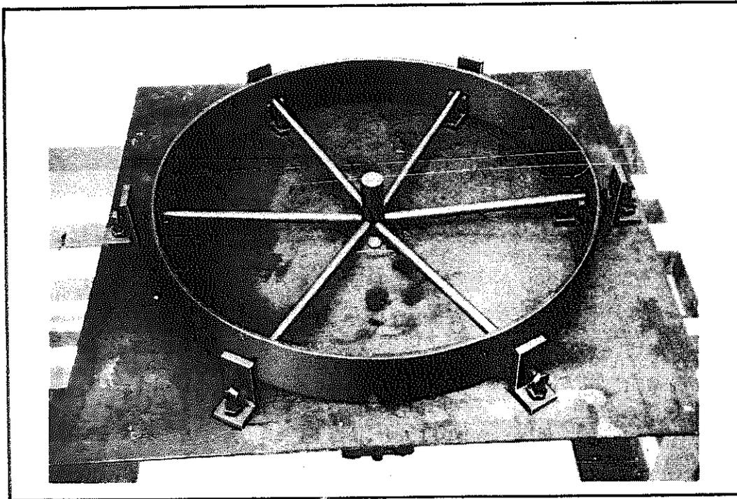
The wheel rim adjuster bolts are slackened off, the wheel lifted to clear the spoke rests and turned  $30^{\circ}$ , then lowered to the jig deck. (Note: the two bolts securing the upper axle guide have their heads cut down to  $1/8''$  (3 mm) in height to avoid their catching on the spokes when the rim is turned  $30^{\circ}$ ).
