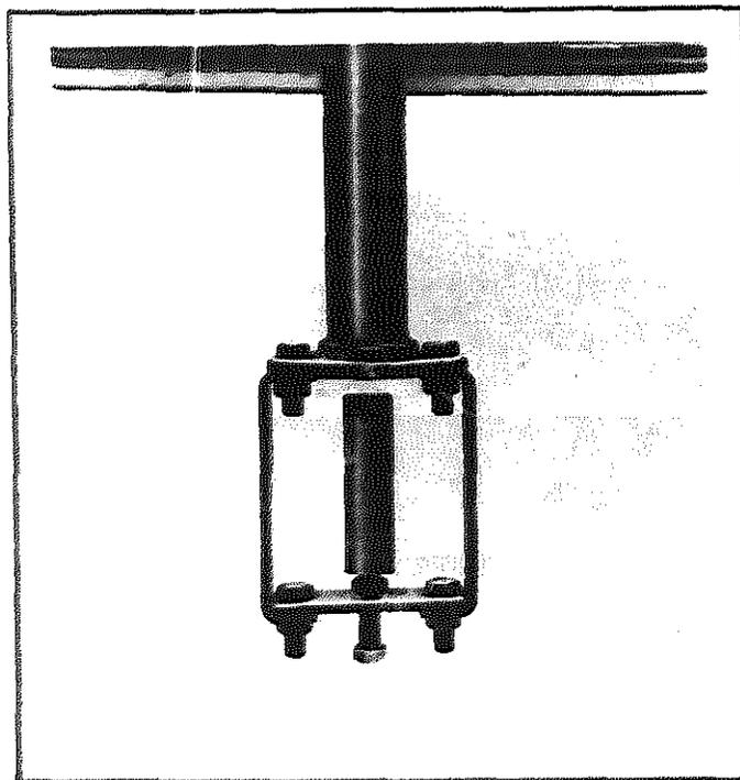
The wheel rim is replaced in the jig, and the axle is inserted down through the upper axle guide (QR) and the lower axle guide (R), the axle end resting on the axle position adjuster bolt (R) the latter then being screwed up or down as required to bring the top of the axle in line with the plane across the upper edge of the wheel rim.
