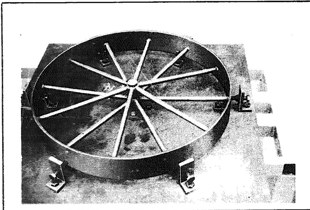
The remaining six alternate wheel spokes are laid in the spoke guides with their inner ends resting on suitably dimensioned distance pieces to position their upper edges at  $\frac{1}{2}$ " (12.5 mm) from the end of the axle, followed by tack welding to wheel rim and axle.
