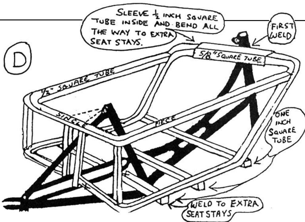
don't be afraid to flatten the stay a little - bike tubing is very strong. However this should not be necessary.
