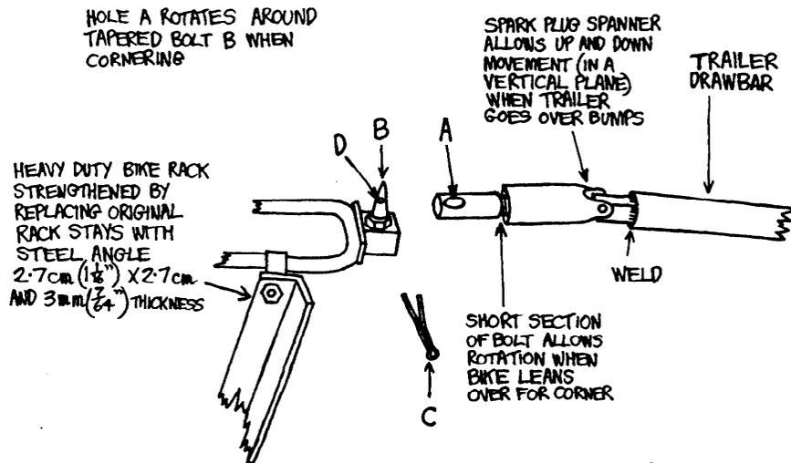
Hole A is slipped over tapered bolt B, then split pin C is inserted through hole D. Split pin holds trailer coupling on towbar, and provides easy 'no tools' quick release of trailer, Split
