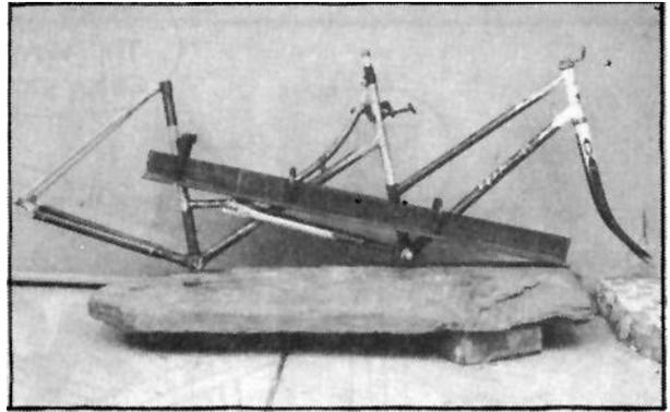
weld. (If stays are long enough weld onto curved top tube as well for extra strength).
