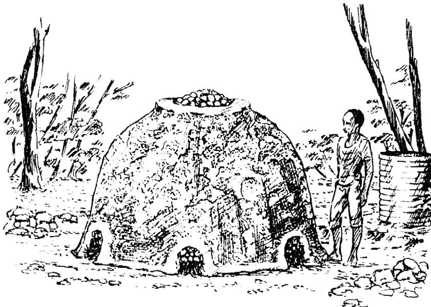
*A heap covered with clay daub.*
