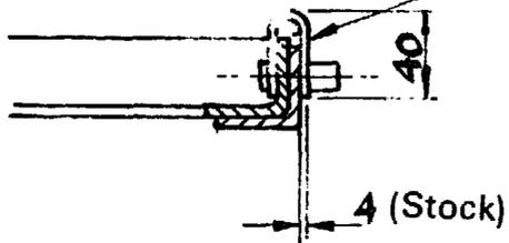
Item (16) is to be folded so that a tight fit is obtained when fitted over items (4) and (5) as shown
