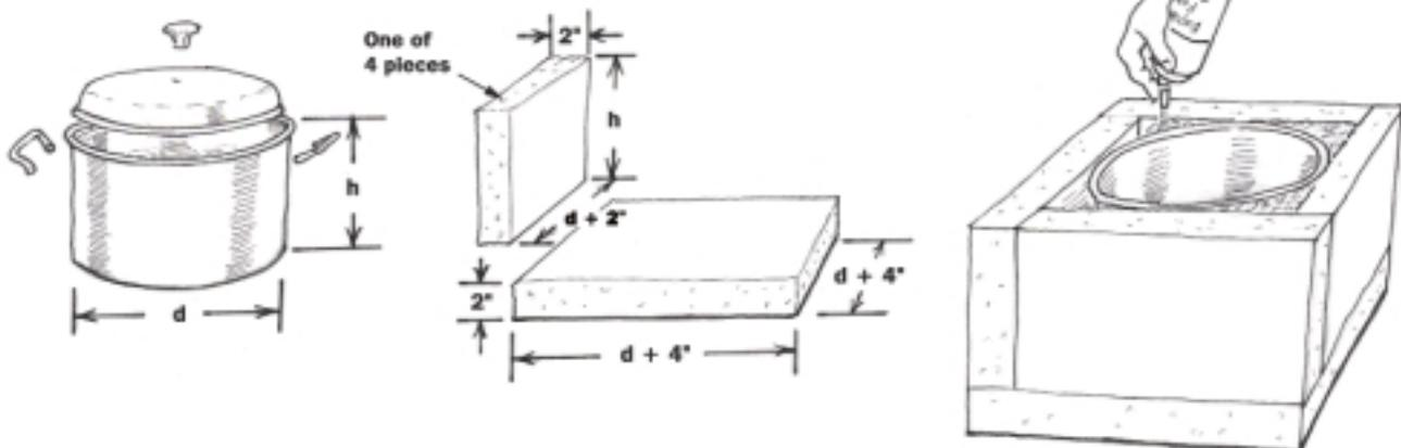
**Figure 1:** Cut and glue together five pieces of two-inch styrofoam pieces, insert well-waxed pot after removing the handles, and fill empty spaces with expanding foam insulation. Note the dimensions of the five foam pieces.
