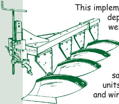
This implement is used to turn sods up to 300 mm depth and is particularly useful on heavier well-structured soils. Turning the soil also has the advantage that weed seeds and unwanted crop residues can be buried deeply. Mouldboard ploughs are not recommended on sandy soils, because poorly-structured units which may exist, can be destroyed and wind erosion be promoted.
