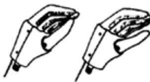
instead of hooks, an artificial hand with a thumb that opens and closes against 2 fingers (expensive and may not last)
