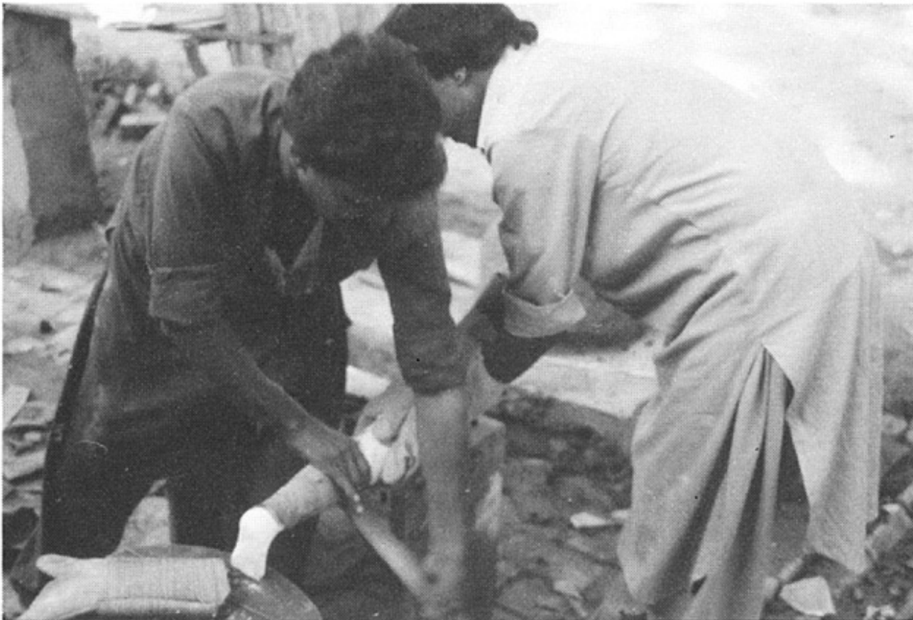
When the plastic is hot and soft, workers drape it over the plaster leg mold. Then they wrap it tightly with strips of rubber inner tube until it hardens. (See p. 552.)
