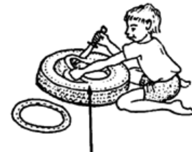
Rings for swinging and many games can be made by cutting out the inner rims of old car tires.
