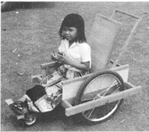
A wood wheelchair in Thailand. The bicycle wheel axles are supported on both sides to keep them from bending.
