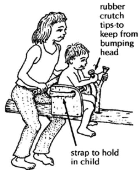
One end of this seesaw has an enclosed seat for a disabled child. Space is left behind the seat for an able-bodied child to sit and protect the disabled child.
