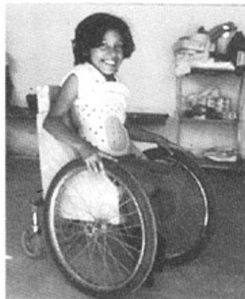
A wheelchair made completely of paper, including the wheels. Paper is glued together using rice flour in water (Zimbabwe).
