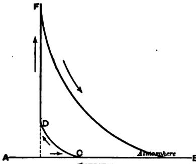
Fig. 121.—Diagram of Perfect Cycle with Compression.
