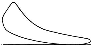
Fig. 74.—Second Lenoir Engine—Indicator Diagram.
