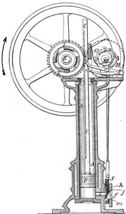
Fig. 9.—Otto and Langen Vertical Engine—
