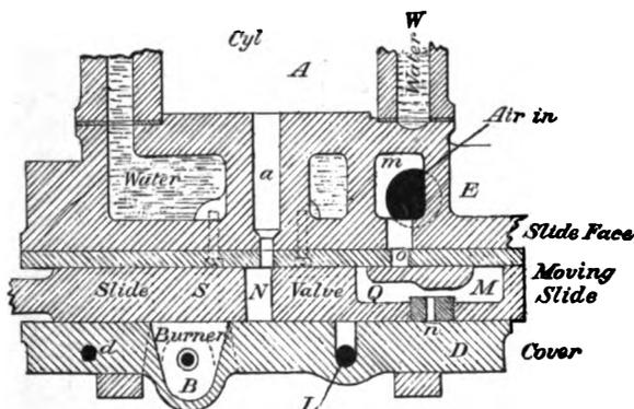
Fig. 37.—Otto Engine, 1876—Sectional Plan of Slide Valve.
