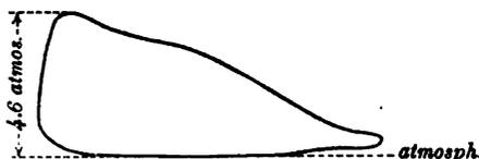
Fig. 18.—Simon Engine—Indicator Diagram.
