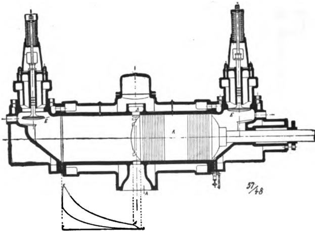
Fig. 84.—Koerting Engine—Section of Cylinder with Diagram.
