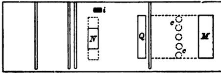
Fig. 38.—Otto Engine—Vertical View of Slide Valve.
