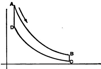
Fig. 115.—Stirling Cycle—Constant Volume.
