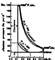
Fig. 28.—Atkinson Cycle Engine
