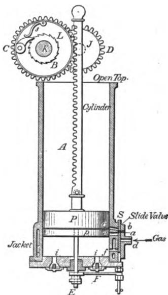
Fig. 2.—Barsanti and Matteucci's Gas Atmospheric Engine. 1854.
