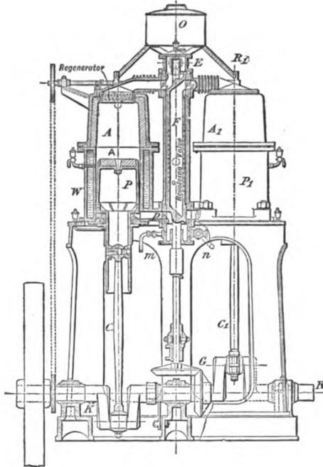
Fig. 130.—Siemens' Regenerative Engine. 1881.
