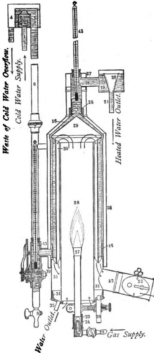
Fig. 118.—Junkers Gas Calorimeter. Sectional Elevation. 1899.
