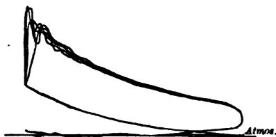
Fig. 137.—Hornsby-Akroyd Engine—Indicator Diagram.
