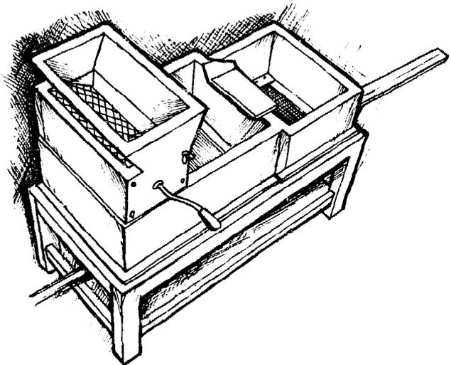
Dry dehullers, in which the beans are cracked between wooden rollers, have also been developed, but they are not as widely used since the grits they yield give tempeh with texture that is not popular in Indonesia; and while the grits are soaking, there is a relatively large loss of solid nutrients and protein.
