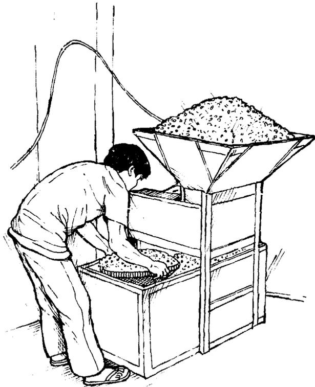
A low-technology dehuller-separator has been developed at the Bandung Institute of Technology. The beans are placed in a hopper and are then dehulled between a hand-turned scored wooden roller and a fixed plate, whence they fall into a large compartment into which water is piped from below. The beans sink onto a screen at the bottom of the compartment while the hulls float over a spillway with the overflowing water and are caught on a separate screen.
