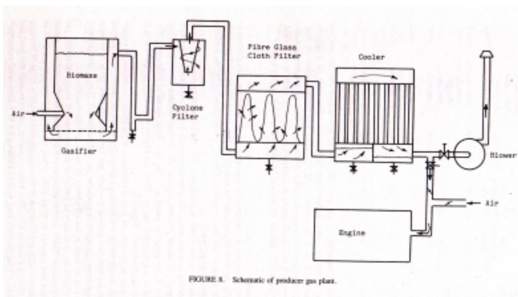
FIGURE 8. Schematic of producer gas plant.
