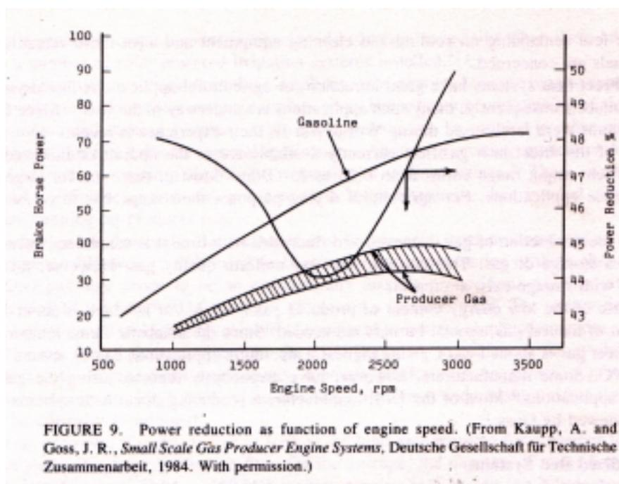
It should be noted that in general the overall efficiency of the IC engine itself does not change though the power derating takes place. However, detailed comparison of the engine efficiencies with and without producer gas has not been done till now because of insufficient data and large variations in producer gas composition<sup>30</sup>. Thus a conservative figure of 15-20% can be used as efficiency of spark ignition engines.
