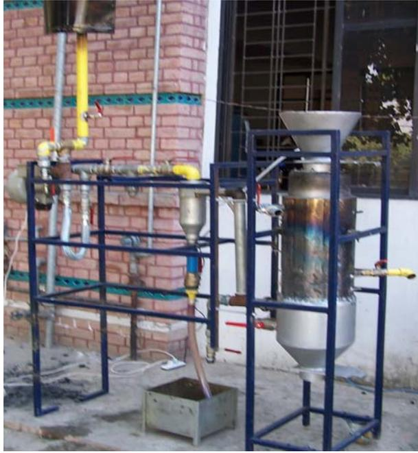
**Figure 3 Pilot scale HGL gasifier**
