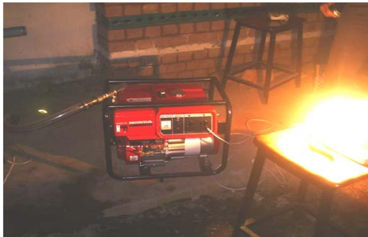
Figure 9 Synthesis Gas Operating the Engine
