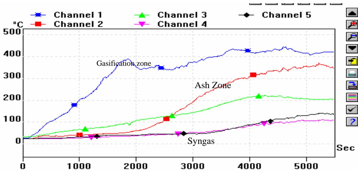
**Figure 8b Typical Temperature Log**
