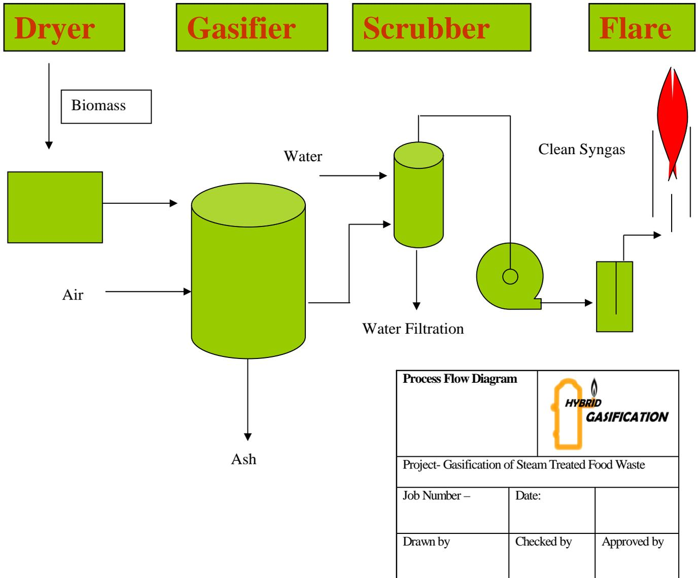
**Figure –4 PFD of Gasification Plant**
