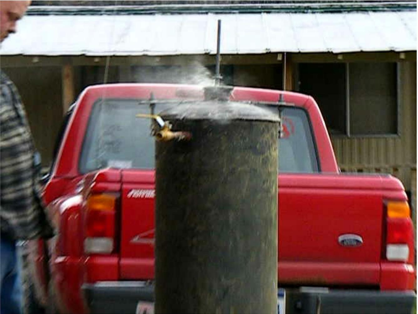
This is I believe smoke coming off the gaskets around the lid of the unit. This is a little pressure in the top and it is bleeding off around the pressure valve spring at the top. You can see some tar slipping up through there around the all thread.
