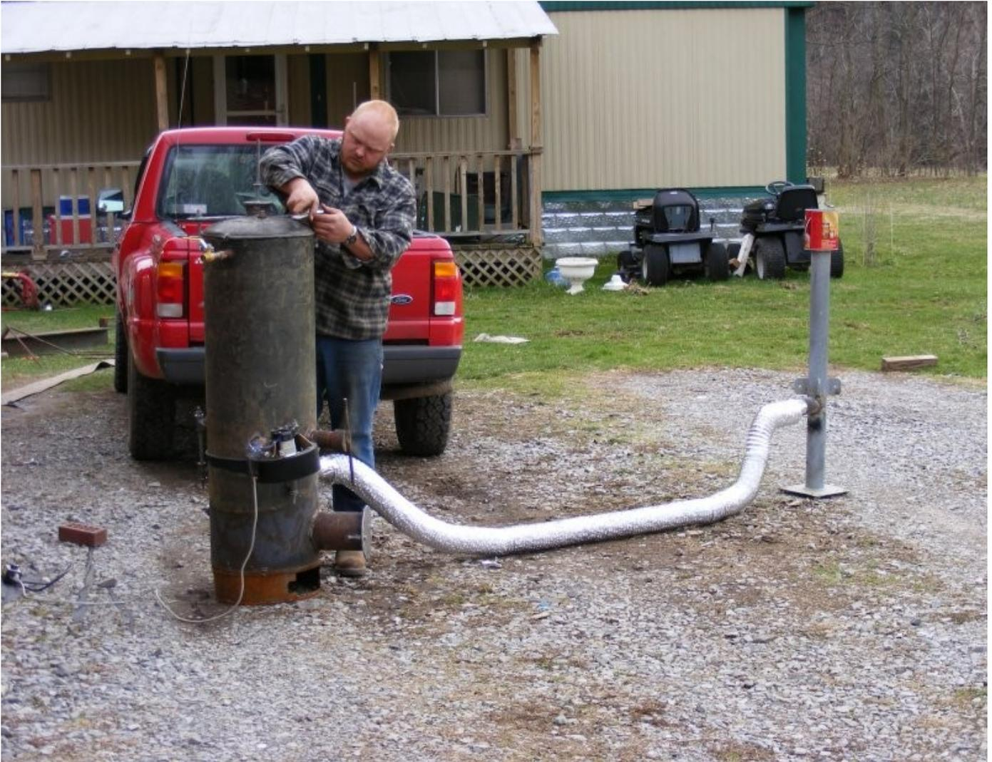
Ready to start the gasifier. Put in the charcoal up and to the nossels. This blower is on the intake of the air supply. It is a 285 CFM blower but we have a variable speed controller on the motor.
