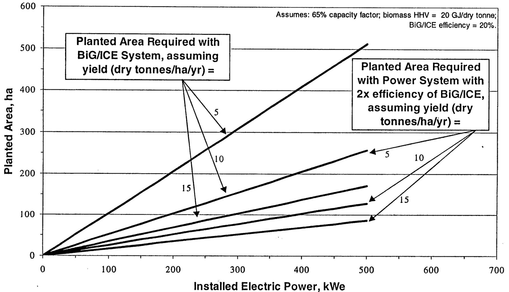
Fig. 10. Approximate planted area for energy crop production required to fuel gasifier-engine systems up to 500 kW<sub>e</sub> in size. Area requirements are shown for BiG/ICE technology and for future technology with double the efficiency of BiG/ICE systems. For each technology, the area is shown for crop yields of 5, 10, and 15 dry tonnes per hectare per year.
