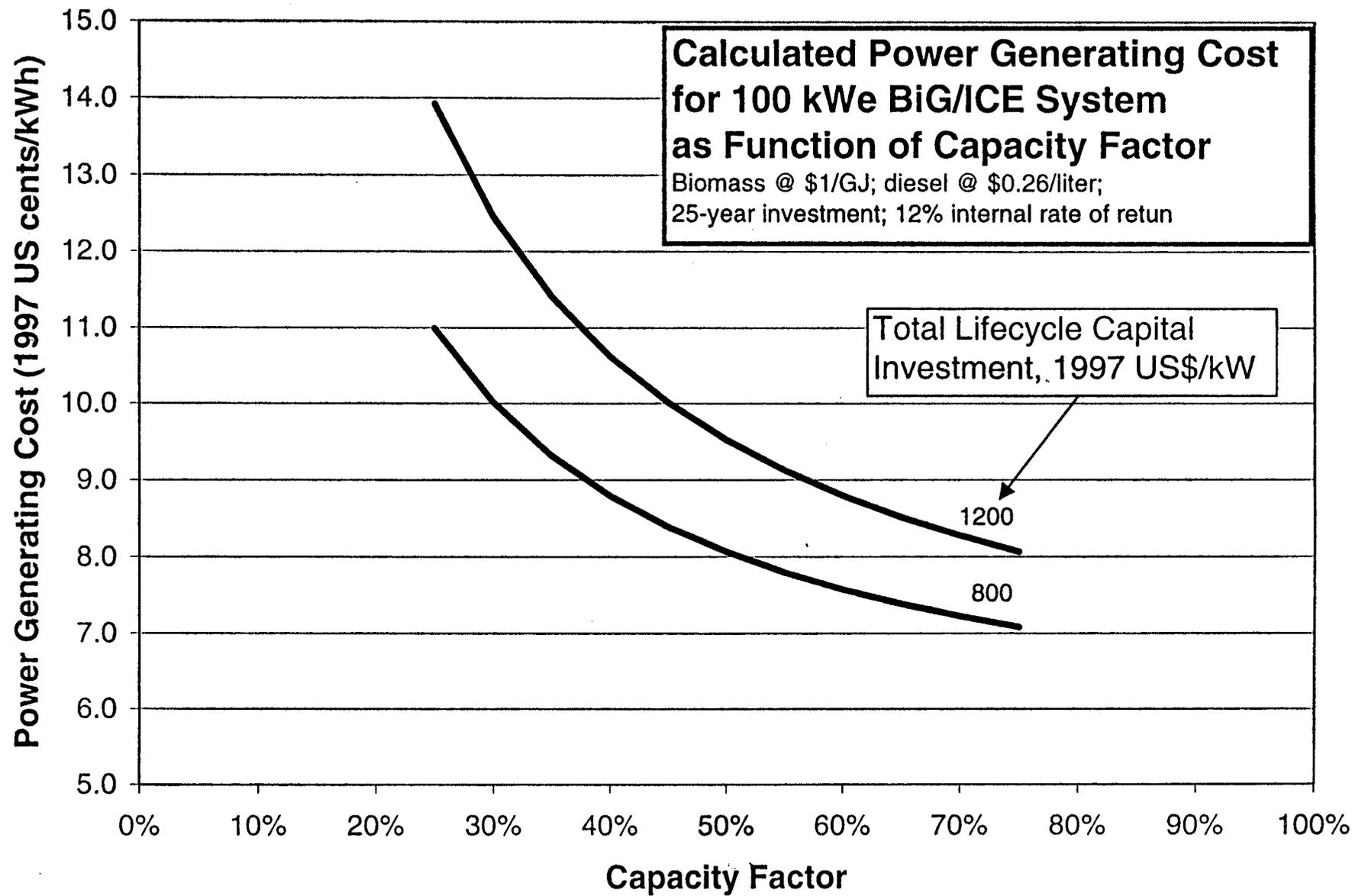
Fig. 13. Calculated electricity generating cost for 100 kW<sub>e</sub> BiG/ICE systems as a function of system capacity factor. Results are shown for two levels of initial capital investment. See Table I for additional details.
