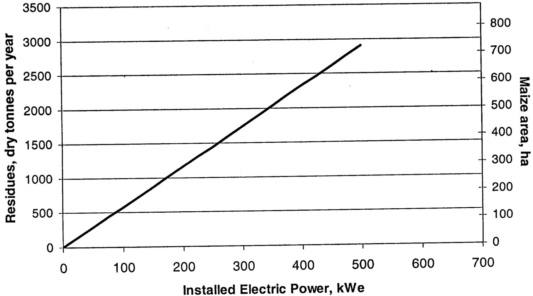
Fig. 6. Approximate maize residue requirements (and associated maize growing area) for biomass-gasifier/internal combustion engine power generation up to 500 kW<sub>e</sub> in size.
