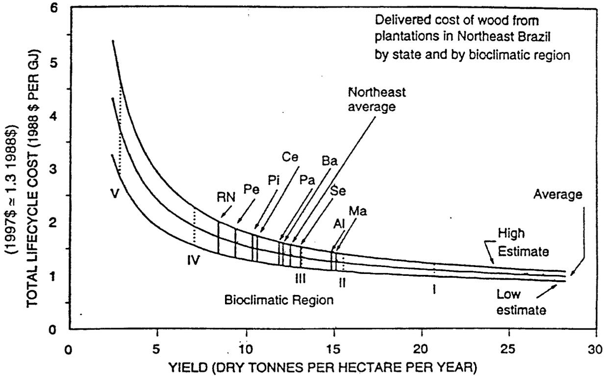
Fig. 9. Estimated potential cost-supply curve for biomass energy from plantations in Northeast Brazil [Carpentieri *et al.*, 1992].
