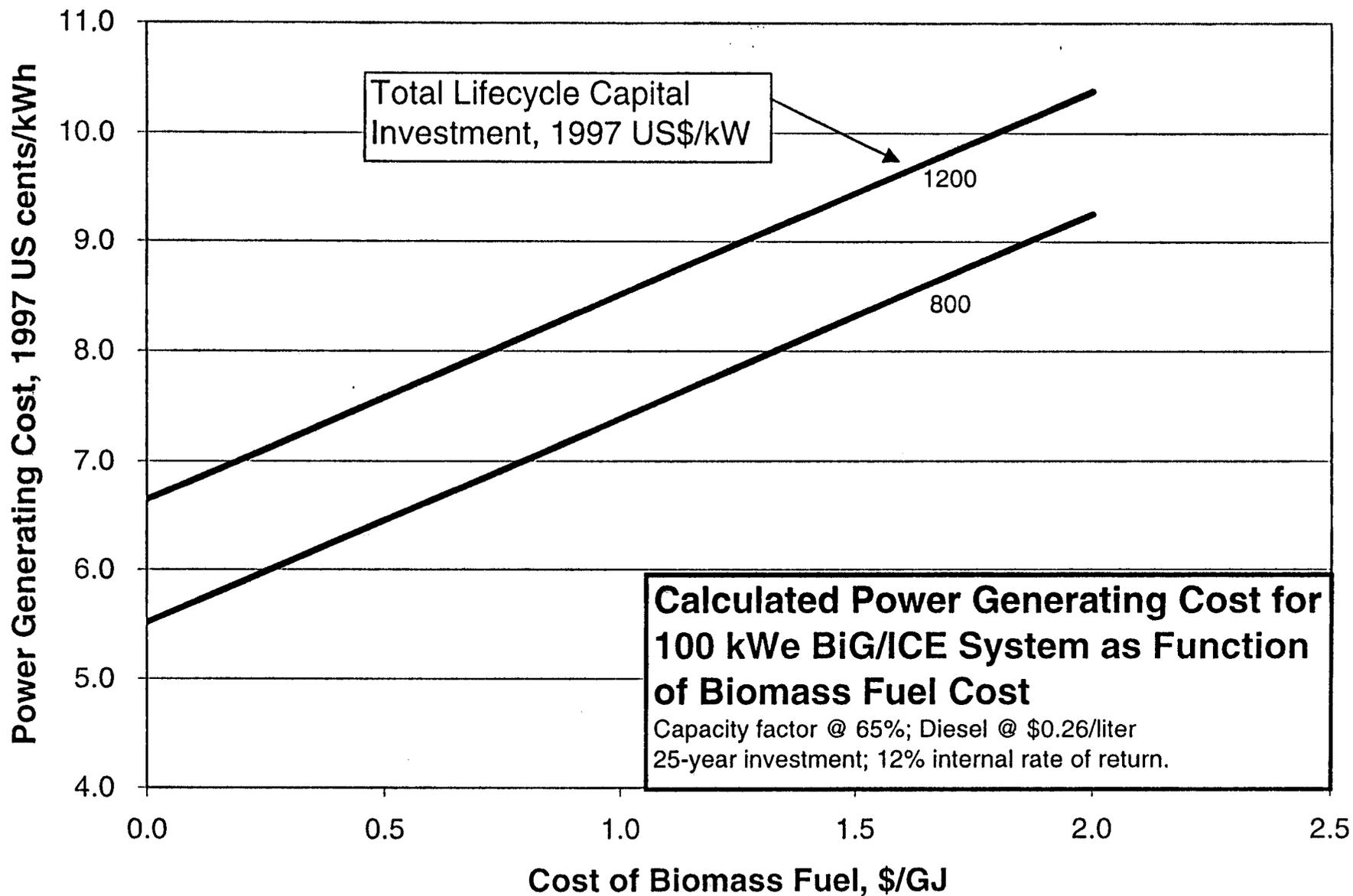
Fig. 14. Calculated electricity generating cost for a 100 kW<sub>e</sub> BiG/ICE system as a function of assumed biomass fuel cost. Results are shown for two levels of initial capital investment. See Table I for additional details.
