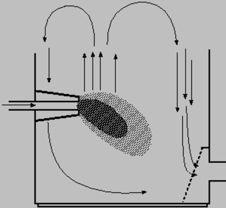
Figure 6: Regular charcoal gasifier operating at low power.
