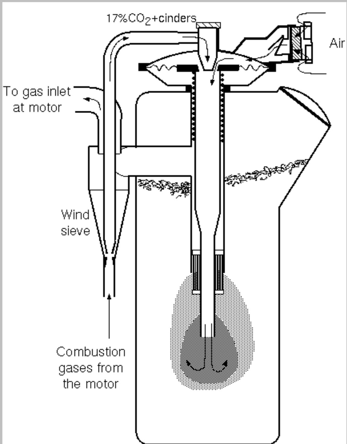
Figure 5: The final Källe-gasifier, complete with wind sieve.
