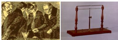
Shown on the left is a lithograph depicting Oersted's original demonstration and on the right is an 1851 example of an experimental apparatus to demonstrate this electromagnetic
