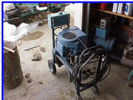
**Here is a new welder/generator that I've just finished in February, 2000. It is a 100 ampere DC welder, powered by a B&S 8 hp gasoline engine. Click on it to go directly to this welder page.**
