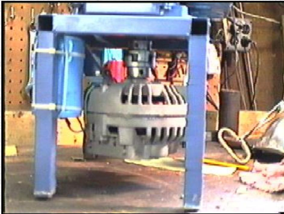
Front view of the alternator. Note the 89000uf filter capacitor (Blue cylinder behind the front left leg) used at the output to filter the output voltage.
