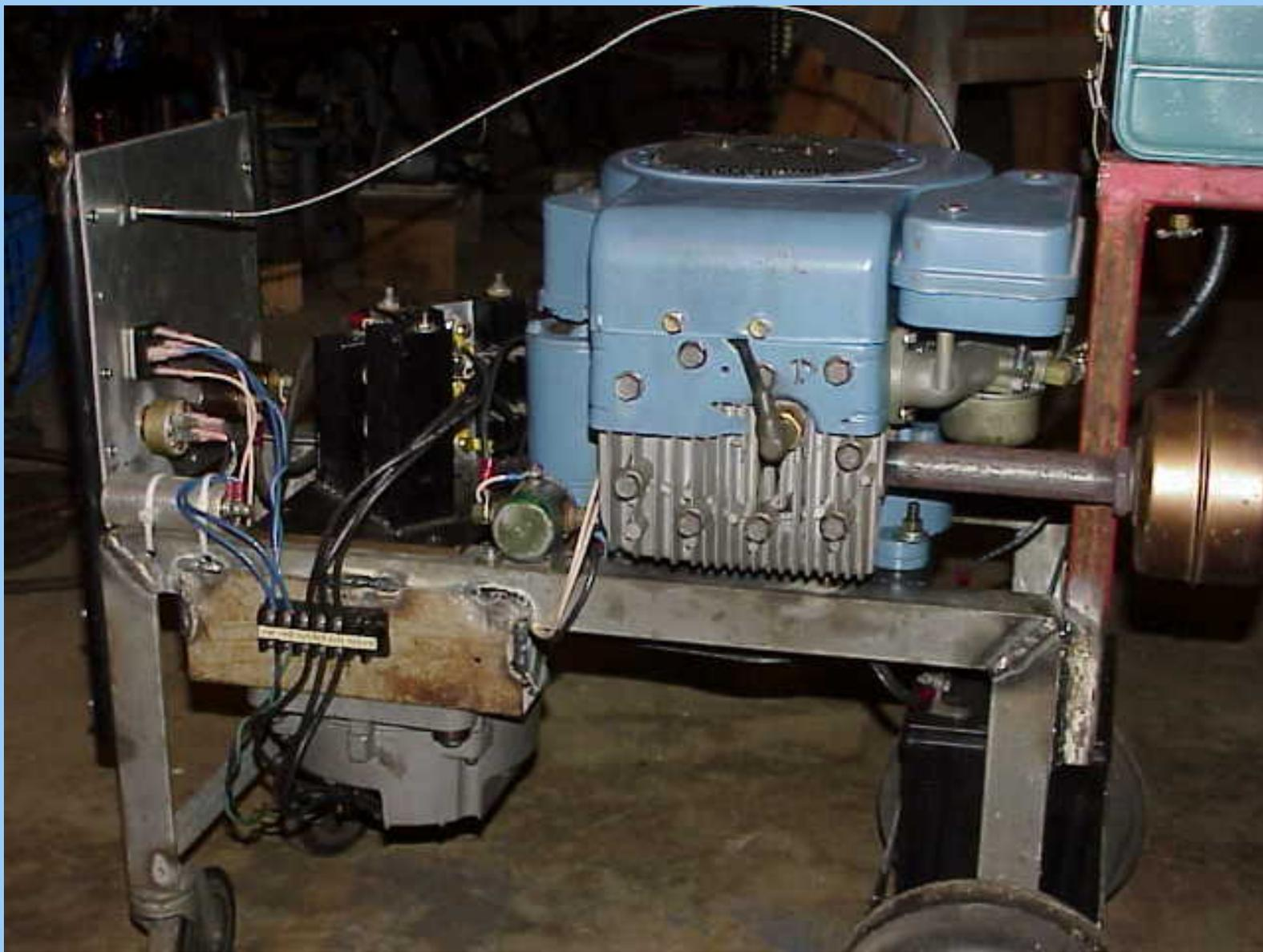
**The terminal block above the alternator has, from left to right: Field power, negative and positive, then the three wires from the three phases from the alternator.**
