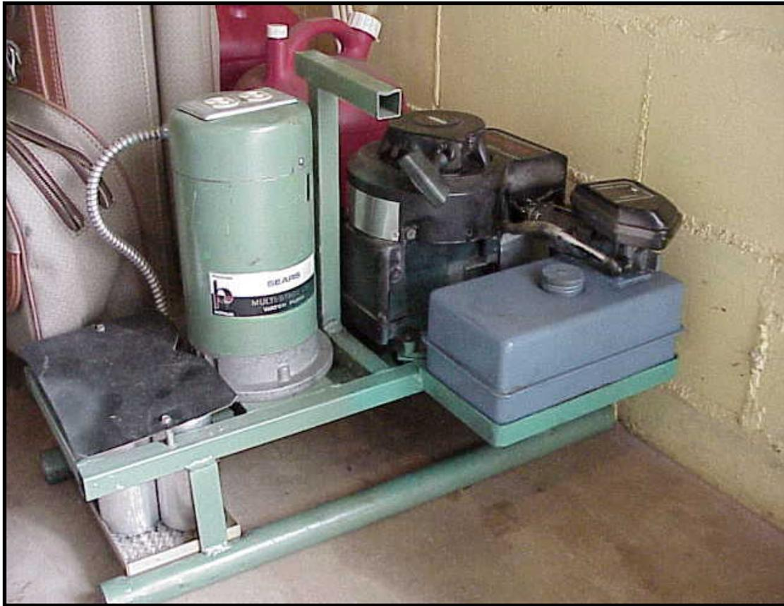
**Note the enlarged gasoline tank. I made this modification in mid June of 1999. This generator was used at the [NC8V field day](#) event and performed perfectly where it ran approximately 12 hours. This one gallon tank allows the generator to run for 4 and 1/2 hours without refueling.**
