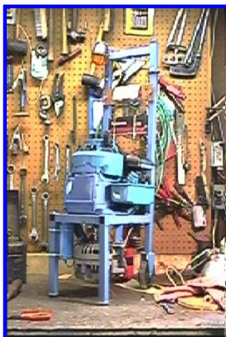
B&S/Chrysler Alternator 12 VDC @ 50 A
