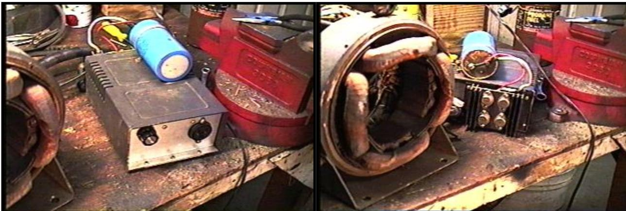
I have 4 pass transistors on the back of it heatsinked. The regulator has to power the 4 poles as electromagnets so it passes a lot of current. I think it is about 6 to 8 amps.
