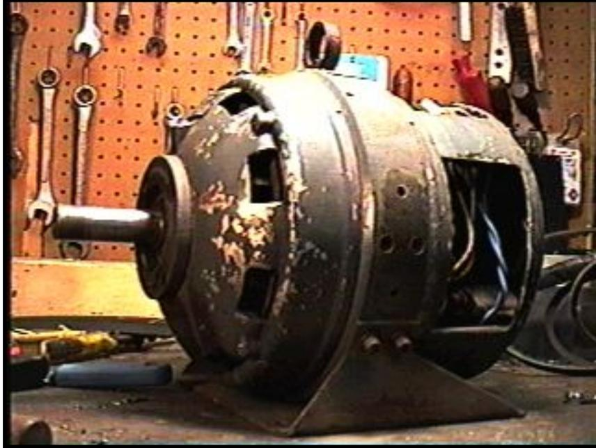
In this generator's original configuration, it was driven by a 3 horsepower, single phase, 124/240VAC 60 hz, electric motor. The outputs were 12 VDC at 25 amps and 120 VAC, 400hz, at 10 amperes. The motor and generator were mounted on a steel frame and weighed in at about 150 pounds. Definitely Navy surplus, as one of the grease fittings called for Navy type grease.
