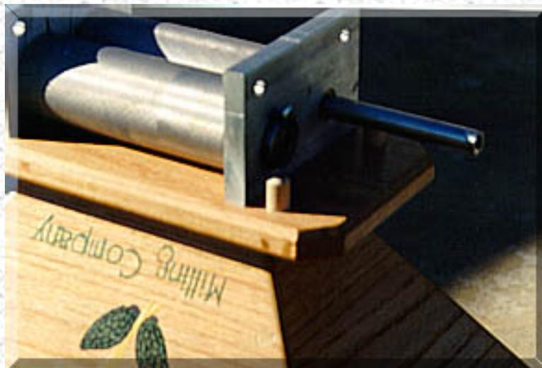
**The malt passing through the rollers transmits motion to the dead roller, eliminating the need for gears or a rubber friction ring. A medium diamond knurl surface was applied to each roller to insure good husk integrity. This, I am told, is possible with 2" diameter rollers.**
