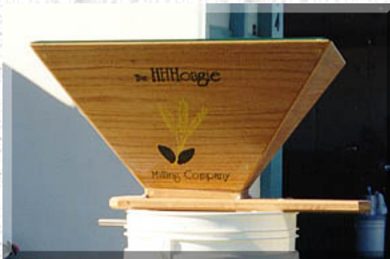
**The HHHoagie Milling Company grain mill is a simple, sturdy self drafting, fully adjustable mill of the two-roller design. It is constructed with 2" diameter rollers, (one live and one dead roller), to provide a low enough nip angle (the angle from the center of the roller axle to the point where the grain contacts the roller surface) to ensure malt will be drawn into the rollers.**
