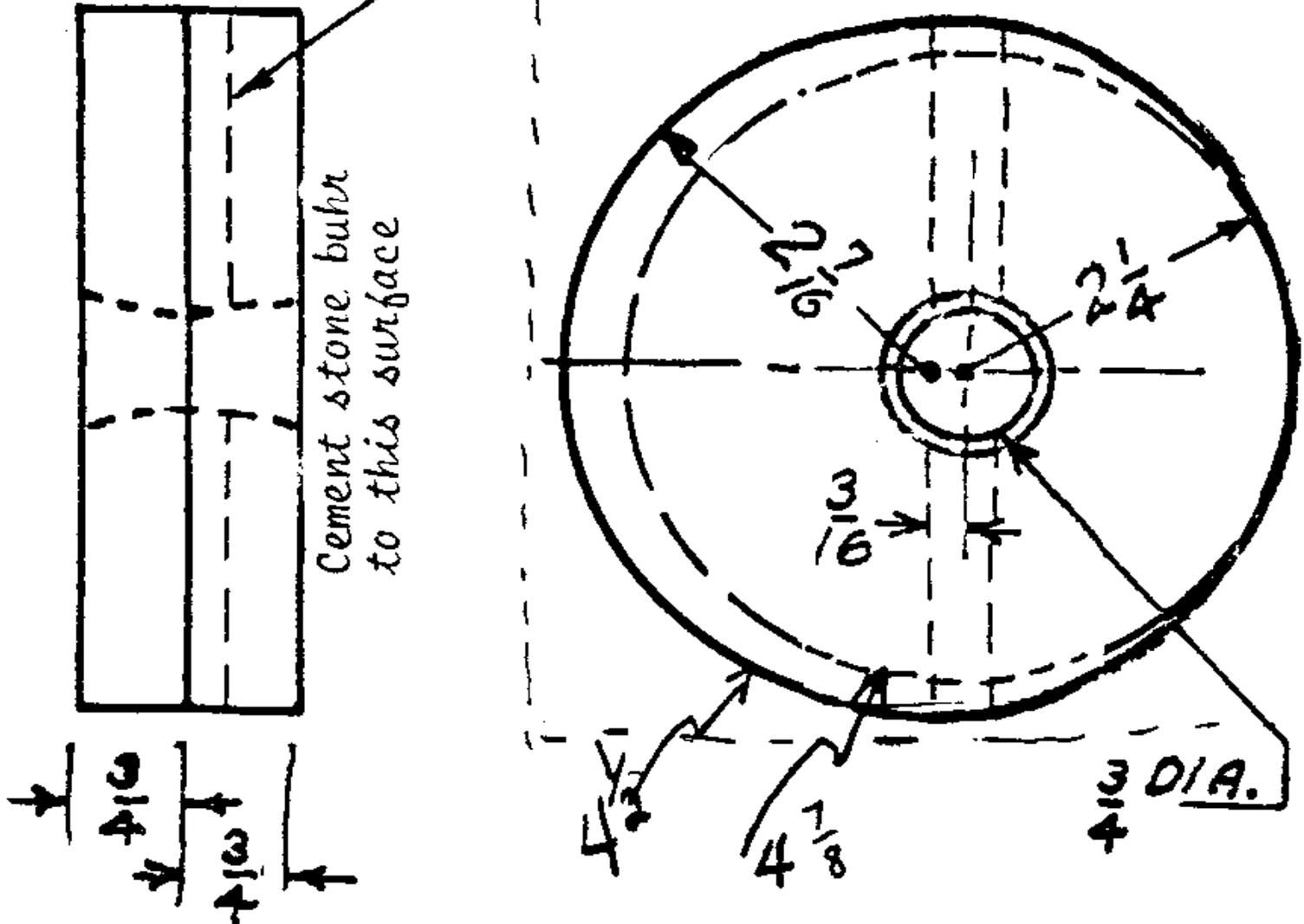
Use two pieces each  $\frac{3}{4}$ " thickness plywood by 5" x 5". Before cutting the pieces round cut the  $\frac{5}{16}$ " by  $\frac{5}{16}$ " slot in one of the pieces as shown. Fasten the two pieces together using about four screws and glue. The  $\frac{3}{4}$  diameter hole should next be located. This hole should pass exactly thru the center of the  $\frac{5}{16}$  x  $\frac{5}{16}$ " slot. Before boring
