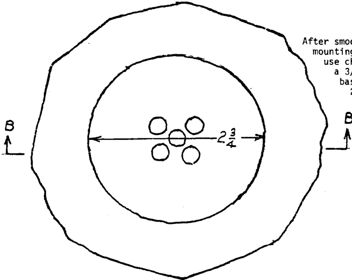
After smoothing and mounting the buhrs, use chisel to form a  $\frac{3}{16}$ " deep basin which is  $2 \frac{3}{4}$ " diameter.
