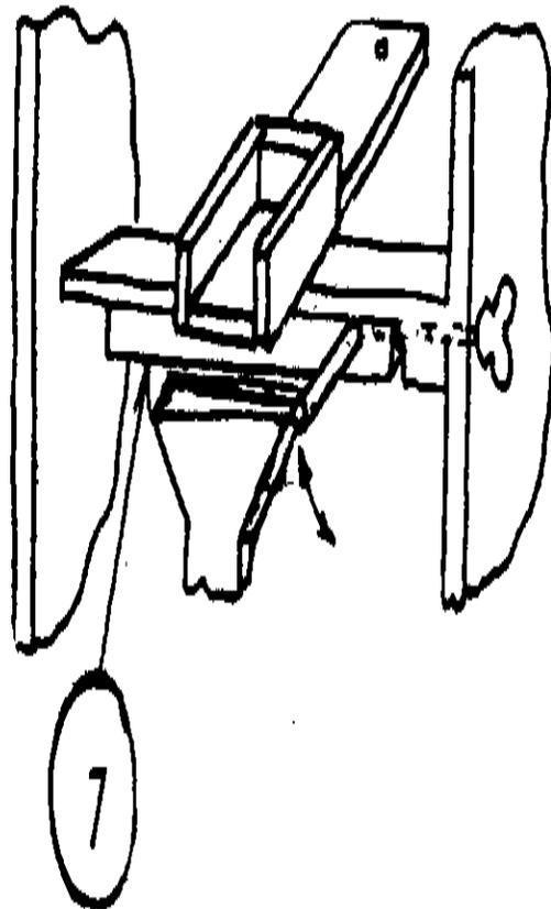
Stove bolt is  $\frac{3}{16}$ " by 2". The winged nut is turned hard against the head of the bolt with epoxy against the head and in the threads. This makes a solid unit of the bolt and winged nut.
