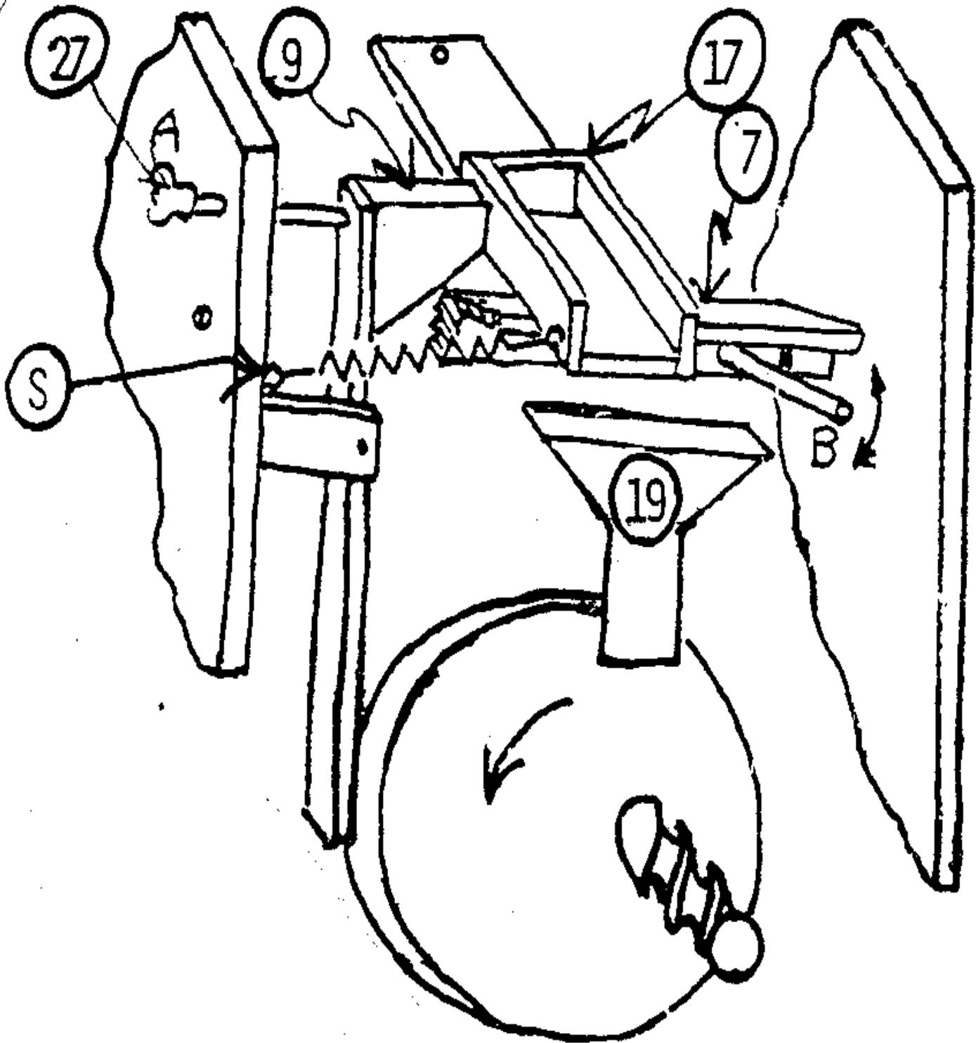
dribbler trough against the Rocker Bar. It is attached at one end to the dribbler as shown and the other end is attached to the inside wall of the mill. The end attached to the mill wall should be about 1/2" lower than the end attached to the dribbler.
