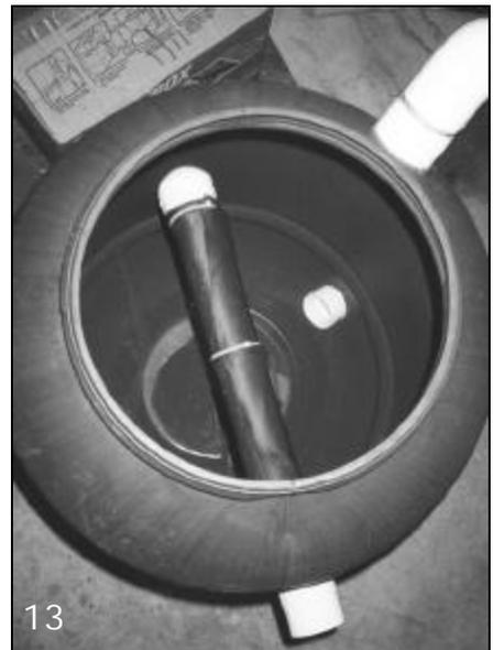
holes boosted the filter-to-intake ratio to 4:1 and I felt better.
