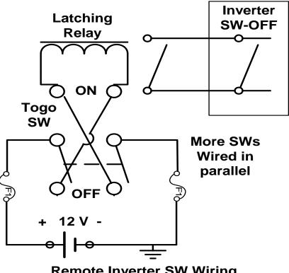
**Remote Inverter SW Wiring**
