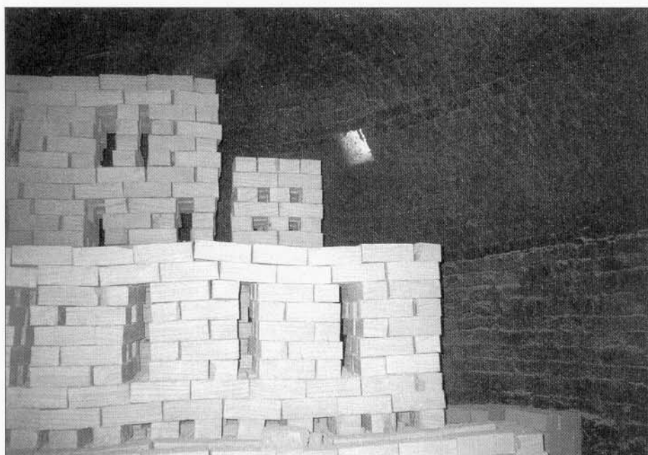
Figure 6 Pillar setting (packing) inside an igloo kiln
