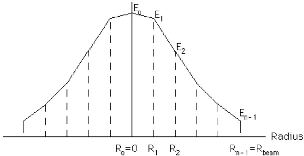
Beam radius is divided into n equal part (radiuses and illumination reading values are indexed from 0, at the beam center, to n-1, at the beam edge).
