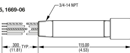
This ‘double ended’ type is used when the field instrument has only a single conduit entry port; the protector attaches to the instrument, and the connection to the field wiring is made inside an external, appropriately rated box connected to the other end of the protector.
