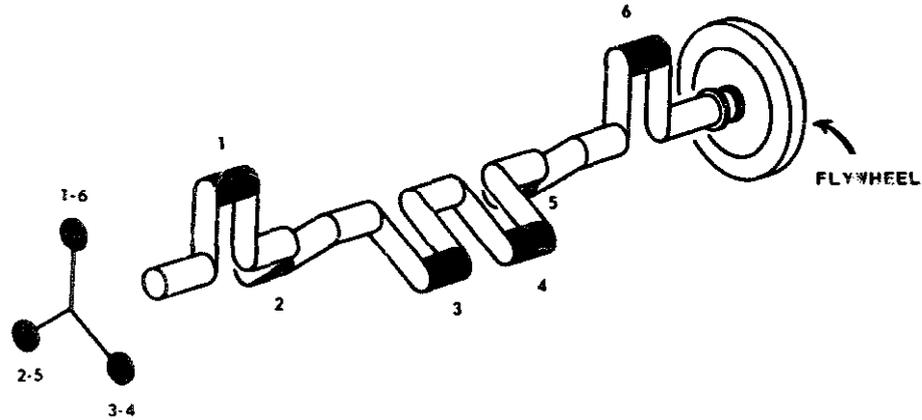
Figure 13-6.—Crankshaft for a six-cylinder engine.
