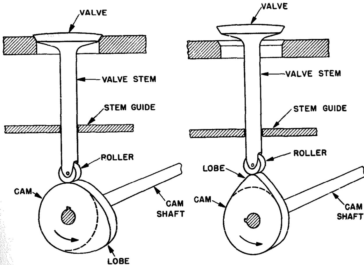
Figure 6-12.—Cam-driven valve.
