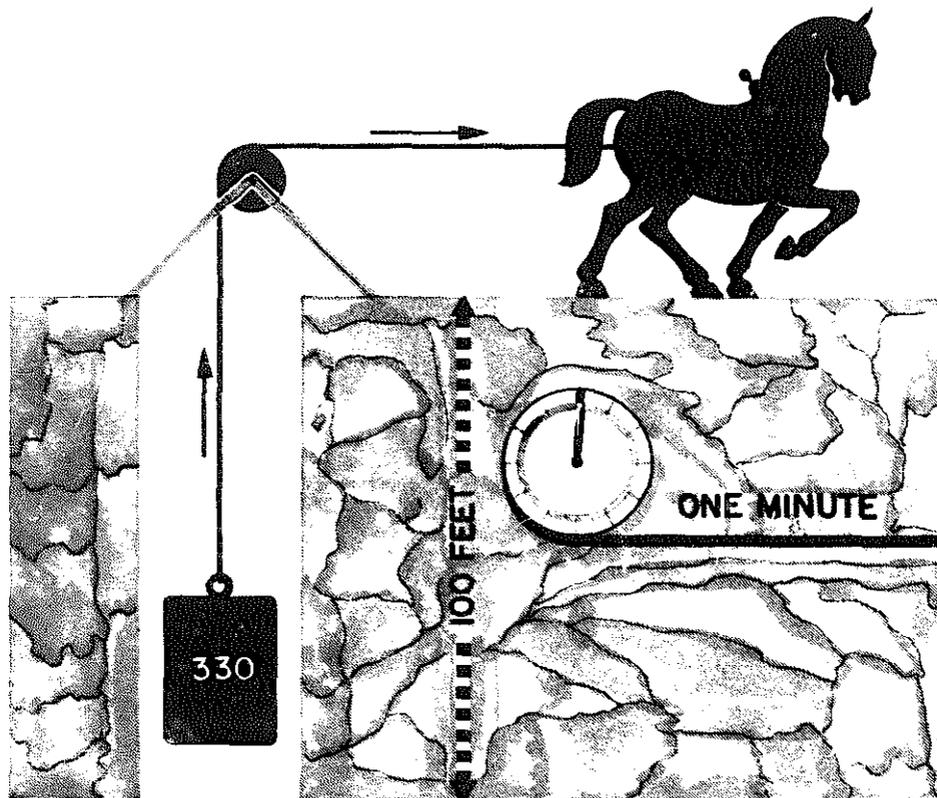
Figure 8-2.—One horsepower.
