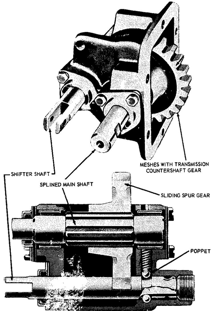
Figure 14-15.--Single speed, single gear, power takeoff.
