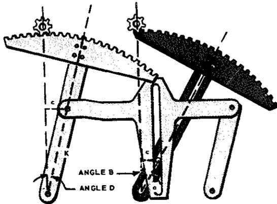
Figure 15-9.— Multiplying with the sector type multiplier. 12.96
