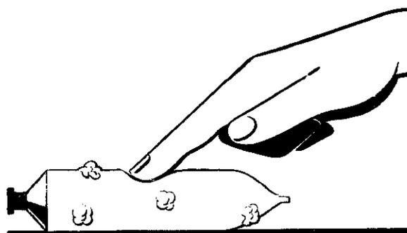
Figure 10-5.—Pressure is transmitted in all directions.
