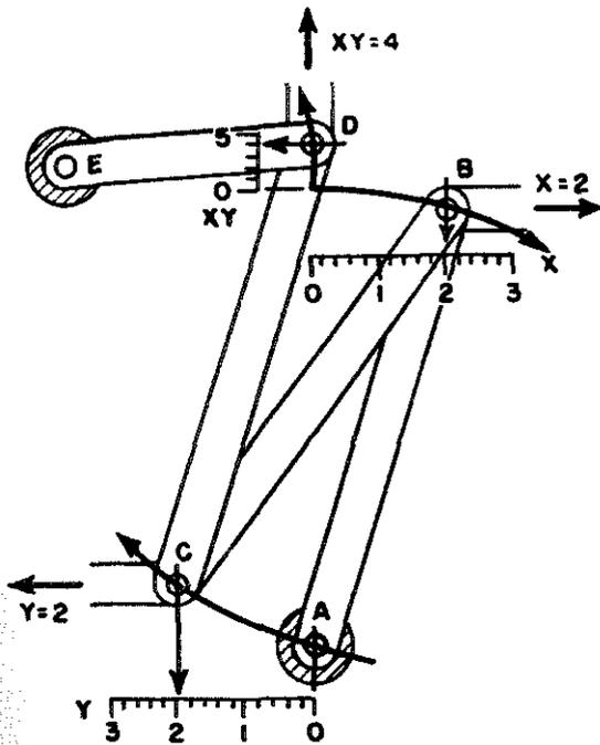
Figure 15-12.—Multiplying linkage. 12.99
