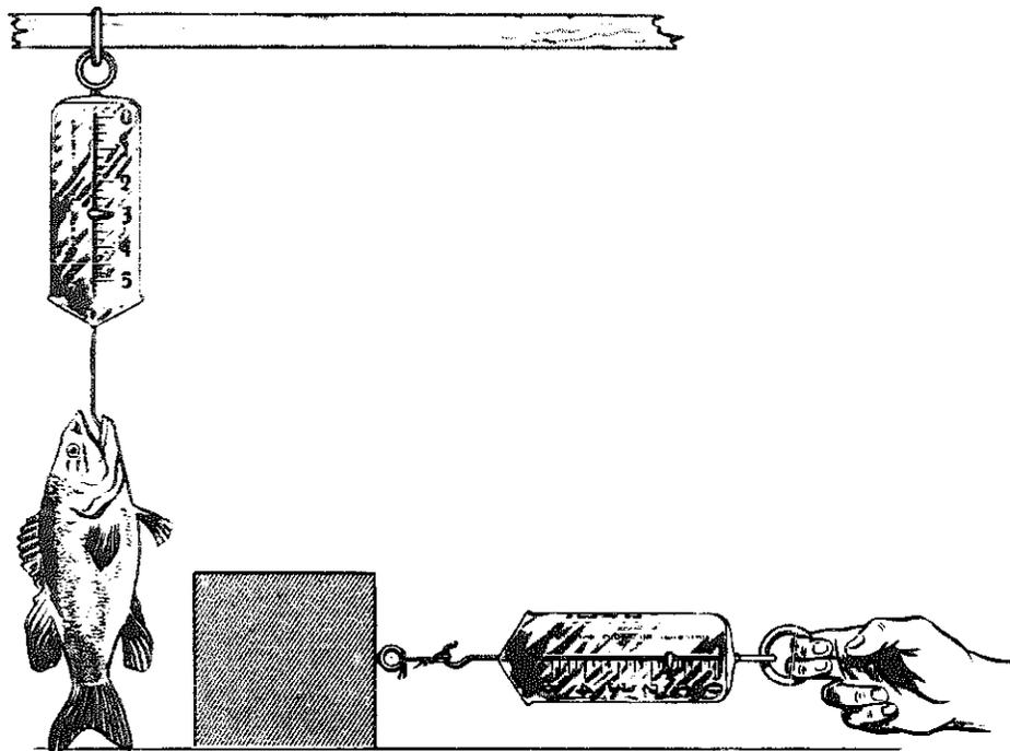
Figure 9-1.—You can measure force with a scale.
