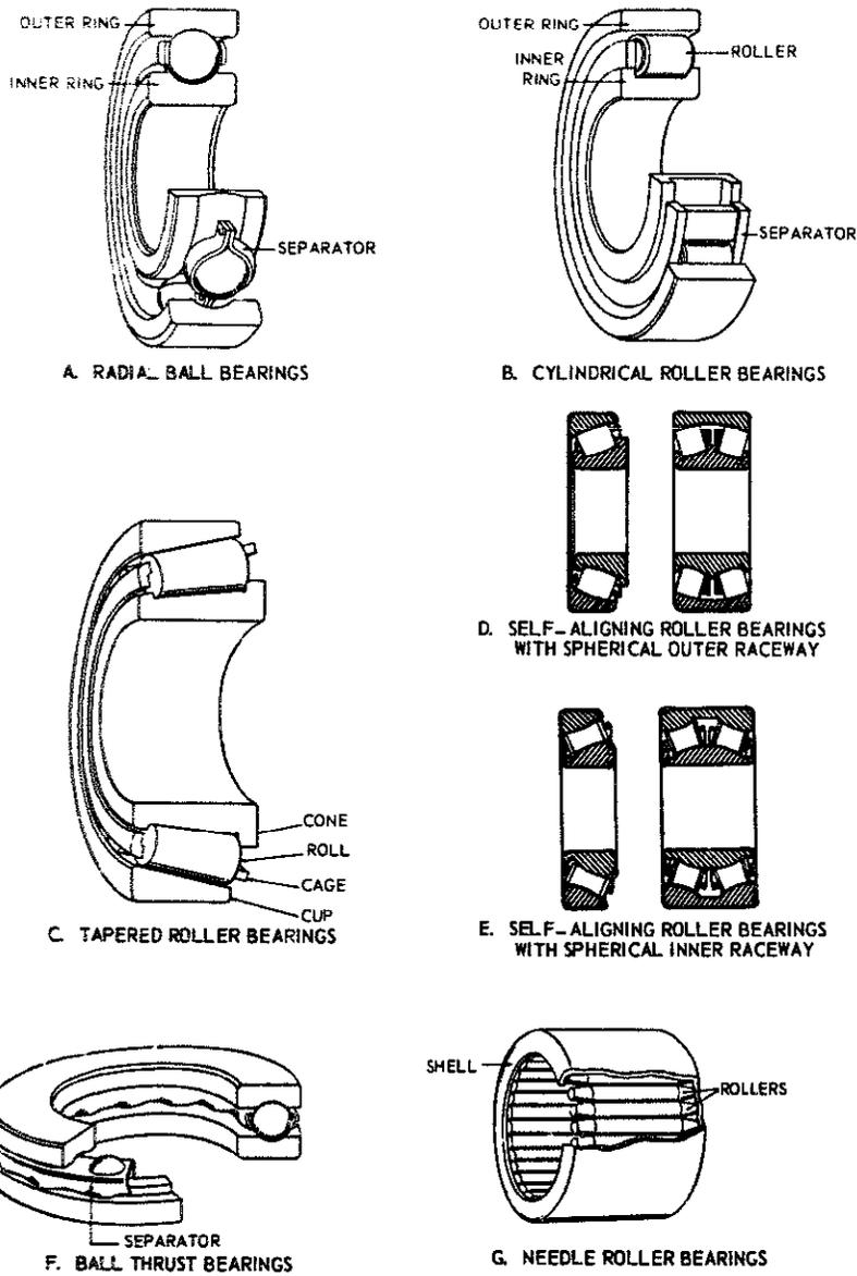
Figure 11-4.—The seven basic types of antifrictional bearings.
