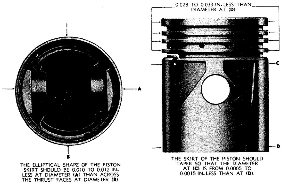
Figure 13-16.—Cam-ground piston.
