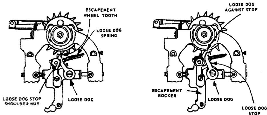
Figure 12-5.—Escapement mechanism.
