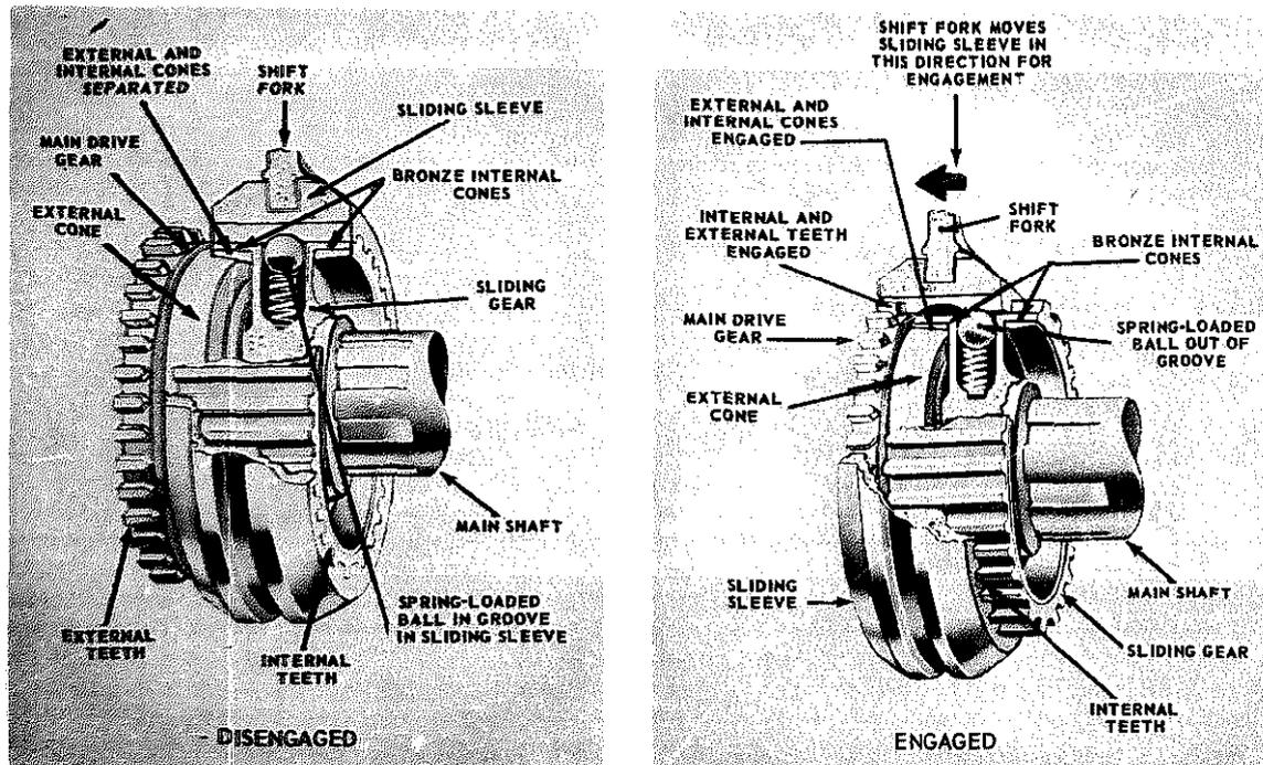
Figure 14-9.—Synchronesh clutch—disengaged and engaged.
