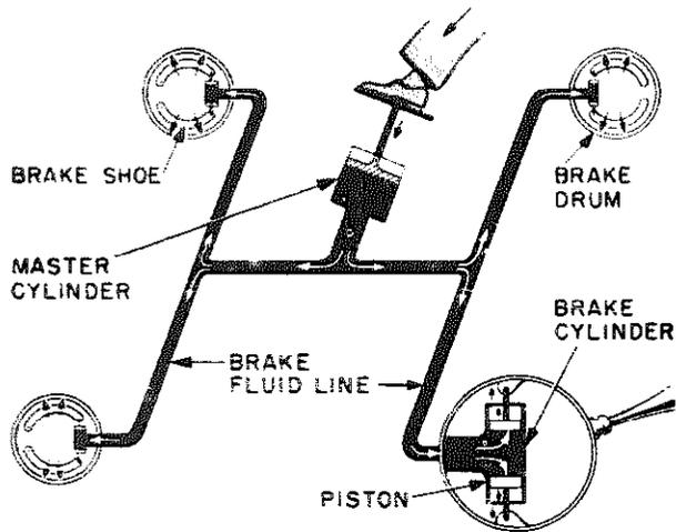
Figure 10-6.—Hydraulic brakes.
