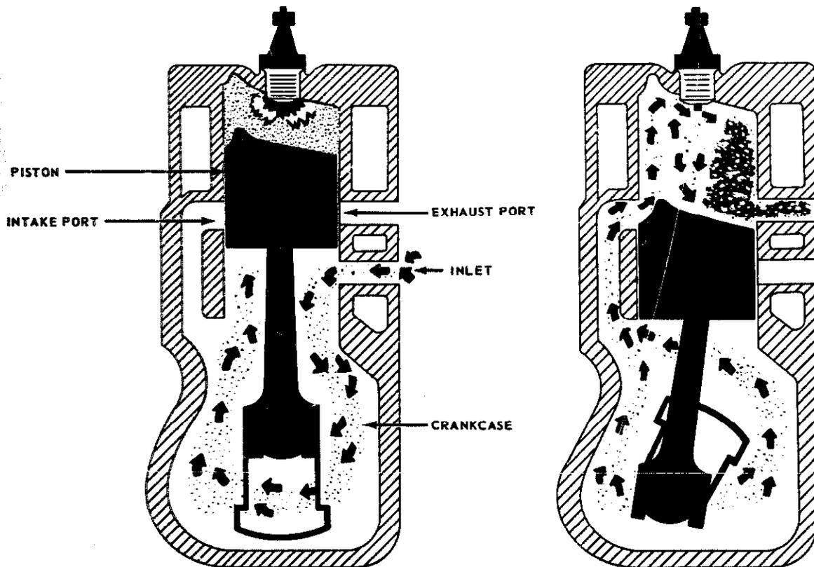
Figure 13-5.—Events in a two-cycle, internal combustion engine.
