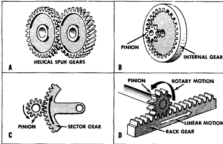
Figure 6-3.—Gear types.
