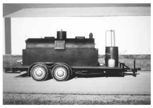
Above: The new metal tank methane digester on its trailer. Photo by Al Rutan
