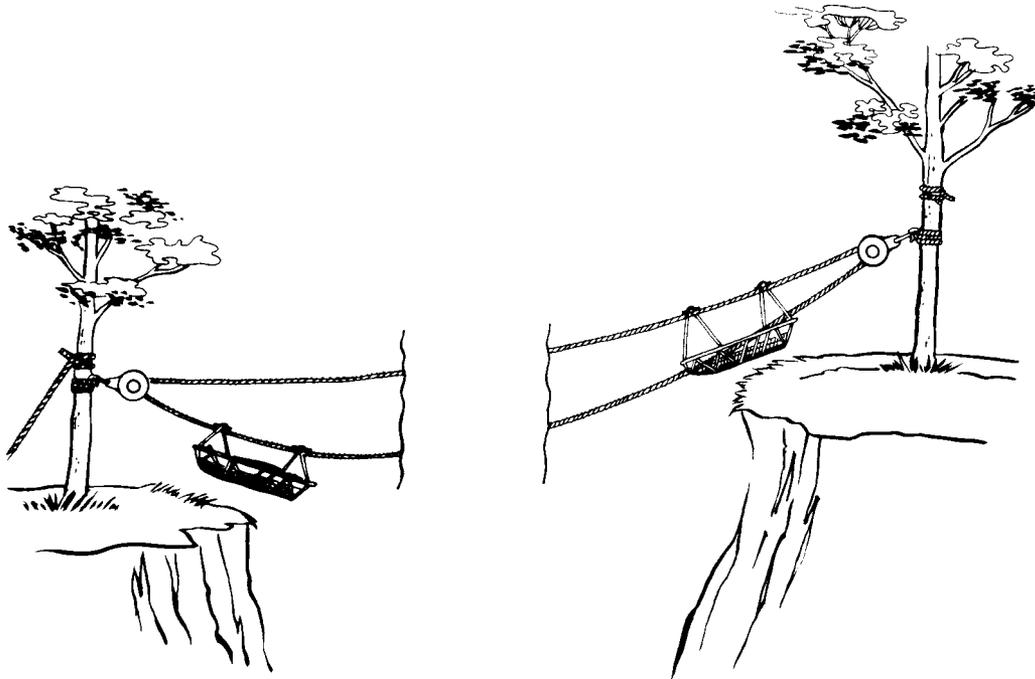
Figure 9-29. Evacuation by horizontal hauling line.
