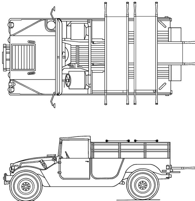
*Figure 10-15. Truck, cargo/troop carrier 1<sup>1</sup>/<sub>4</sub> ton, 4x4, M998 (four-man configuration), with three litters.*
