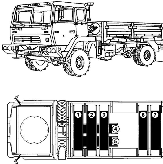
*Figure 10-21b. Loading the truck, cargo, LMTV, LVAD/AD, 2<sup>1</sup>/<sub>2</sub> ton, M-1081.*
