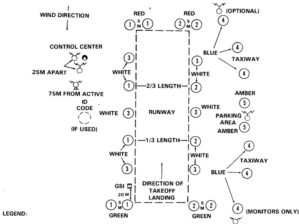
Figure 10-40. Marking and lighting of airplane LZ (night).
