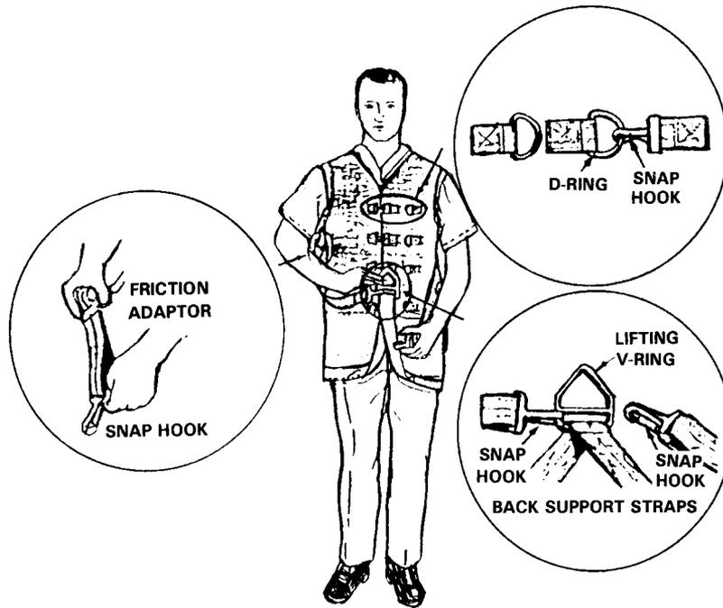
Figure E-12. Hoisting vest donning procedures
