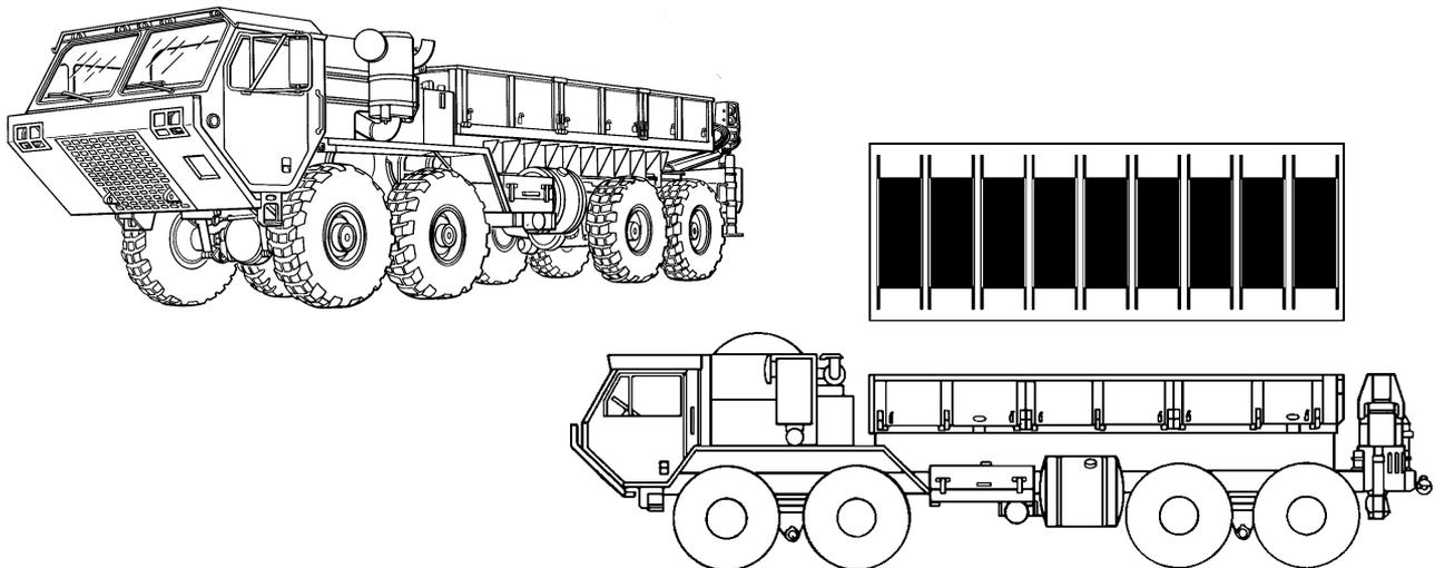
Figure 10-18. Heavy expanded, mobility tactical truck, 8x8, cargo, M977.
