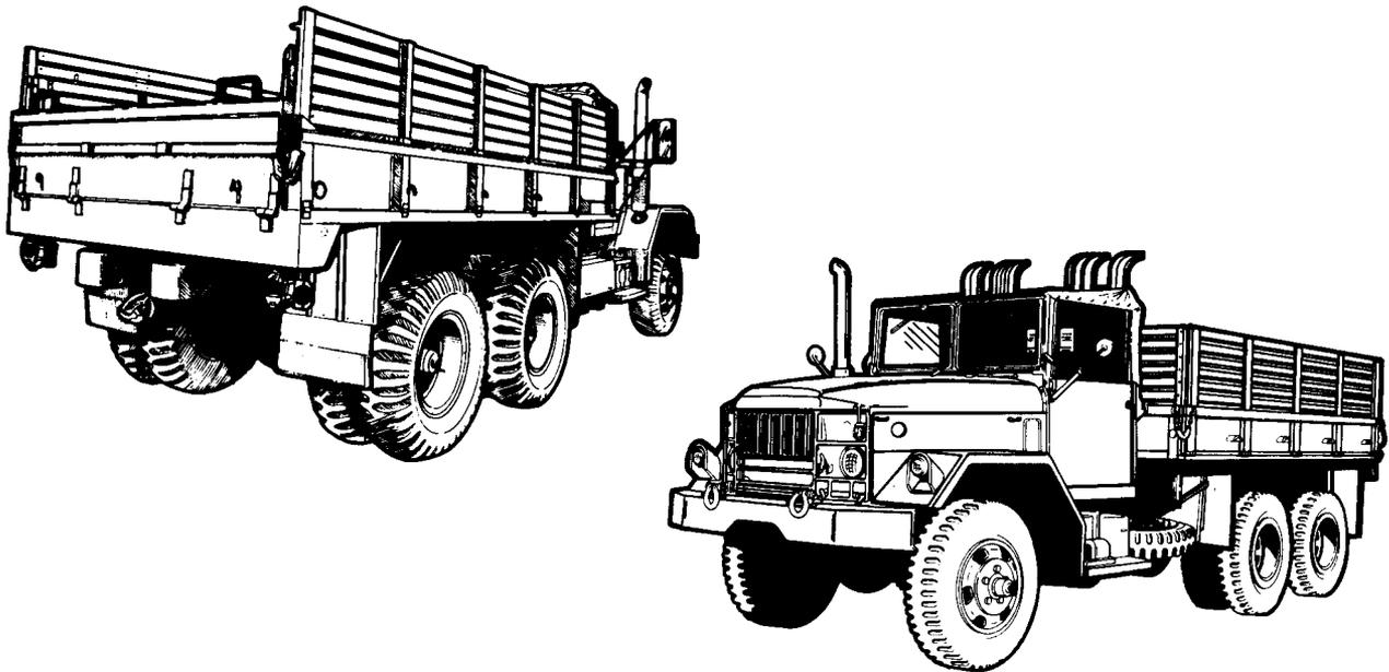
*Figure 10-17. Truck, cargo, 5 ton, 6x6, wide bed, and truck, cargo, 2½ ton, 6x6, wide bed.*
