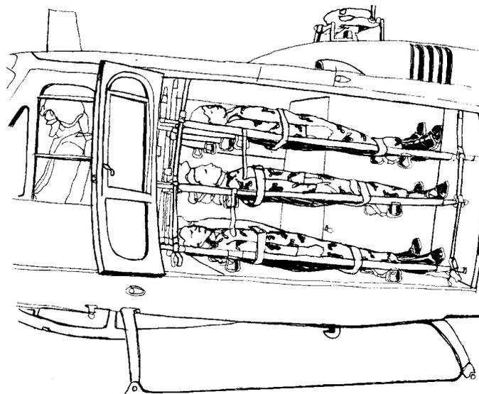
Figure 10-32. Interior view of UH-1H/V Iroquois six-litter configuration.
