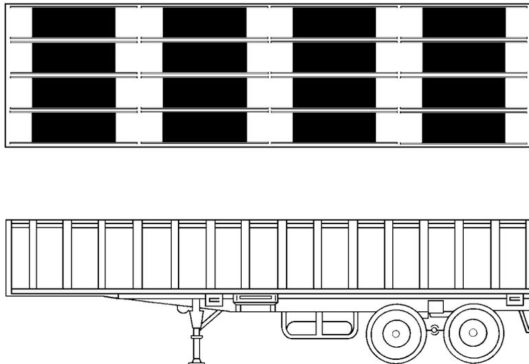
Figure 10-19. Semitrailer, cargo, 22<sup>1</sup>/<sub>2</sub> ton, M871, loaded with litter.
