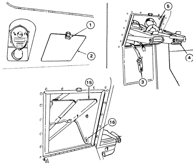
Figure 10-7. Litter rail extension stowage compartment, M997.
