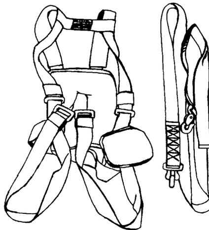
Figure E-1. Vest, hoist operator, and lifeline.
