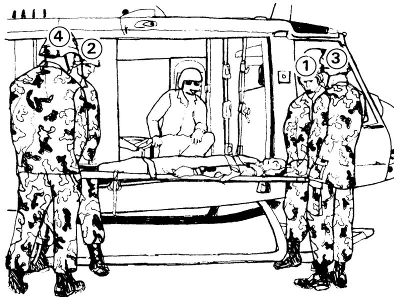
Figure 10-34. Loading air ambulance (UH-1H/V) from right side (step two).
