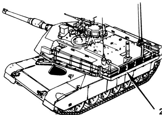
Figure 8-23. The rear of the turret in position.
