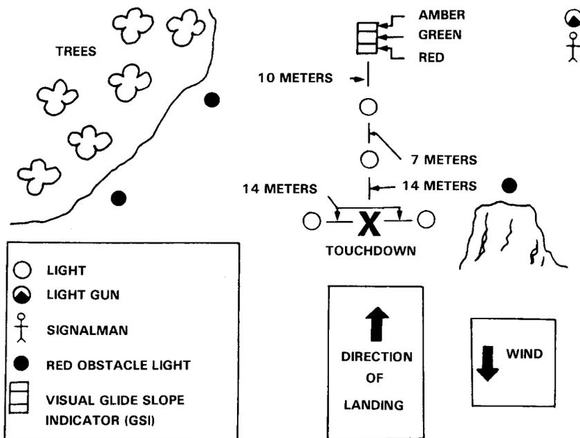
Figure 10-28. Field expedient inverted landing zone (night).
