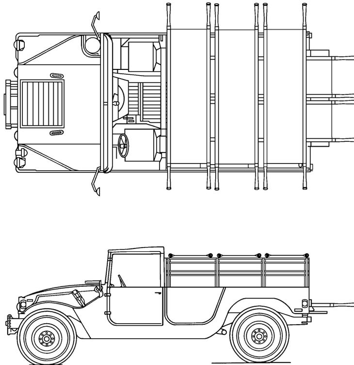
*Figure 10-16. Truck, cargo/troop carrier, 1<sup>1</sup>/<sub>4</sub> ton, 4x4, M998 (two-man configuration), with five litters.*
