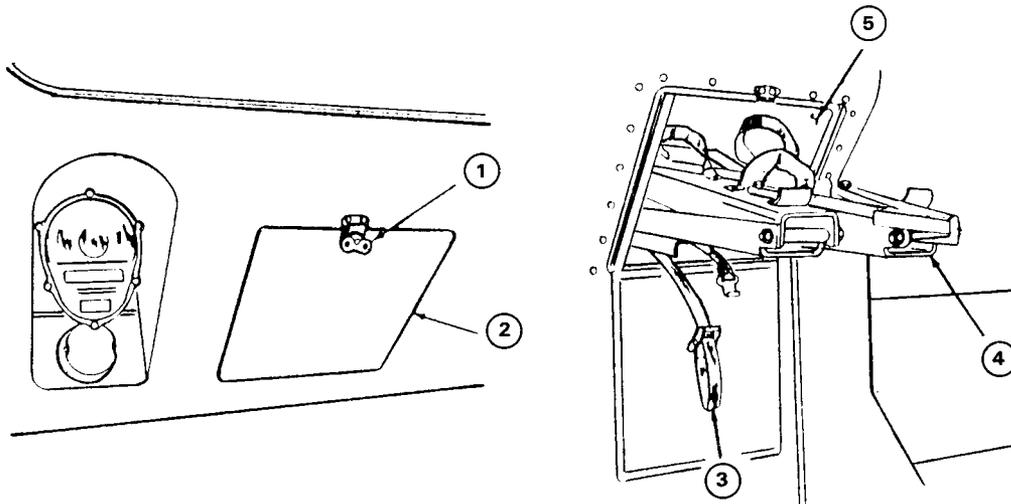
Figure 10-2. Litter rail extension stowage compartment, M996.
