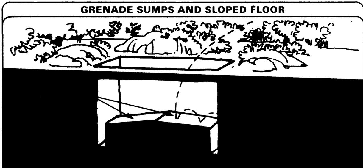
If time permits, an elevated floor stand of saplings can be built so that soldiers do not have to stand in mud or water. Grenade sumps must remain clear.
