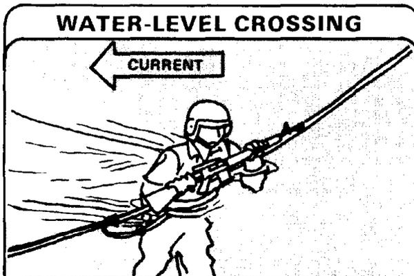
**Crossing Method at Water Level.** Hold onto the rope with both hands, face upstream, and walk into the water. Cross the bridge by sliding and pulling the hands along the rope. (For safety, each soldier ties a sling rope around his waist, leaving a working end of about 3 to 4 feet. He ties a bowline in the working end and attaches a snaplink to the loop. He then hooks the snaplink to the rope bridge.)
