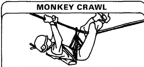
*Monkey crawl.* Hang suspended below the rope, holding the rope with the hands and crossing the knees over the top of the rope. Pull with the hands and push with the legs. (For safety, each soldier ties a rappel seat and hooks the snaplink to the rope bridge.) This is the safest and the best way to cross the one-rope bridge.
