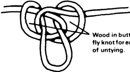
Wood in butterfly knot for ease of untying.
