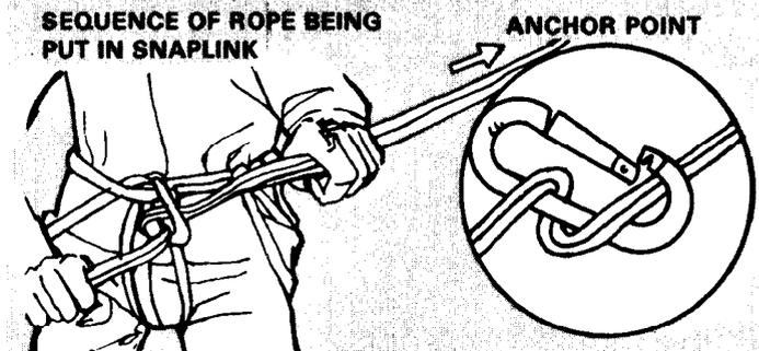
Bring the ends of rope between the legs (front to rear), up and around the legs (rear to front), and under the waist loop.
