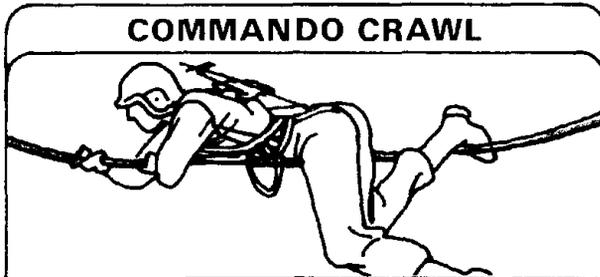
*Commando crawl.* Lie on the top of the rope with the instep of the right foot hooked on the rope. Let the left leg hang to maintain balance. Pull across with the hands and arms, at the same time pushing on the rope with the right foot. (For safety, each soldier ties a rappel seat and hooks the snaplink to the rope bridge.)
