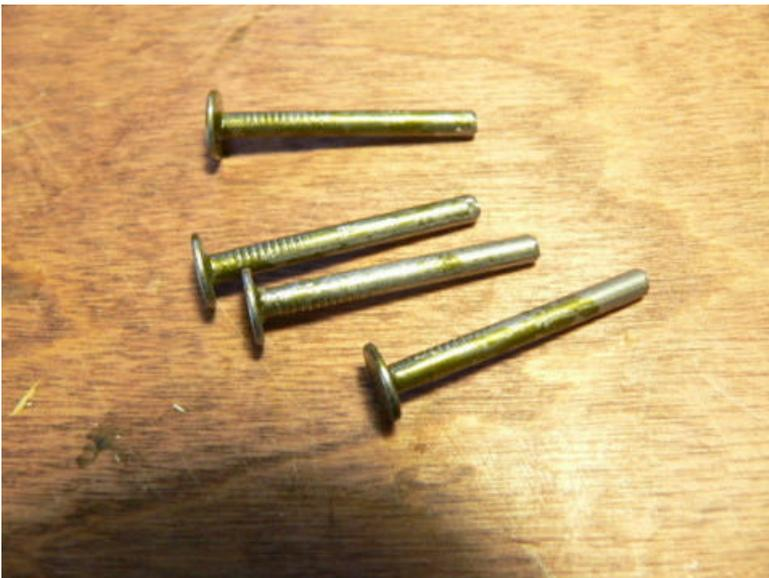
Cut 4 16 penny nails and cut them 1.125" long (including the head). De-burr the ends you've cut (so they're not sharp). Once the coil winder is finished, we'll insert these through the 4 holes in the front (4" diameter) disk and they'll also go into the holes in the rear disk, so that the disks are pinned together and the pins will be supported both in the front and in the back. These 4 pins will form the center of the coil.
