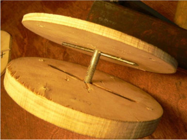
Put the 5/8" thick disk on the shaft so that it fits over the pin that's through the shaft, and bring it tightly against the 1/4" thick disk.
