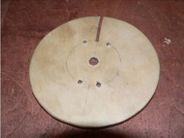
Cut a slot in the front 4" diameter disk as shown. It should be about 1/8" wide and should come right to the center, and stop between the two pins that are nearest each other. We'll start winding the coils from this slot and it needs to be centered at the narrowest part of the coil.
