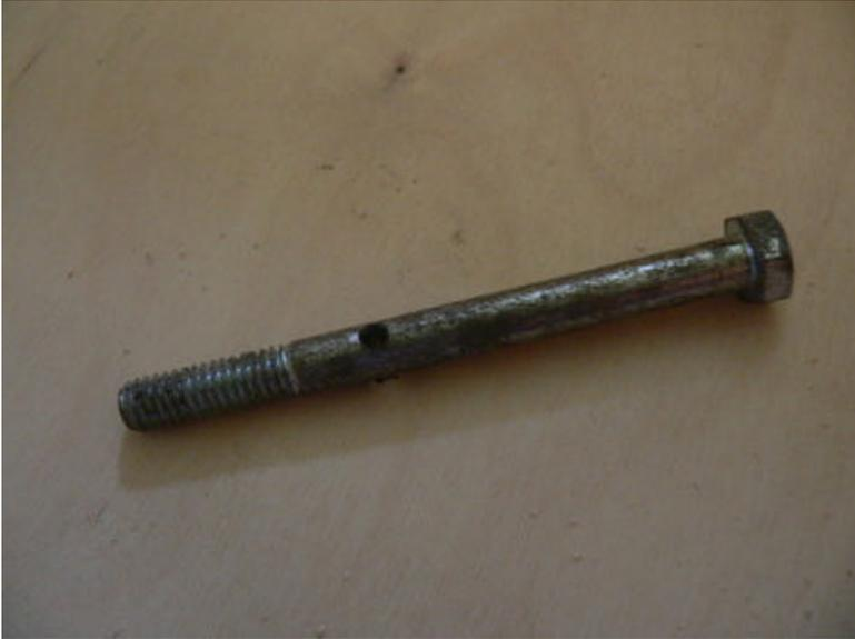
Drill a hole ( $9/64$ " ) through the 3.5" long bolt. The hole should be drilled on center at  $2 \frac{3}{8}$ " from the bottom of the bolts head. The  $9/64$ " hole is a good diameter to fit a 16D nail pretty tightly.
