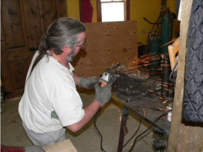
Whenever we cut metal there are sharp burrs at the cut. It's nice to cleanup all our cuts (and welds) with a grinder. Pictured above George is grinding the cuts (he should be wearing a face mask).
