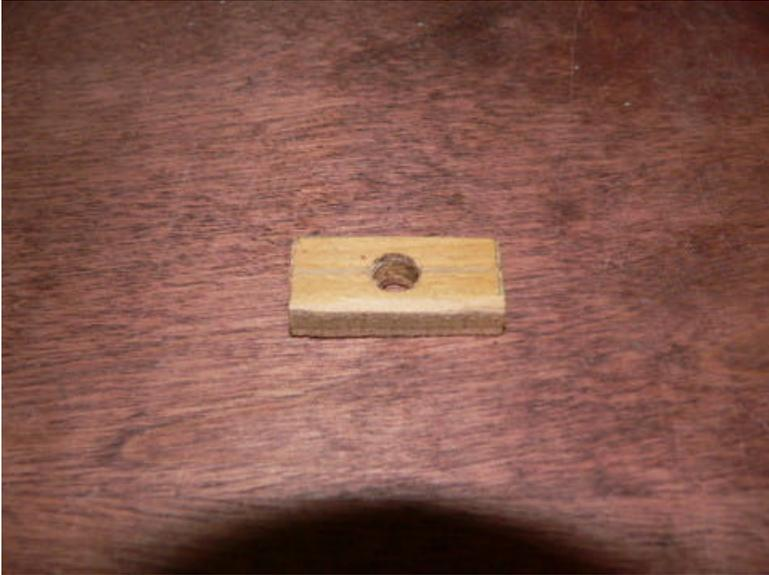
Cut a piece of  $3/8$ " plywood rectangular as shown above. It's 1.5" tall, and  $3/4$ " wide. Drill a  $5/16$ " hole through the center. This serves as a spacer between the disks.
