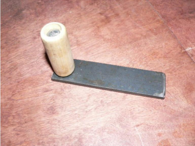
Put the shorter bolt (2.5" long) through the wooden handle and thread it into the 5" long bar stock which has been drilled and tapped to accept the bolt. Put a washer in between the handle and the bar stock. Thread the bolt in so that the threads come flush with the back of the bar stock, and the handle should turn freely .
