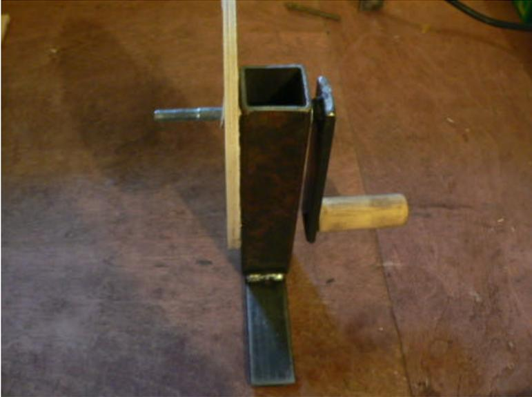
Put another washer on and then put the 6" diameter 1/4" thick disk on. The countersunk holes need to be pointing back, towards the handle.
