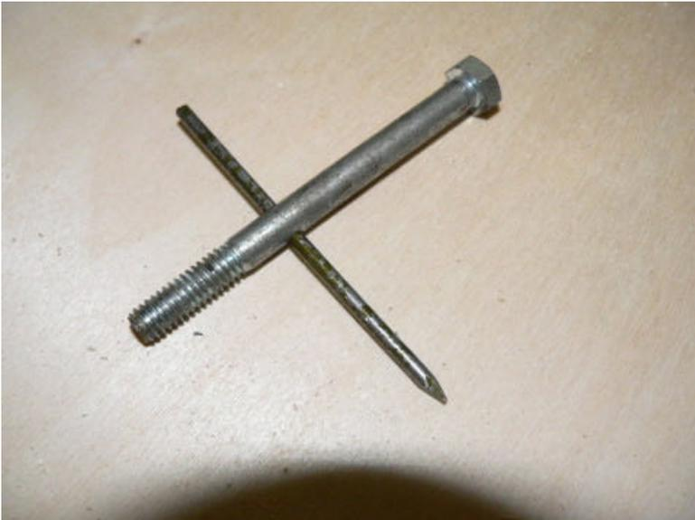
The nail serves as a pin to lock the spool to the shaft (the bolt is the shaft)
