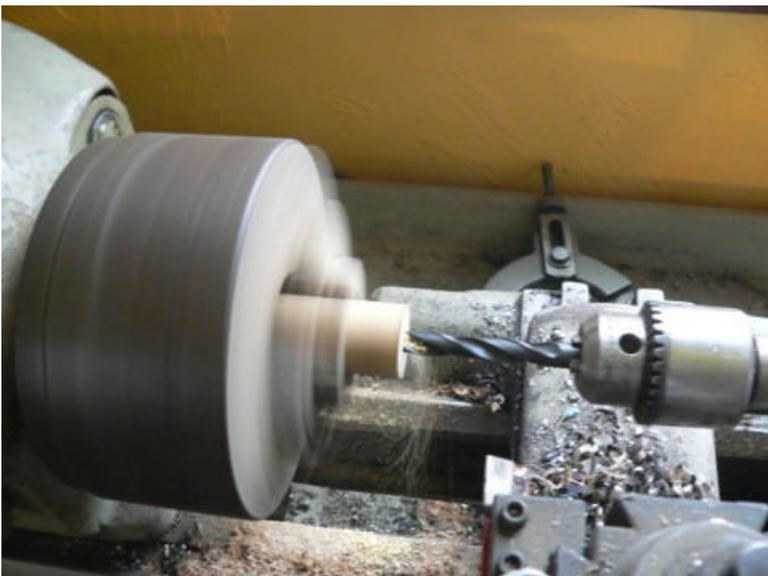
We cut the dowel off with any saw, and then drill it out on the lathe. While it's on the lathe it's nice to round the edges and sand it a bit. If you don't have a lathe, you could do this carefully with a hand drill or drill press, or - if it's just for one machine the wooden handle is not very important, it just makes for more comfortable winding.
