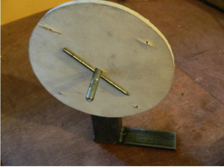
Insert the pin through the shaft and center it.
