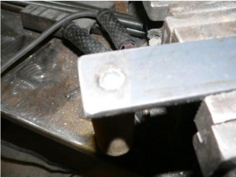
Turn it over and spot weld where the bolt is through the bar stock -this assures that the handle will never come loose.
