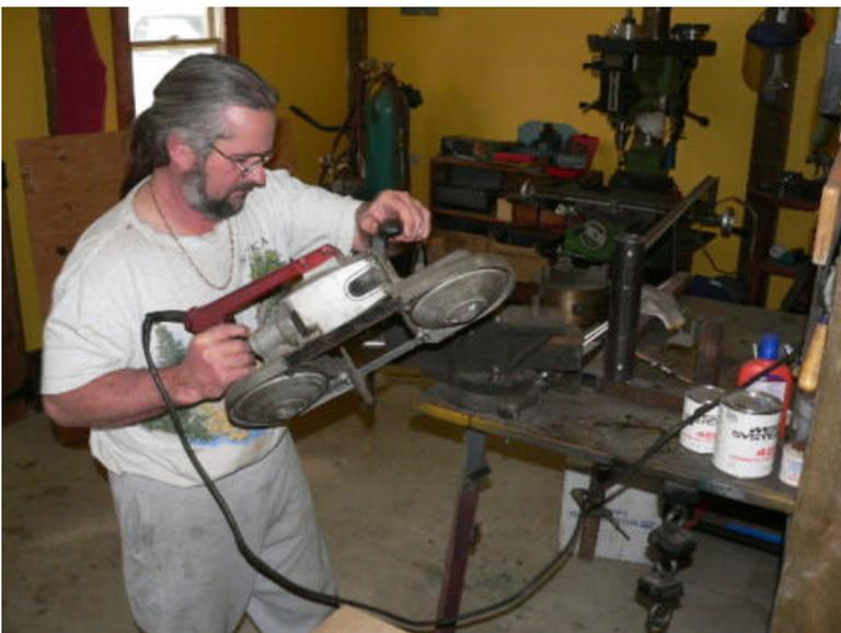
First step is to cut out some metal parts. I find the portable metal cutting band saw fast and easy, but a hack saw, saw zall or even a torch would work fine. In building wind turbines we often have to adapt a design to accommodate the tools and resources that are available to us, sometimes this requires some imagination.
