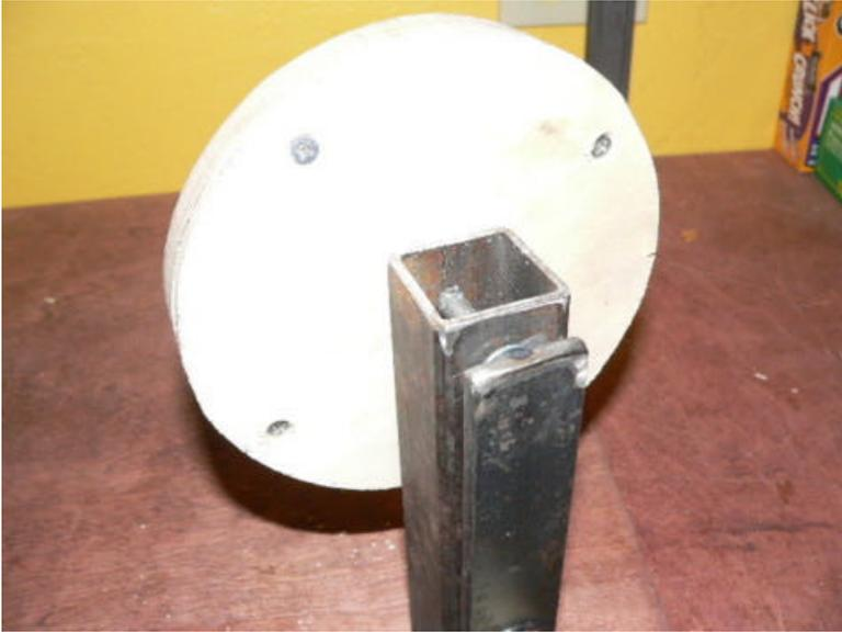
Use 5/8" long wood screws to screw the two disks together coming in through the back of the coil winder, through the 4 holes we drilled and countersunk earlier. The screw heads need to be flush, they must not stick out.
