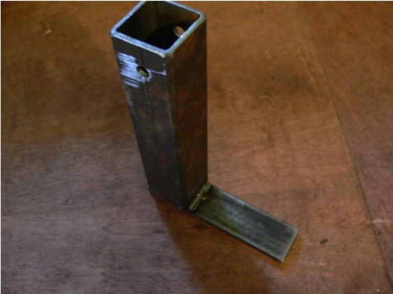
Weld the 5" long bar stock that has no holes in it to the bottom (the end furthest from the hole) of the square tubing. This serves as a base so that we can clamp the coil winder to a workbench.
