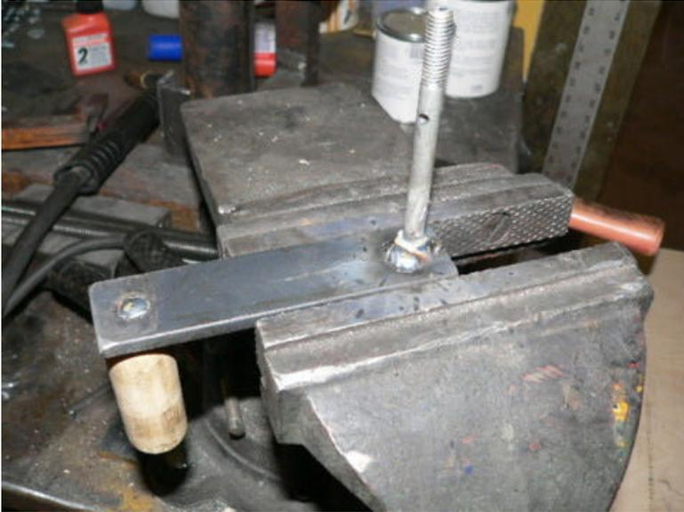
Take the longer bolt (the one with the hole drilled in it) and weld it to the other end of the handle as shown in the picture. It needs to be square!
