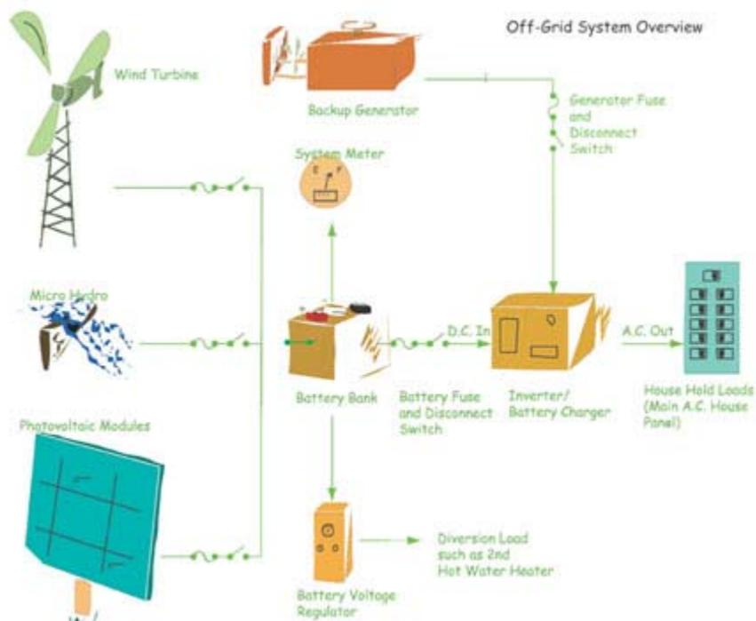
All off-grid systems work much in the same fashion. Collect energy from a renewable source (wind, sun, and/or stream), convert it to electricity and store the energy, usually in a battery bank. When we
