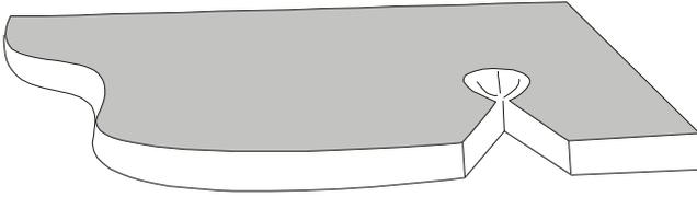
Take your knife, saw, or whatever is best for you, and cut a v-notch in the wood as illustrated. The opening of the v shouldn't be bigger than about a 1/4 of an inch. It is important that the notch—where the v comes to a point—is not too wide. If that happens the spindle will have a tendency to slip into the notch and prevent you from spinning. The point of the v should come to a point about 1/16 of an inch into the depression where the spindle will be working.
