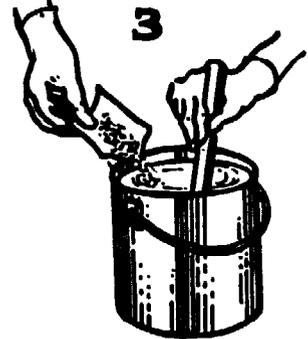
PREPARE SENSITIZING SOLUTION BY DISSOLVING 2 1/2 OZ. OF POTASSIUM BICHROMATE IN 1 GAL. OF LUKE WARM WATER — CHILL TO 60° F. OR UNDER BEFORE USING GOOD FOR TWO WEEKS.
