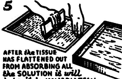
AFTER THE TISSUE HAS FLATTENED OUT FROM ABSORBING ALL THE SOLUTION IT WILL TAKE, IT IS IMMEDIATELY REMOVED FROM THE BATH AND SQUEEGEED GELATIN EMULSION SIDE DOWN UPON THE LACQUERED AND WAXED AND POLISHED POSITIVE WHICH ACTS ALSO AS THE TEMPORARY SUPPORT.
