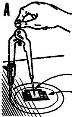
**A** TO PREVENT DAMAGE TO CUTTING FILM AT COMPASS POINT IN CUTTING CIRCLES
