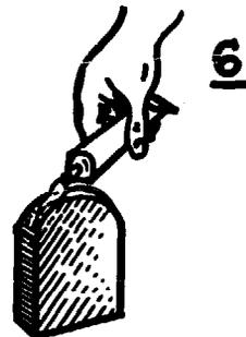
SPREAD EPOXY CEMENT UPON CURVED END OF PLYWOOD HANDLE
