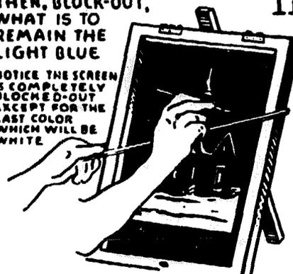
12 AFTER PRINTING THE FINAL COLOR OR WHITE, THE FINISHED PRINT SHOULD BE AN EXACT REPRODUCTION OF THE ORIGINAL MASTER SKETCH
