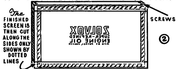
AFTER THE MESH HAS BEEN CUT ALONG SIDES OF THE FRAME AND THE SCREWS REMOVED, THE STENCIL SCREEN WILL LOOK LIKE THIS.
