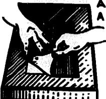
AFTER PRINTING RUN HAS BEEN COMPLETED THE TOP STENCIL SCREEN IS DETACHED, AND BOTH SCREENS CLEANED IN USUAL WAY.
