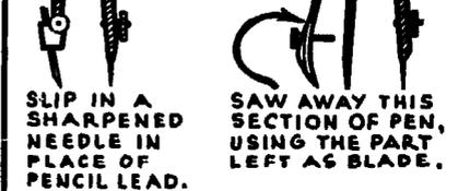
SLIP IN A SHARPENED NEEDLE IN PLACE OF PENCIL LEAD.
