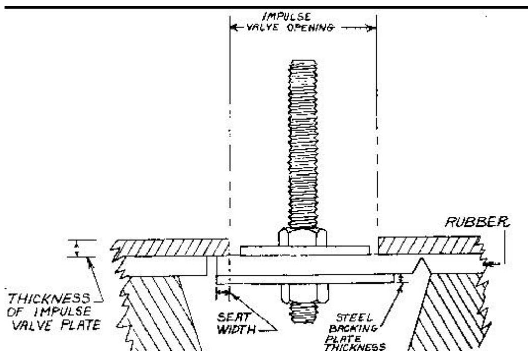
**Thickness of impulse valve plate**
