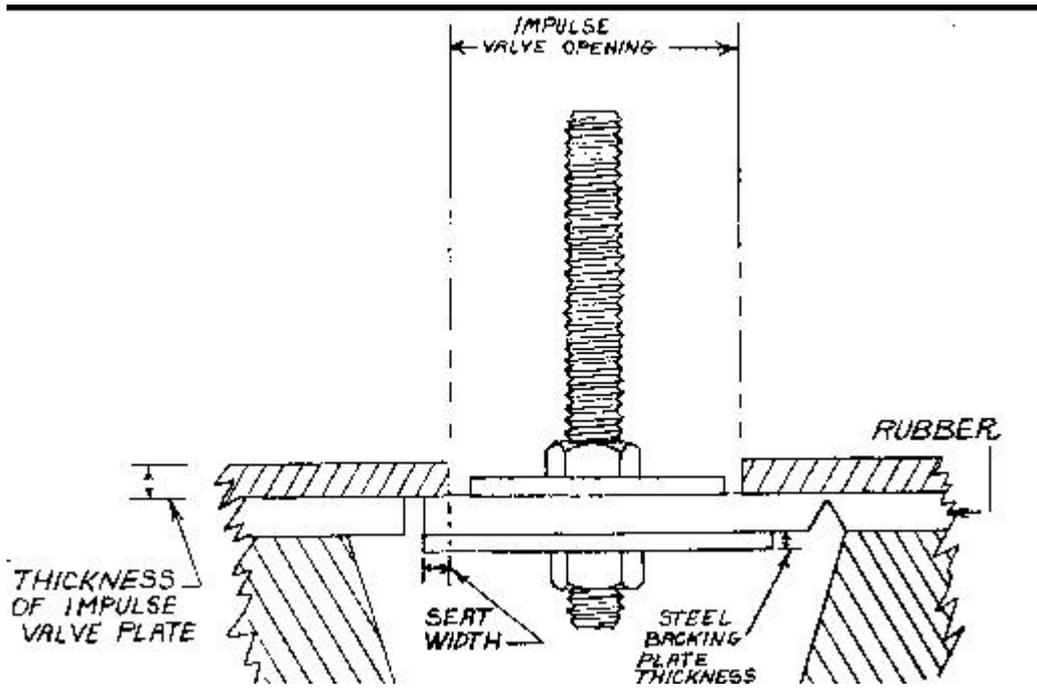
**Impulse valve steel backing**
