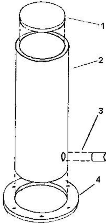
**Welded hydram, accumulator: exploded view**
