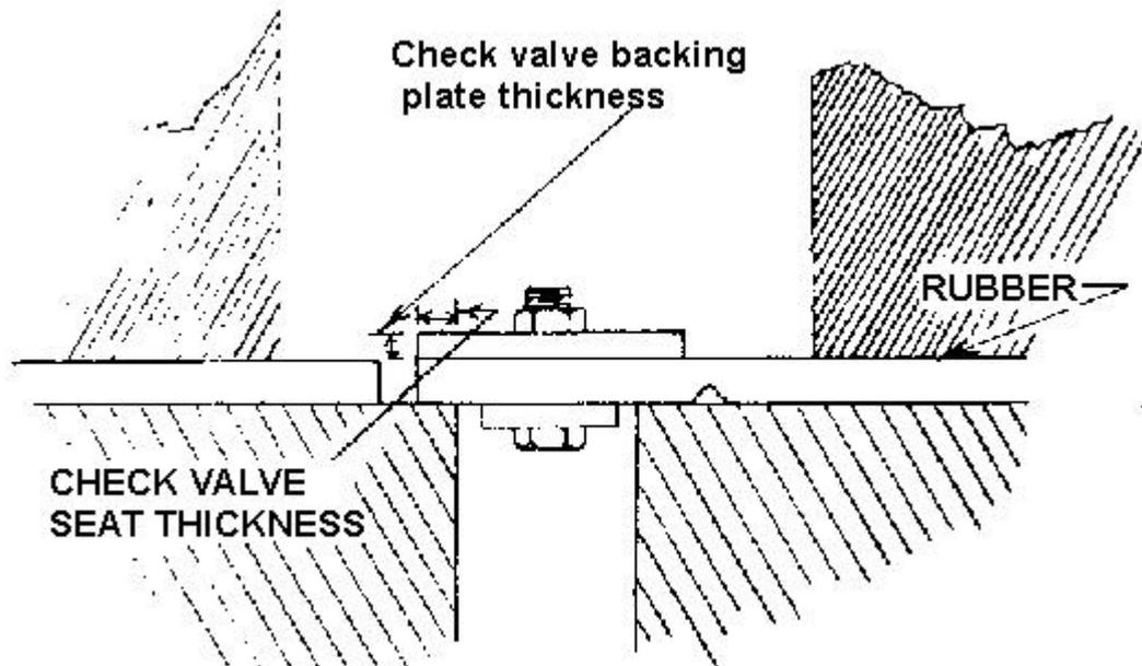
Check valve backing thickness in inches
