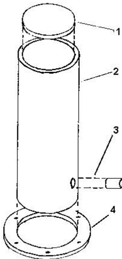
**Welded hydram: accumulator: exploded view**
