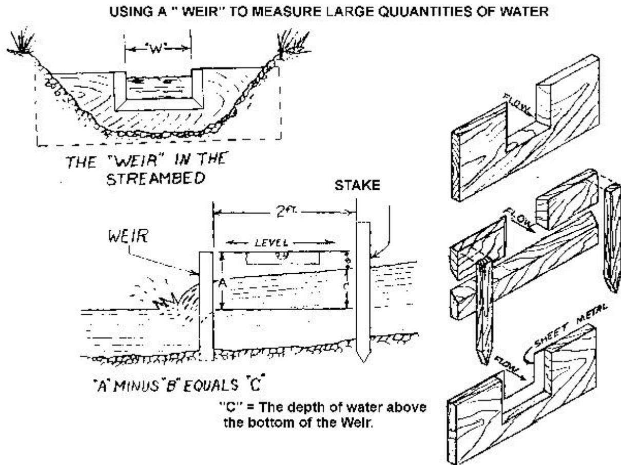
Using a "Weir" to measure large quantities of water
