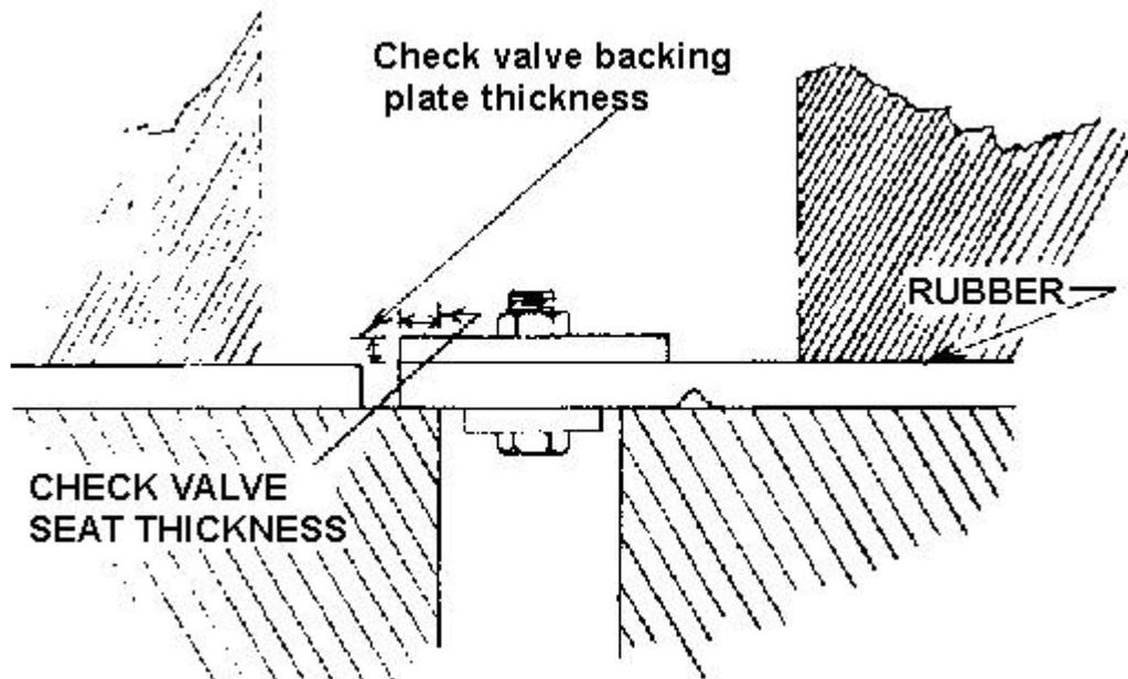
Check valve backing thickness in millimeters
