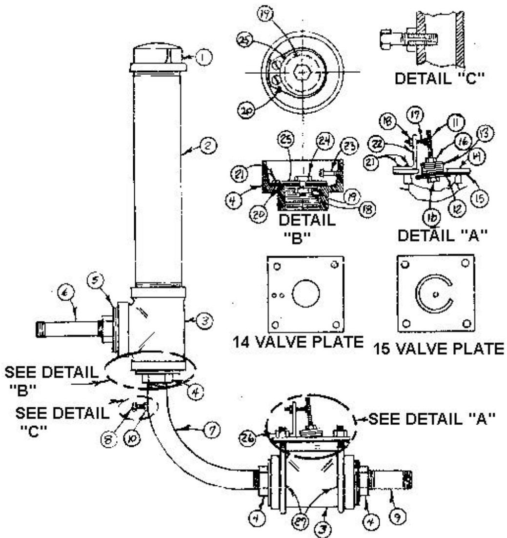
Pipe fitting hydram with field-made valves
