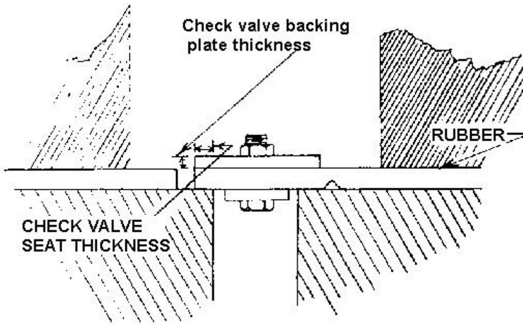
**Check valve backing thickness in inches**
