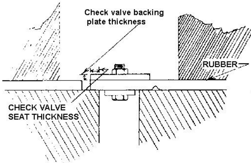
**Check valve seat width in millimeters**
