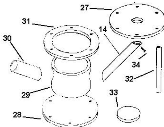
**Welded hydram, impulse cavity: exploded view**
