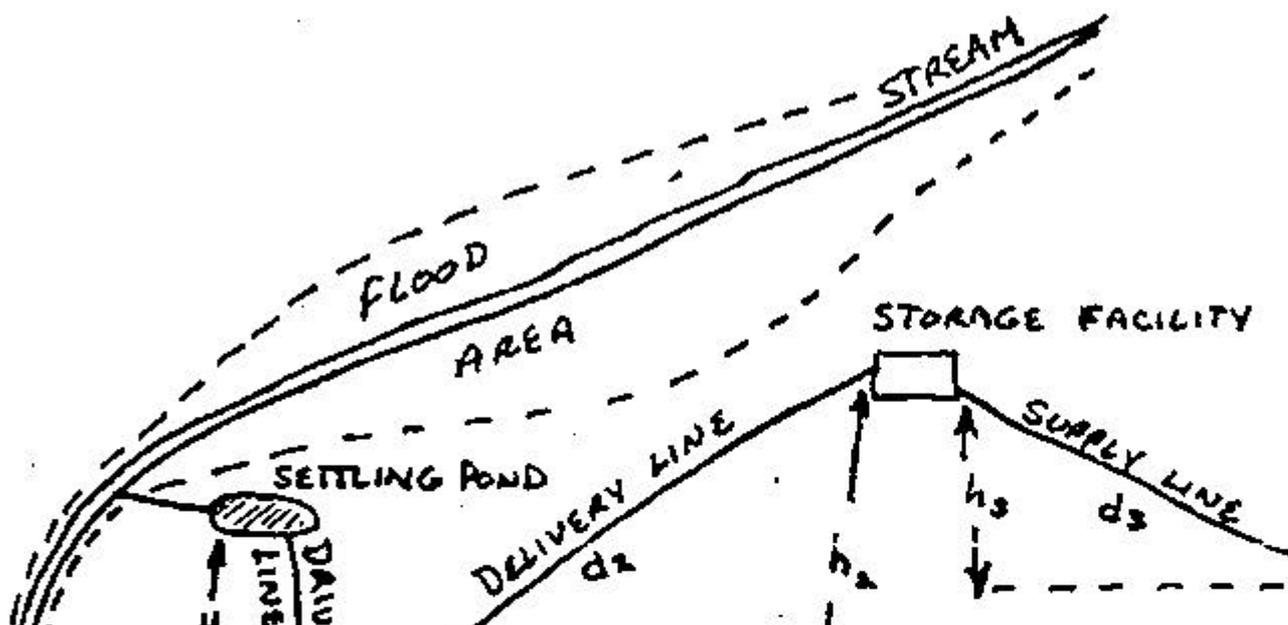
Diagram of hydram system for site selection
