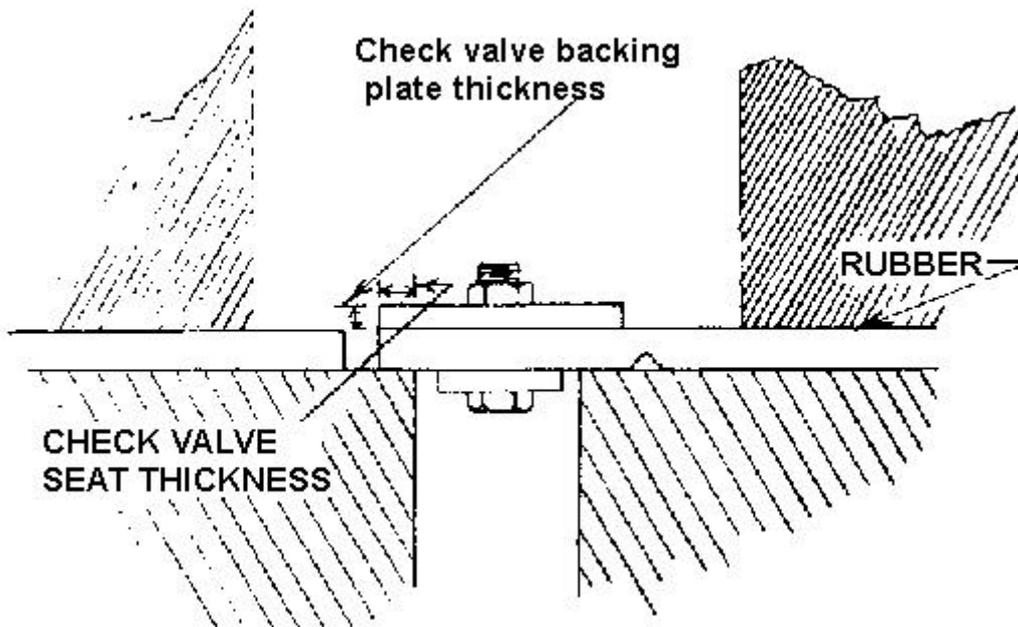
**Check valve backing thickness in millimeters**
