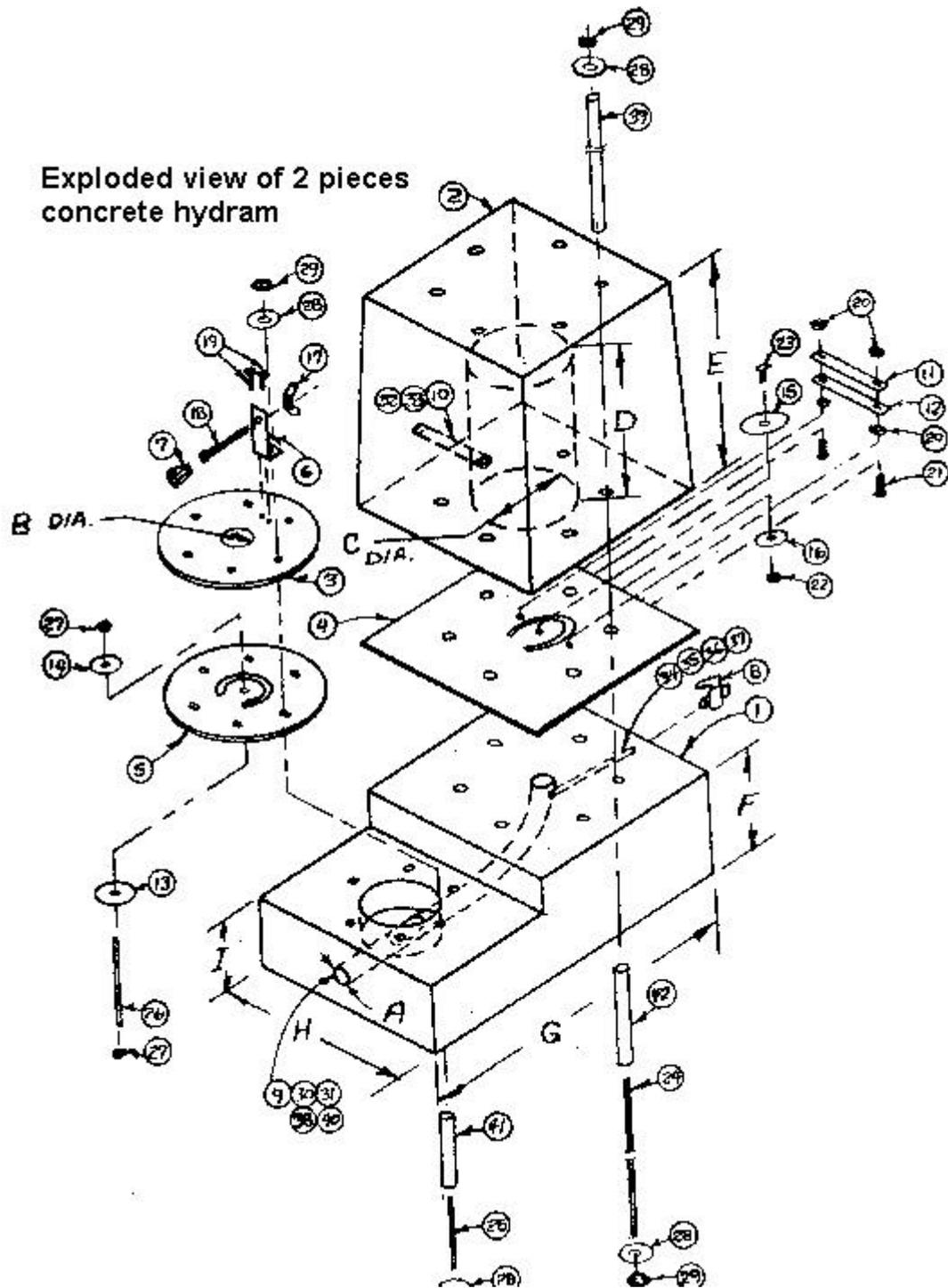
Exploded view of 2 - piece concrete hydram
