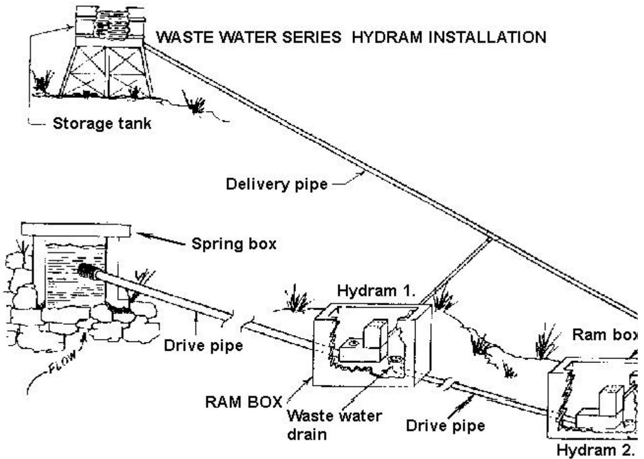
Waste water series hydrum installation
