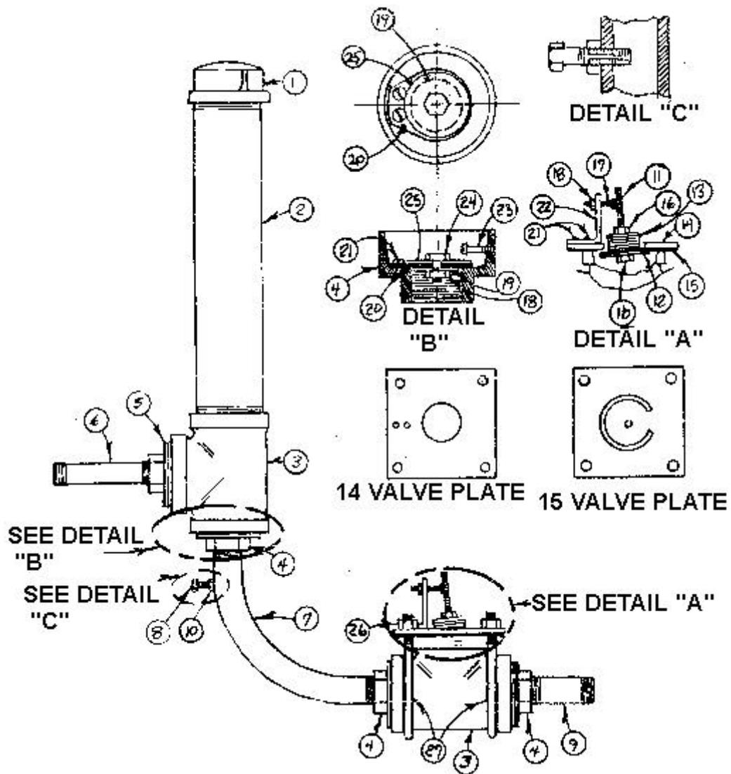
Pipe fitting hydram with field-made valves
