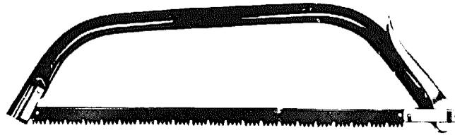
FIGURE 1.27: TUBULAR STEEL FRAME BOW SAW
