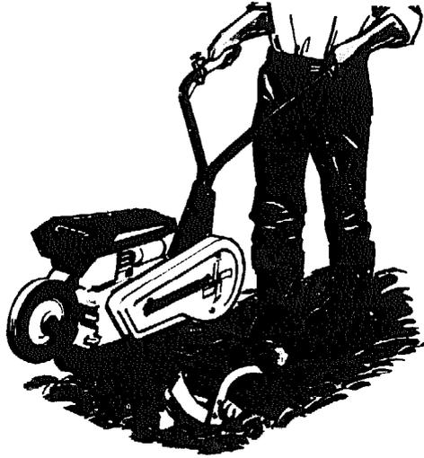
FIGURE TN 6.14 : SMALL SINGLE-AXLE TRACTOR WITH ROTAVATOR BLADES MOUNTED ON DRIVING AXLE
