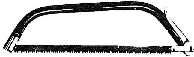
FIGURE 1.27: TUBULAR STEEL FRAME BOW SAW
