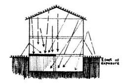
In homes with 2 or more stories above ground, the extent of the basement ceiling modification can usually be reduced to 12' x 12'. Note, however, that vertical side walls may be required if the basement wall exposure exceeds two feet.
