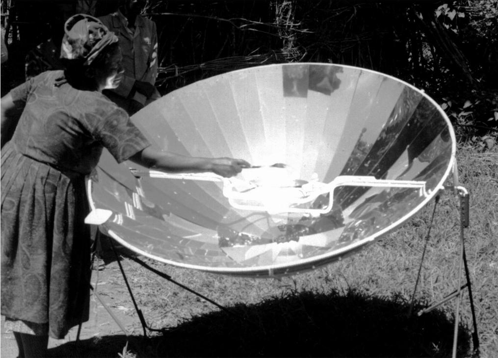
Figure 1: Roasting coffe with the AMSI solar cooker
