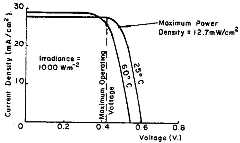
FIGURE 17 – EFFECT OF CELL TEMPERATURE ON V-I CHARACTERISTIC
