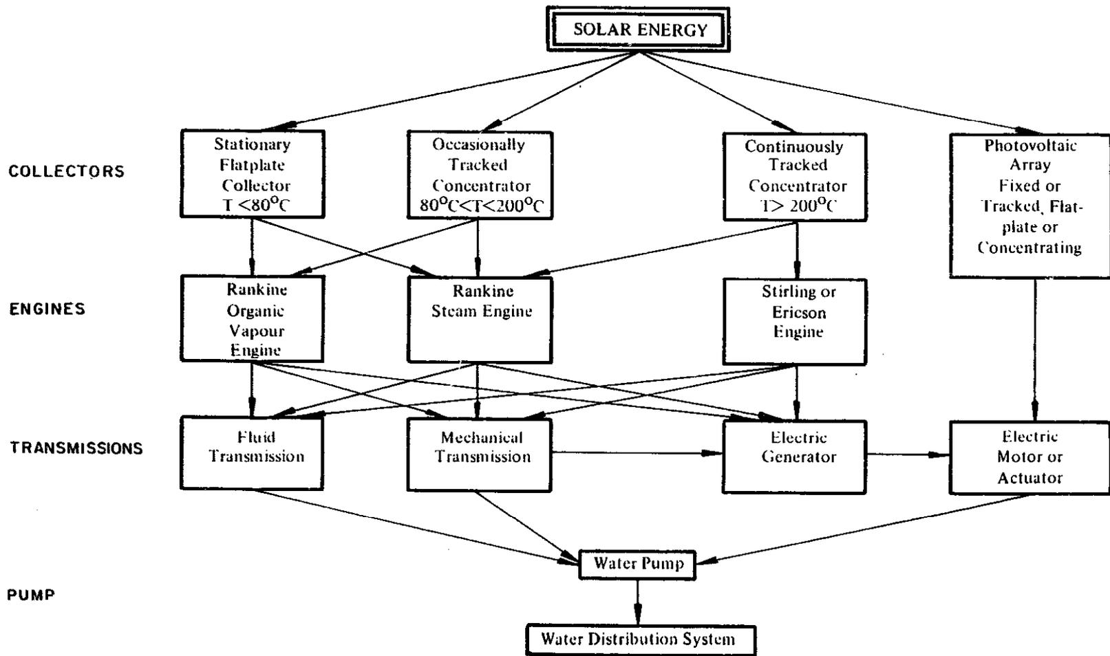
FIGURE 2 - FEASIBLE OPTIONS FOR SOLAR - POWERED PUMPING SYSTEMS
