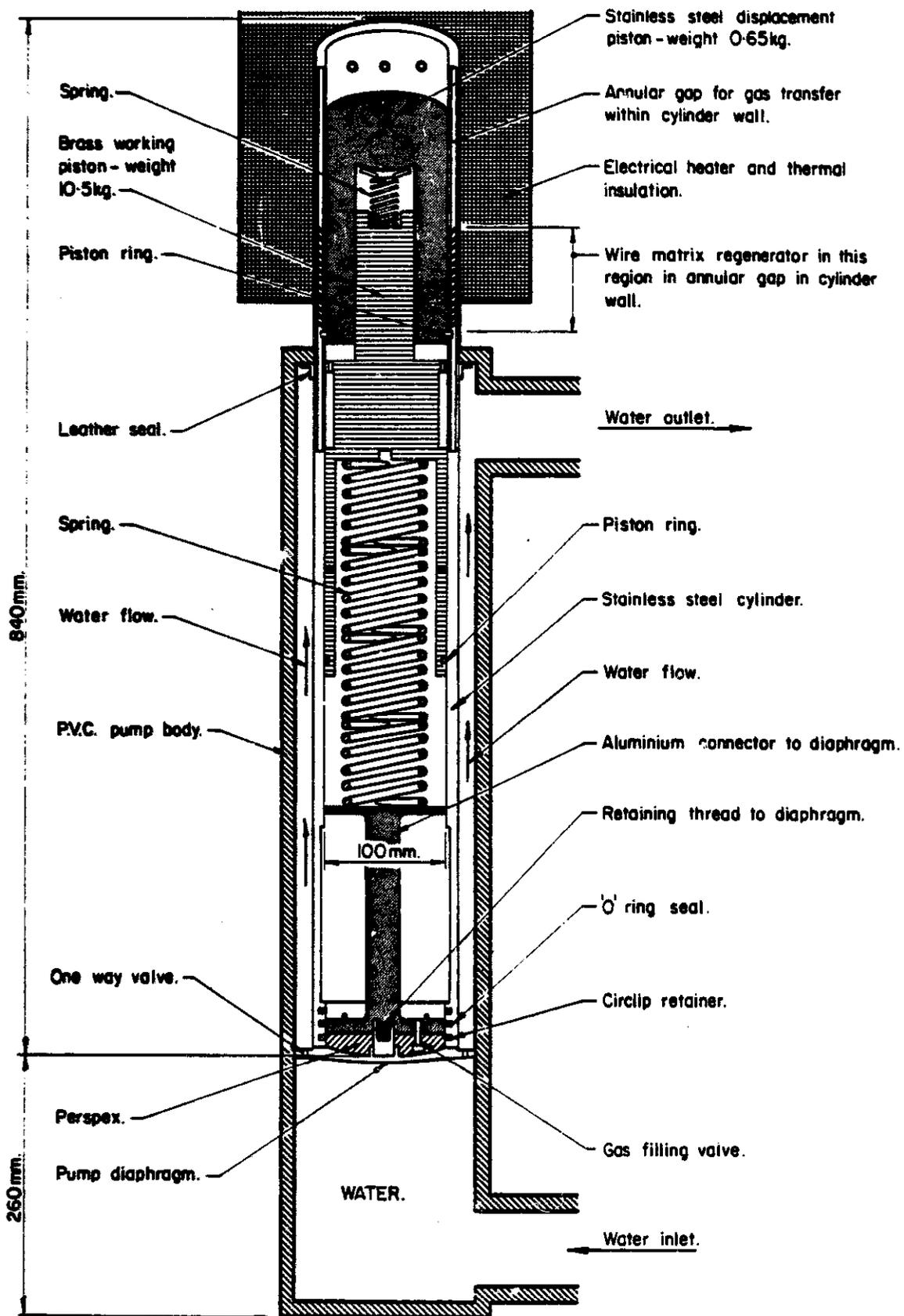
FIGURE 49 - GENERAL ARRANGEMENT OF SUNPOWER INC. STIRLING ENGINE
