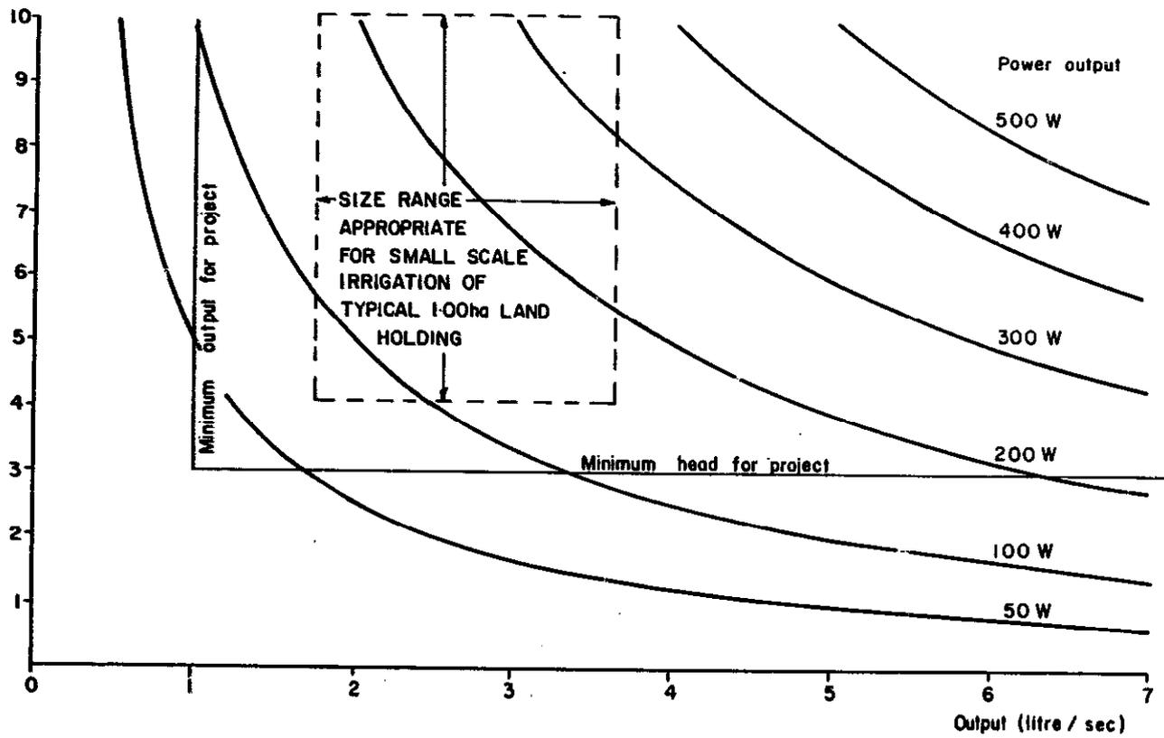
FIGURE 3 - POWER OUTPUT REQUIREMENTS FOR VARIOUS HEADS AND DELIVERY RATES
