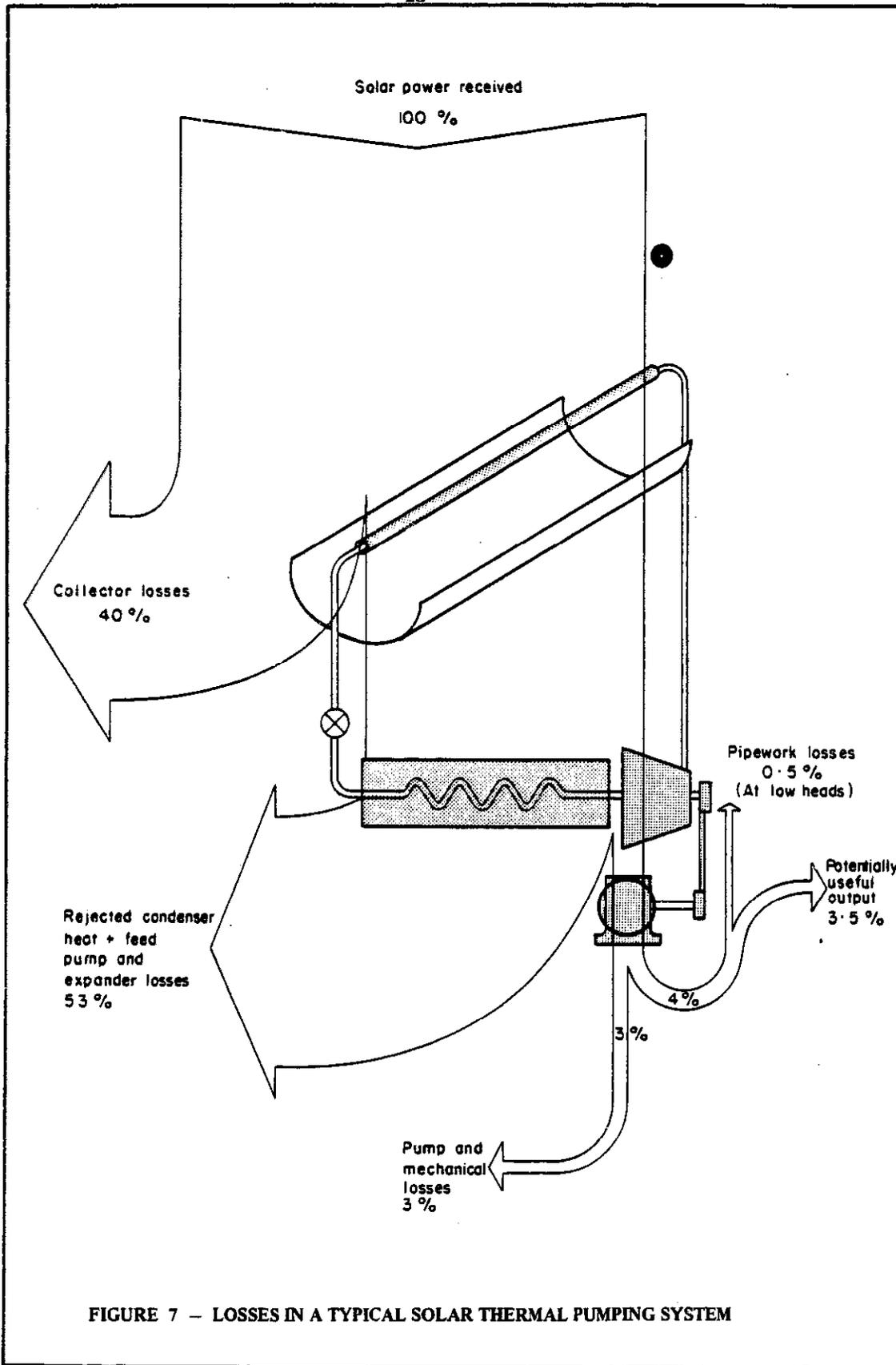
FIGURE 7 - LOSSES IN A TYPICAL SOLAR THERMAL PUMPING SYSTEM
