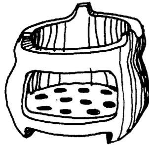
4. *This stove has holes for secondary air in the wall of the combustion chamber.*
