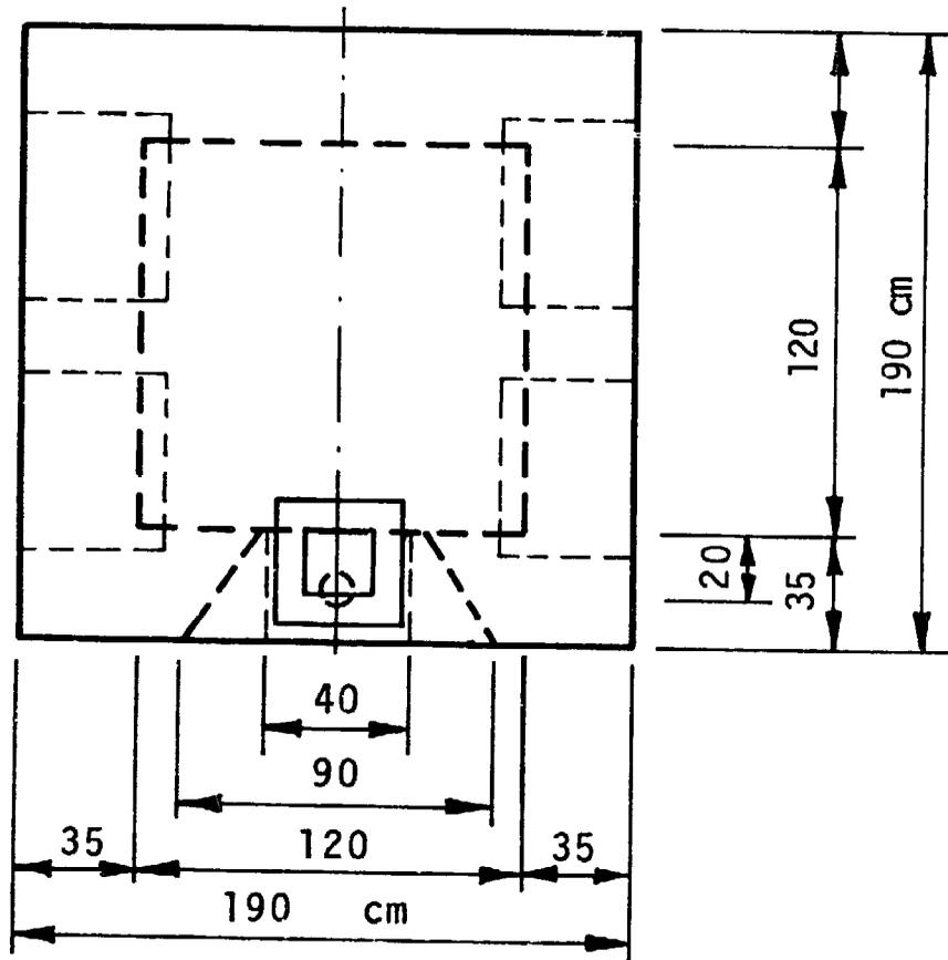
That is the basic design of the oven. A few helpful improvements are recommended. The thin metal sheet covering the ledge could be replaced by an iron plate, say 2 mm thick, of the same shape, hinged along the front edge so that it can be flipped up to expose a hole in the ledge through which the embers can drop straight into a bucket recessed into the oven wall. This is neater and cleaner than letting the hot embers and ashes fall on the floor.
