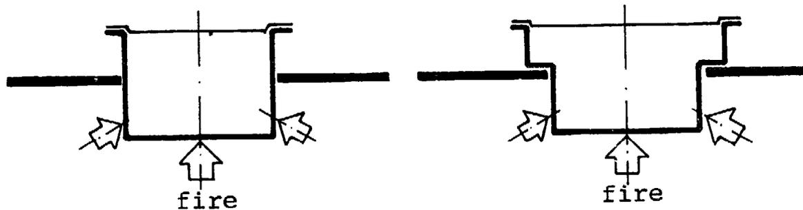
For a smoke-free room and for proper functioning of the stove cooking pots should sit snugly on the cooking stove. It is very useful to have rings, made of cast-iron, to enable adjustment to the different diameters.
