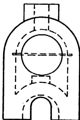
Use mud plaster to close in the front of the oven up to the drum. Use drum lid as a door. Build chimney extension.
