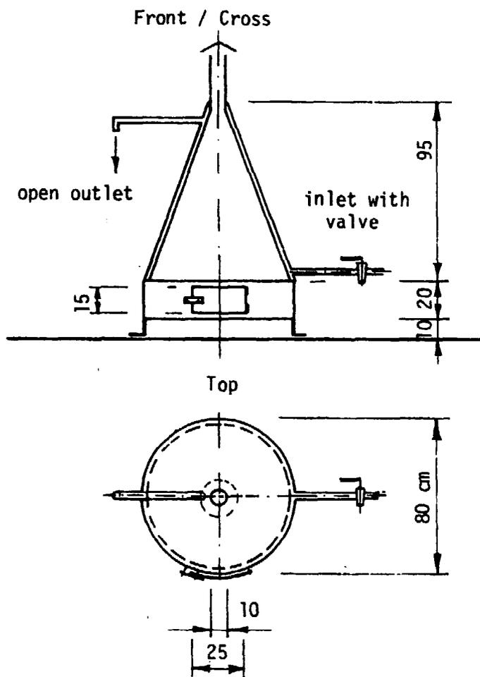
It was a double cone of galvanized-iron sheeting, one inside the other, with a gap of two or three millimeters between them. Water entered at the bottom and came out at the top. The cone was mounted on a fire box in which old newspaper were crumpled up and set ablaze. Within a few seconds the outflowing water was hot. Once the fire is lighted, the water should be allowed to flow, or steam pressure may build up and burst the cone.
