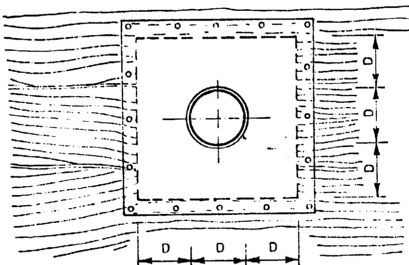
To prevent heat transfer from the pipe to the ceiling materials a space, all around the metal pipe, of the diameter of the pipe (or even with more distance) is required.
