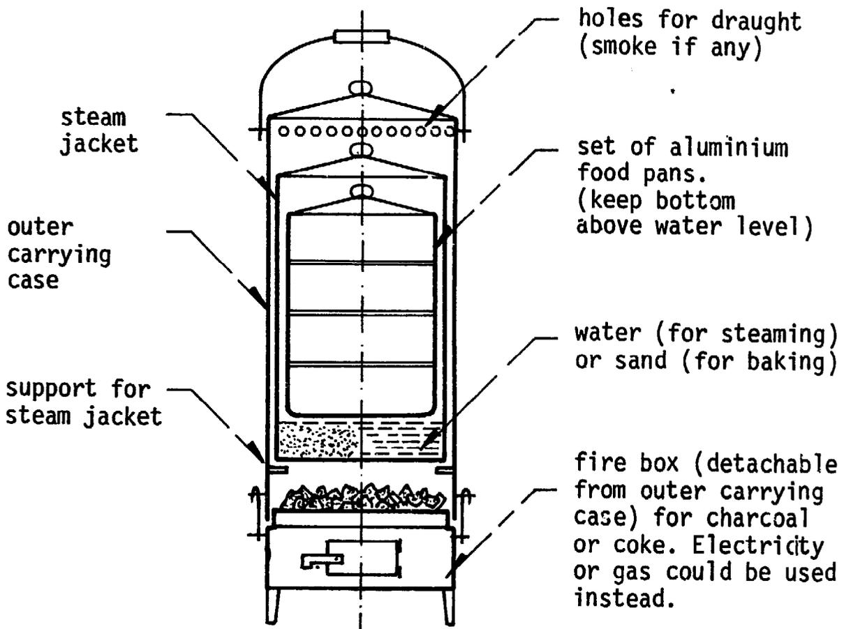
For steaming the food, the steam jacket holds 2.5 cm of water below the pans, but not touching them. For baking, the water is replaced by sand. Obviously baking and steaming cannot be done together. All frying, e.g. of onions or spices for curry, must be done separately before setting up the food in the cooker. There may be some limitations to what the Ic-Mic will do, but the advantages are enormous.
