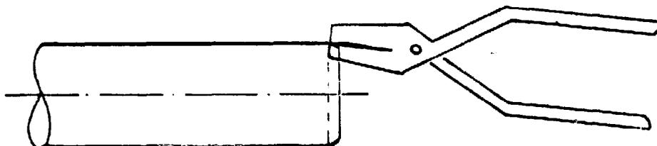
To enable easy fitting the narrow end of the pipe should be prepared this way (and where necessary also the wide end - to keep the air gaps small).
