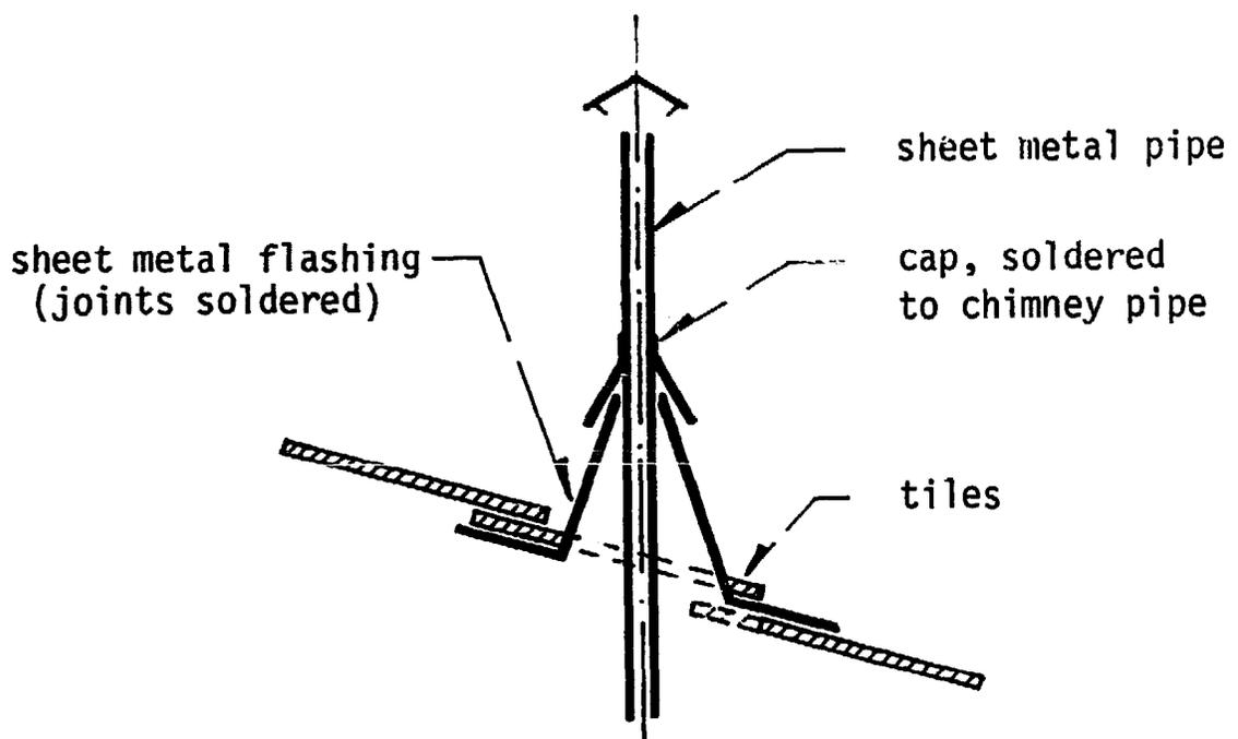
CHIMNEY PIPES ABOVE ROOF TOP
