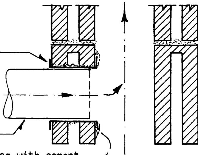
CROSS VIEW of chimney, made with hollow blocks
