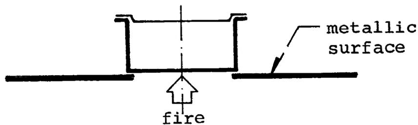
It is essential that much of the bottom (and possibly also the sides) is exposed to direct heat.
