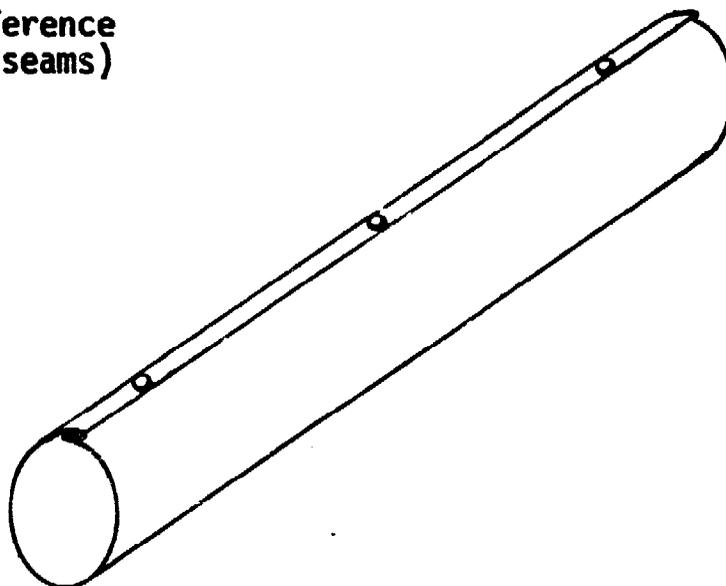
Sheet metal pipes may be riveted or folded. If folding is applied some rivets are required to prevent the seams' opening.
