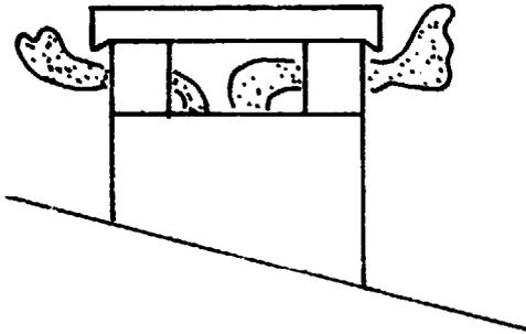
The top of a chimney requires a hat for protection from rain. However, the design may need to be in such a way that the draught is increased, even with wind from the side (without providing back-flow to the stoves).
