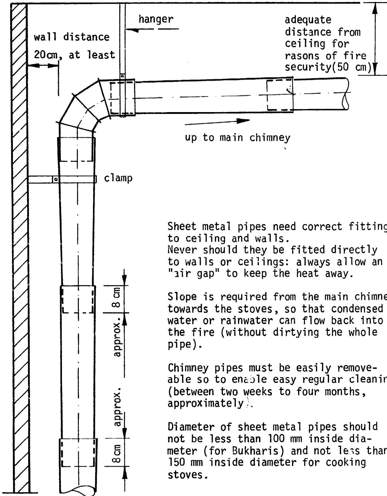
Sheet metal pipes need correct fitting to ceiling and walls. Never should they be fitted directly to walls or ceilings: always allow an "air gap" to keep the heat away.
