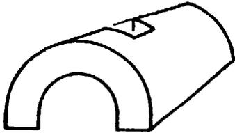
Construct a small mud brick vault leaving a hole (approx. 15 x 15 cm)
