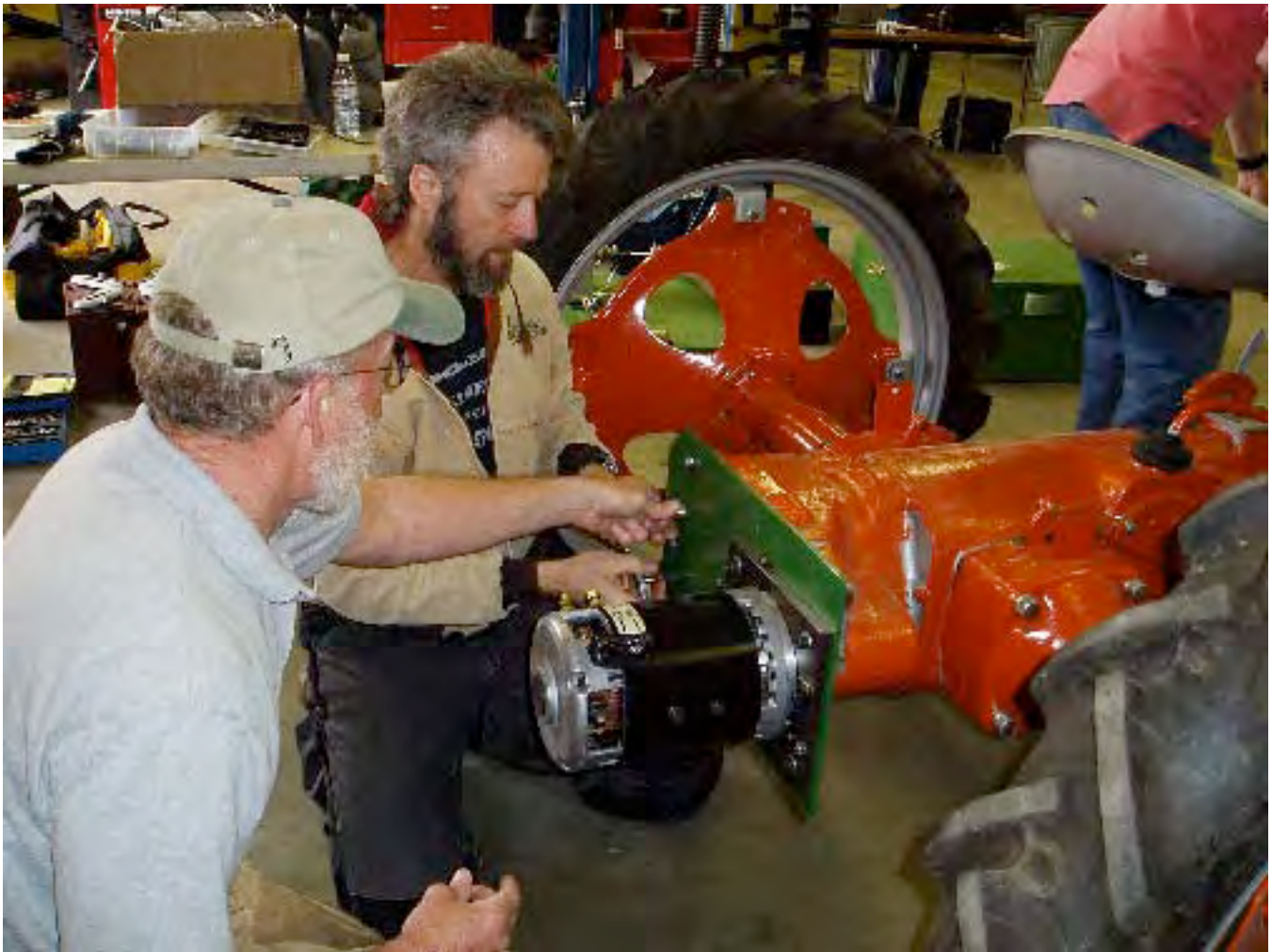
Motor plate installation.
