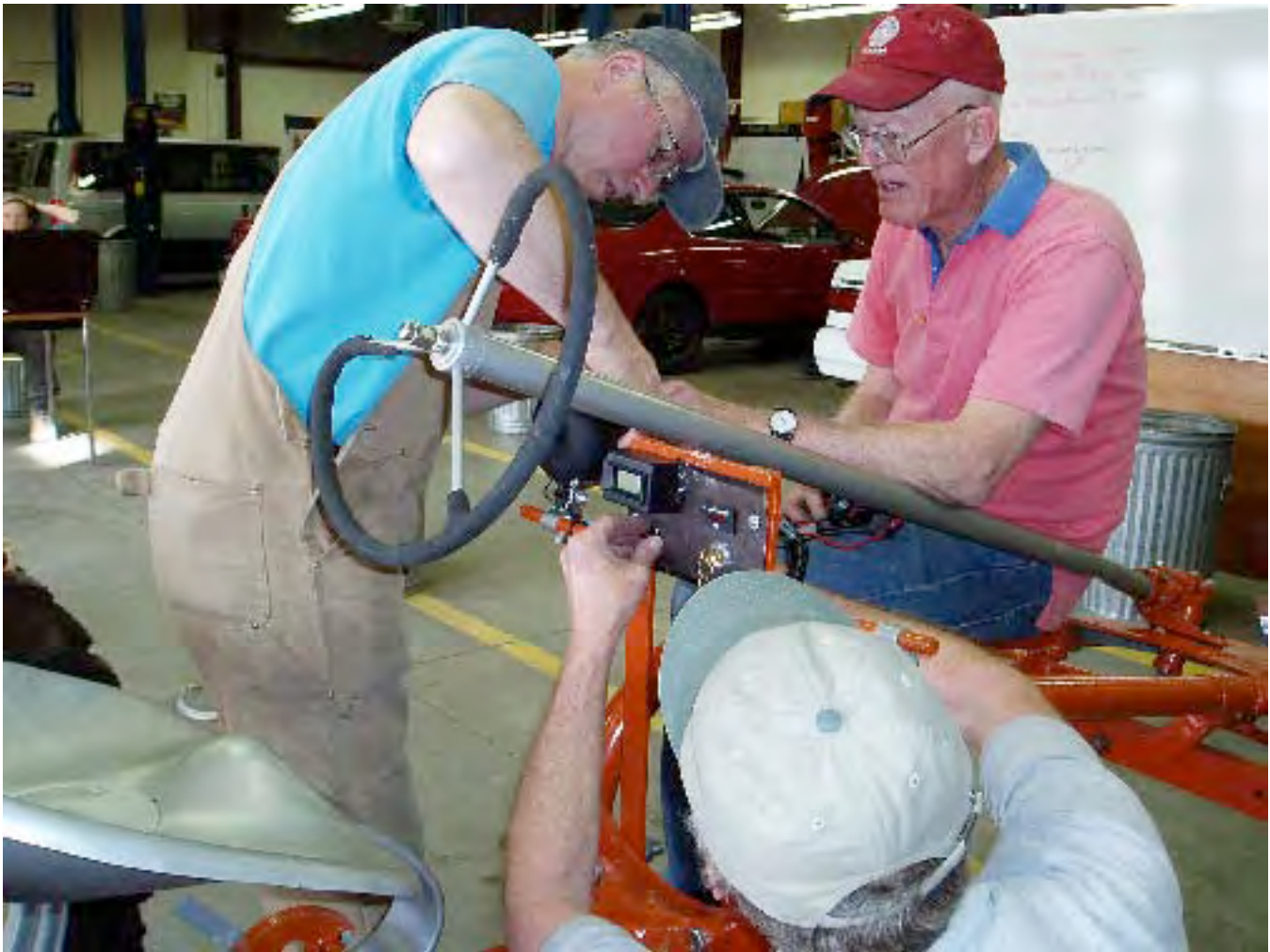
Instrument cluster installation.
