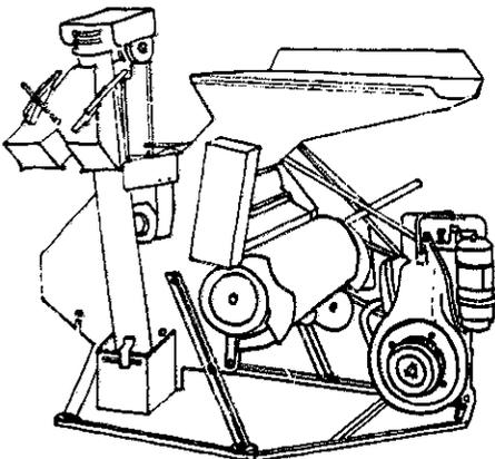
The Bamba tropical sheller is designed for African millet, sorghum and maize and can be operated by one person. It is powered by either a 5.5hp electric motor or 9hp petrol or diesel engine or with power take-off for any tractor. The output per hour is 1500kg of maize or 300-500kg of millet.
