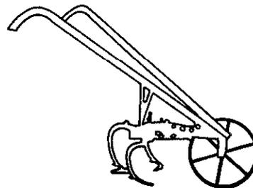
for different types of work if necessary. The cultivator is available with various attachments for weeding, hilling, ridging or furrowing. It has a capacity of 4-5 ha/h and a working width of 250-350mm. The net weight of the cultivator is 17kg.
