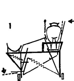
Sheep enters race and is secured in a cage. All movements of the machine initiated by foot levers.
