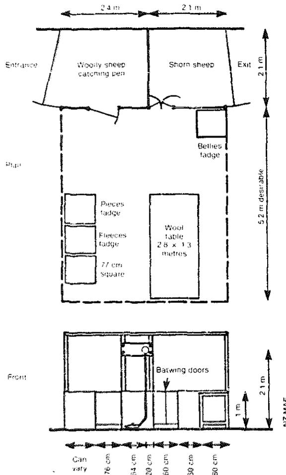
*A small general-purpose building with a single stand can comfortably handle 400-600 sheep. Blade shearing, portable machines or fixed equipment can all be considered.*
