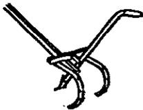
**VIKAS JR. CULTIVATOR** The Vikas Jr. is a simpler version of the R.N. Cultivator above. The width of the 3 tines is easily adjustable. A mouldboard plough, seeding attachments, and sweeps of various sizes can be supplied. The area covered by the Vikas Jr. is 1.2-1.6ha per day.
