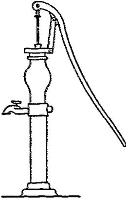
The five models listed here are capable of both raising water and forcing it to a higher point. They have in common the following features: mainly cast iron construction; three-pivot handle system with stuffing box and pump rod guide; air chamber; and valved outlet spout.
