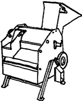
The M30 maize sheller standard model (illustrated) is supplied with a 240mm diameter pulley and carrier arms. The power requirement is 3 to 5hp and output is 2000 to 3000kg/h. The following accessories can be fitted:
