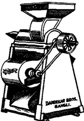
This machine (illustrated left) can either be hand-operated or power-operated, requiring a 5hp motor or engine. The shelling capacity is 1500kg/h.
