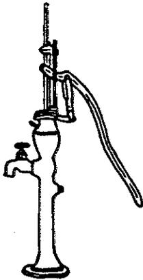
Similar to the above lift and force models the five listed here have two main additional features: adjustable fulcrum position for varying the mechanical advantage and stroke length; and extra pump rod guides to maintain vertical reciprocating motion.
