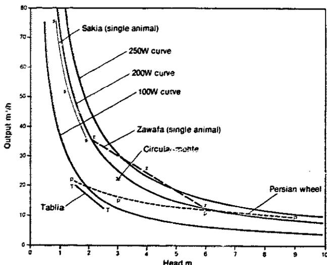
Fig 4. Discharge versus head performance: Traditional animal-powered pumps.
