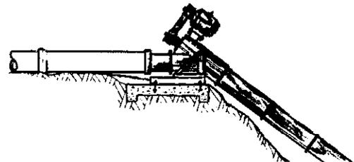
1m head. Alternatively a 9hp model can deliver 330m<sup>3</sup>/h at a total head of 4.6m or 950m<sup>3</sup>/h at 1m.
