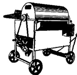
from 6-8 quintals/h (using 10hp motor) up to 10-12 quintals/h (using 20hp motor).
