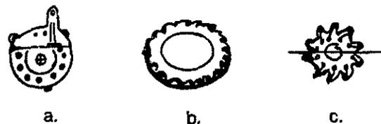
Fig.8 Seed metering wheels and plates: a. vertical cell-wheel, b. horizontal feed disc, c. spoon disc.
