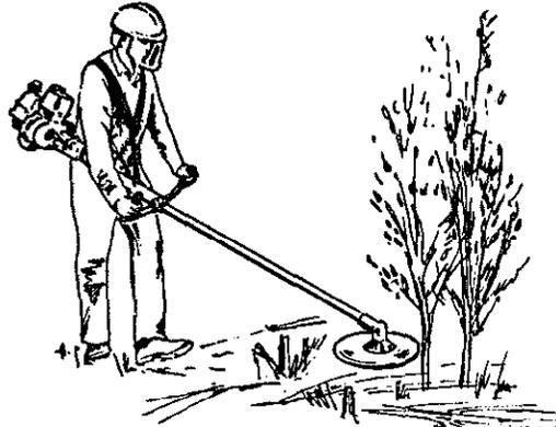
OPERATOR WEARING PROTECTIVE HEAD GEAR
