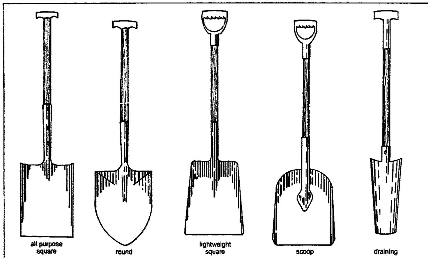
The shovel, which has been employed since the earliest times in both agricultural and construction activities, is a tool used to move loose or unconsolidated materials short distances. It differs in form and function from the spade (see Section 1, Seedbed Preparation) which is essentially a digging instrument.
