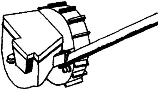
Fig.4 Rolling seed drill — single-row vegetable seeder.
