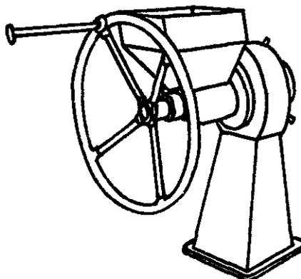
**DUNIA HAND-OPERATED GRINDING MILL**
