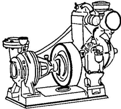
**KIRLOSKAR PUMPSETS** A range of diesel engine and electric motor driven centrifugal pumpsets are available. The engines of the vertical water cooled single-cylinder variety 5 to 8.7hp, are connected directly to end-suction type pumps suitable for total heads from 6 to 26m with corresponding outputs from 120 to 36m<sup>3</sup>/h. The electric motor pumpsets are capable of twice this performance.
