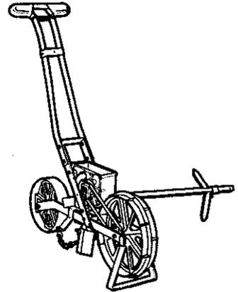
Precision seeders can be used to plant a wide variety of vegetable seeds through six easily interchangeable seed plates which regulate the seed flow from the hopper to the planting mechanism. The seeder when in use opens the soil, plants the seeds at the desired spacing and depth, and covers the seeds while marking the adjacent row.
