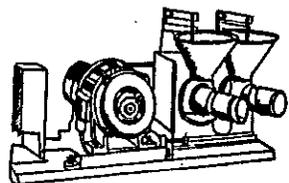
**OIL FRUIT SPINDLE PRESS** Fruits are not warmed prior to pressing in the press (above right). The press-head must however be heated by flame or hot water prior to operation. Power requirement 1.75-3.5kW with an output of 25-70kg/h. Manufactured by Komet in W. Germany and available through:
