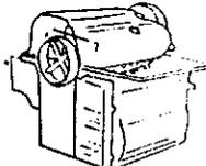
above, with a width of 75cm and a power requirement of 2-4hp. It is suitable for threshing various kinds of beans and other pulses, rice and wheat, and features interchangeable screens for different sizes of grain. The speed can be adjusted by changing the V-belt pulleys between the threshing drum and winnower. The universal thresher has a capacity of 1500kg/h for beans, and an overall weight of 120kg.
