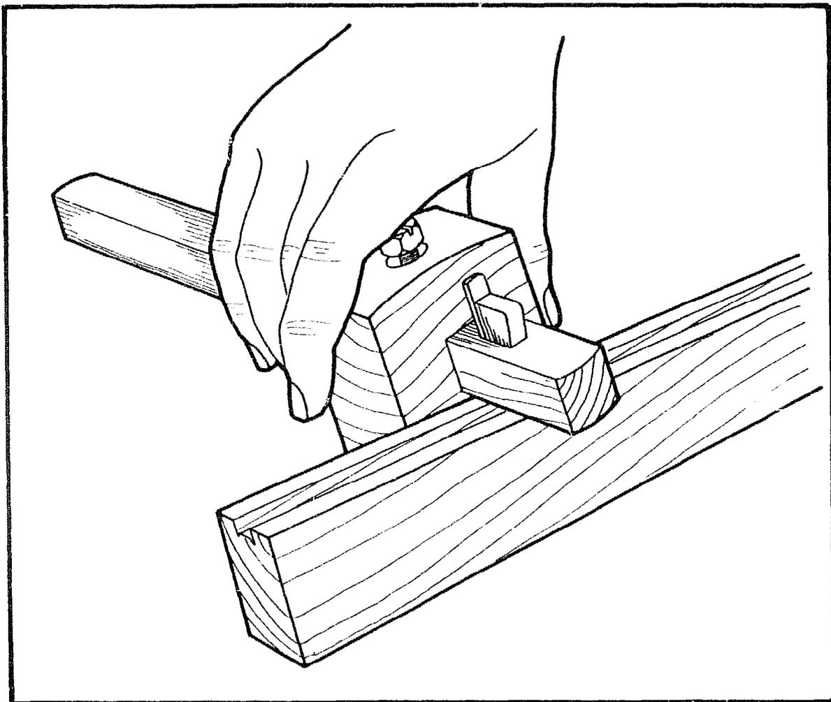
Cutting gauges are very similar to marking gauges, but instead of a metal spur, the stem carries a small knife blade held in position by a wedge. In the drawing the fence is fixed to the stem, using a 6mm bolt as a locking screw, but the wedge method could be just as effective.
