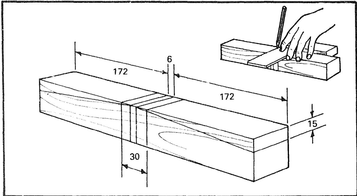
Take the timber prepared for the fence, mark a point in the centre, and square two lines all round 3mm either side. Square two lines all round 15mm either side of the centre mark. On each end, square two lines 15mm below the top edge.
