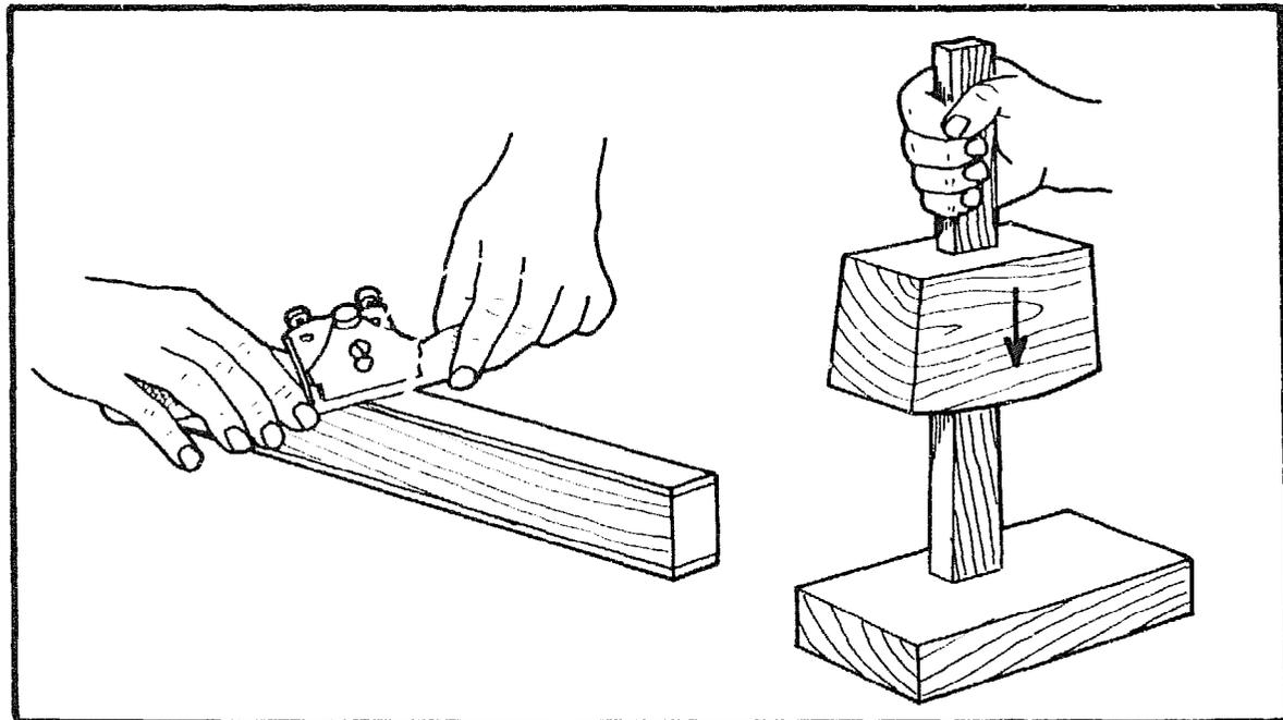
Shape the handle with a spokeshave or a plane down to the lines. To fit it, push the bottom of the handle through the top of the head and tap it down on a piece of wood.
