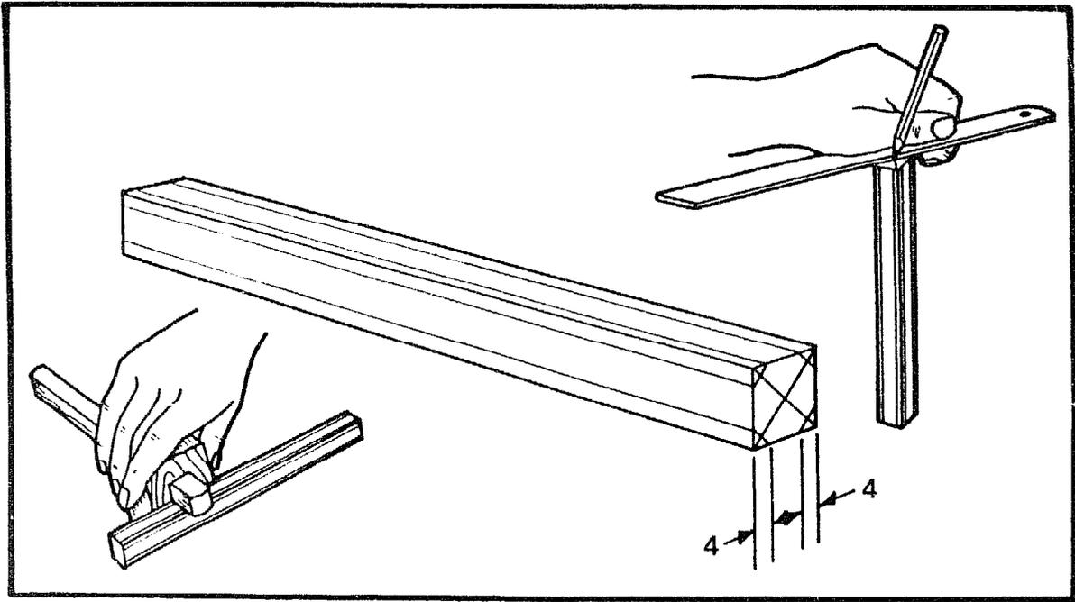
Take the timber prepared for the stock; find the centres of each end by marking the diagonals. Gauge eight lines, 4mm in from each end. Plane off the corners down to the gauge lines.
