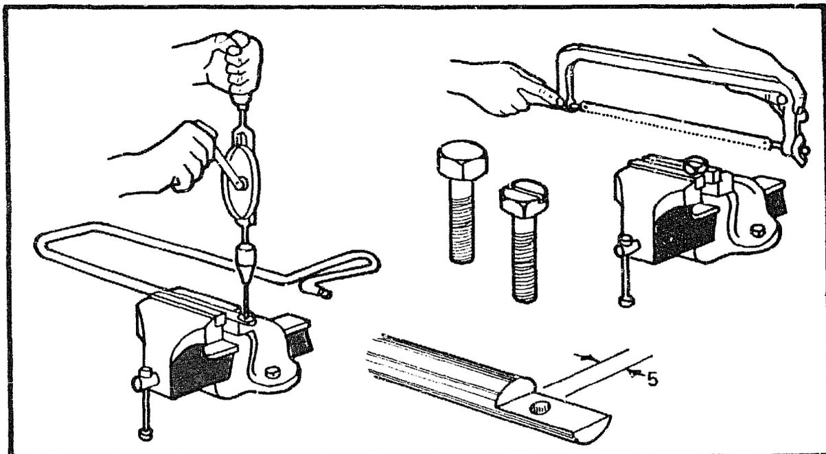
Punch and drill 6mm holes in the end of each leg of the frame. The centre of the holes should be exactly 5mm from the shoulder.
