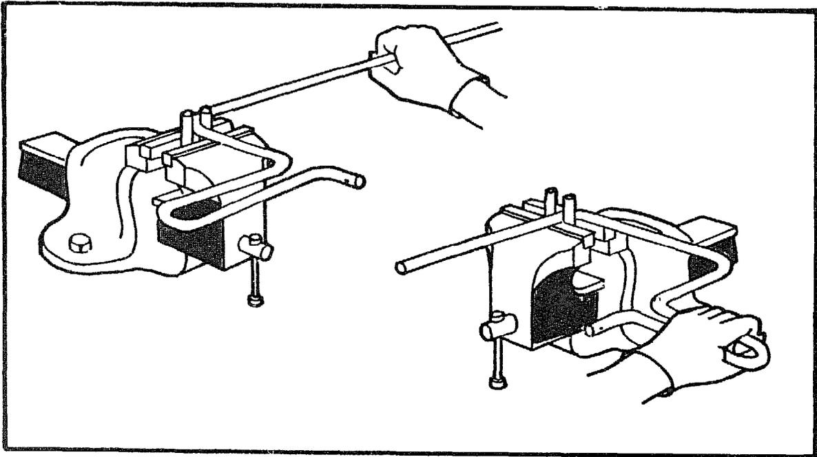
Measure 140mm from the end of the rod, heat it up until red hot, and make another 90 degree bend.
