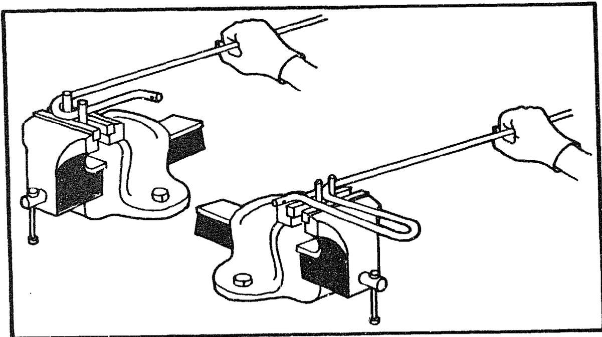
Heat up the rod 120mm from the first bend and make the handle by bending 180 degrees. Opposite the first bend make another 90 degree bend.
