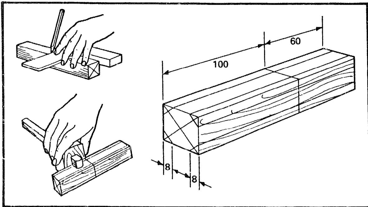
Take the timber prepared for the handles and mark the diagonals on each end to find the centres. Square a line all round 100mm from one end.
