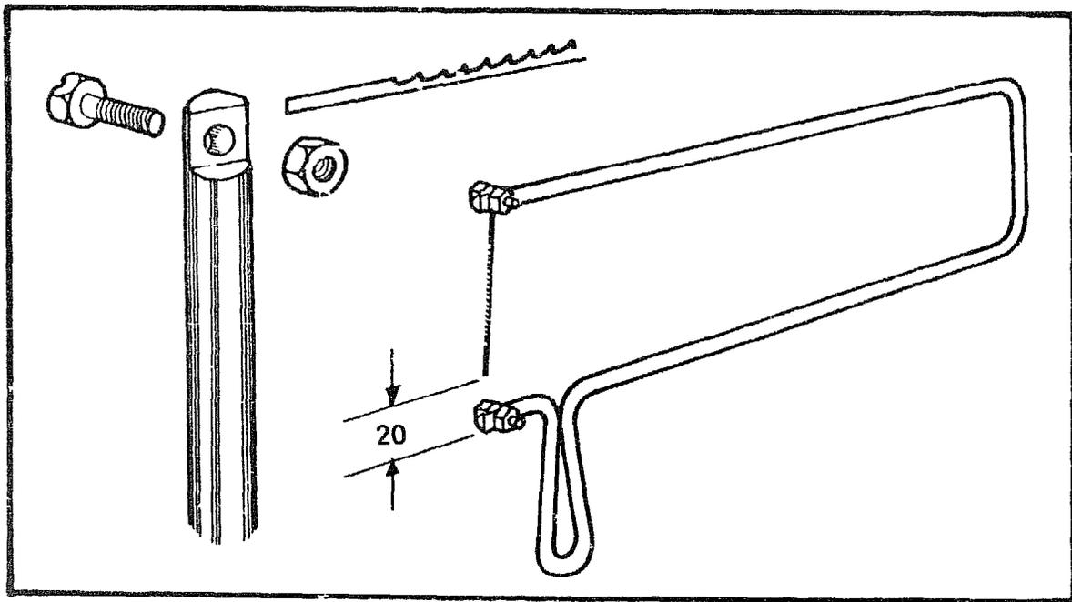
Place the bolts through from the round side of the frame and screw the nut on. The nut should not be able to turn because of the shoulder cut in the frame. Clamp the blade into one leg of the frame.
