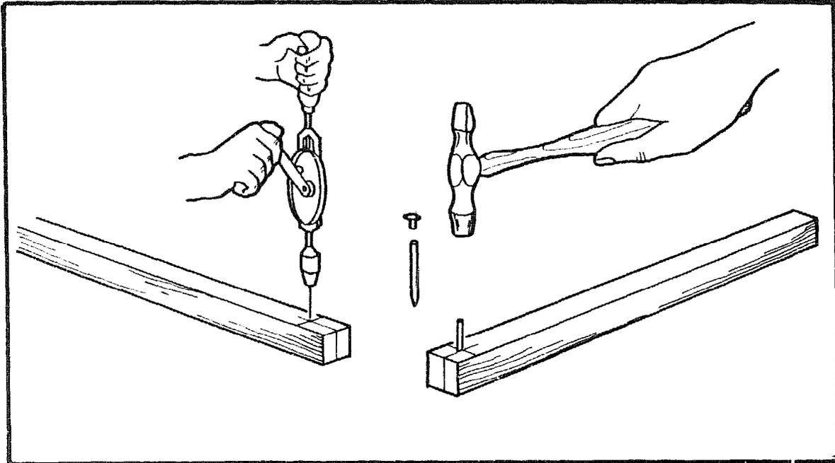
From both sides drill a hole with a bit slightly smaller than the diameter of the nail you will use as the spur. If you do not have a bit small enough, cut the head off a 20mm nail and use this to make the hole.
