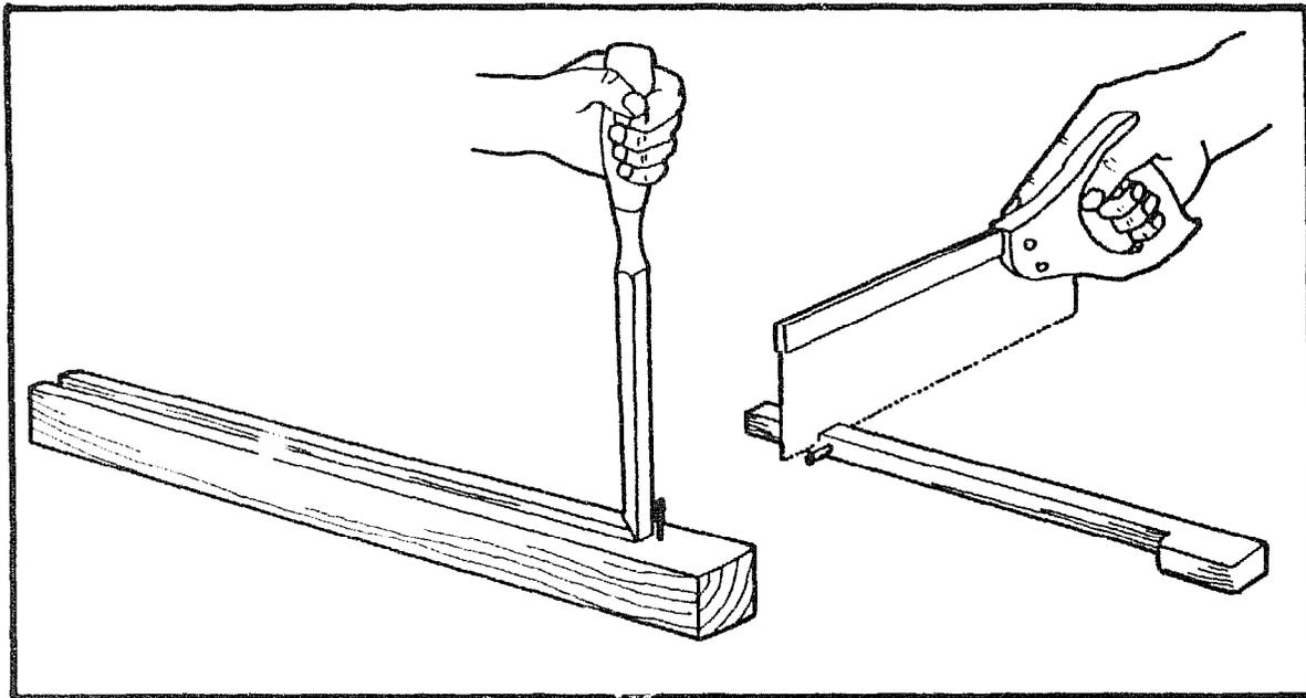
With a 6mm chisel, cut the groove back to within 3mm of the spur in the stem.
