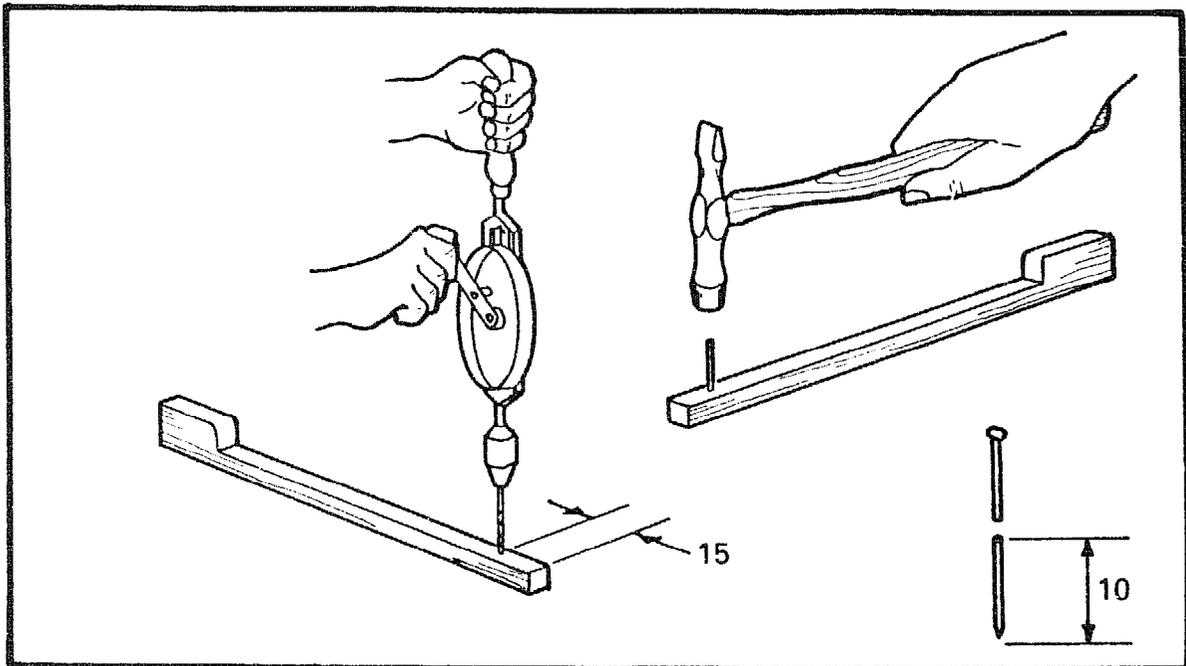
Use the same drill to bore a hole in the slider, 10mm from the end. Take another 25mm nail and cut it down to 10mm in length. Carefully hammer this into the slider, again leaving 5mm sticking out. Drilling the hole first should prevent the timber splitting.
