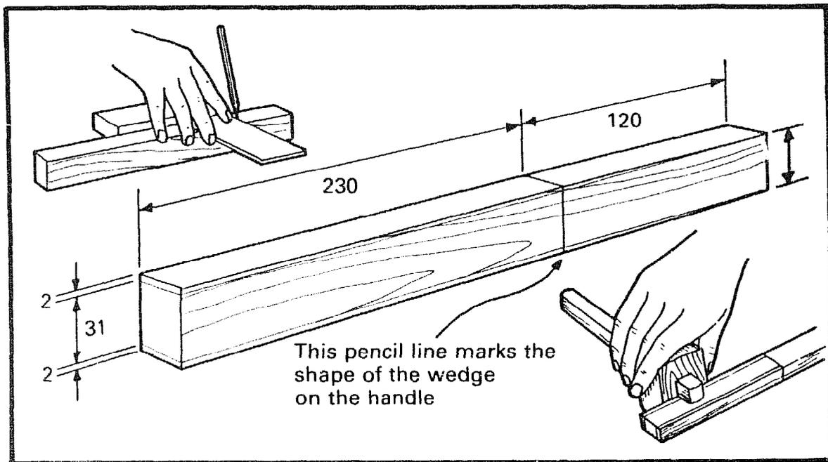
Square a line all round 120mm from the end of the handle. From this line gauge 2mm on both sides, to the other end. With a pencil mark the wedge shape at the top of the handle.
