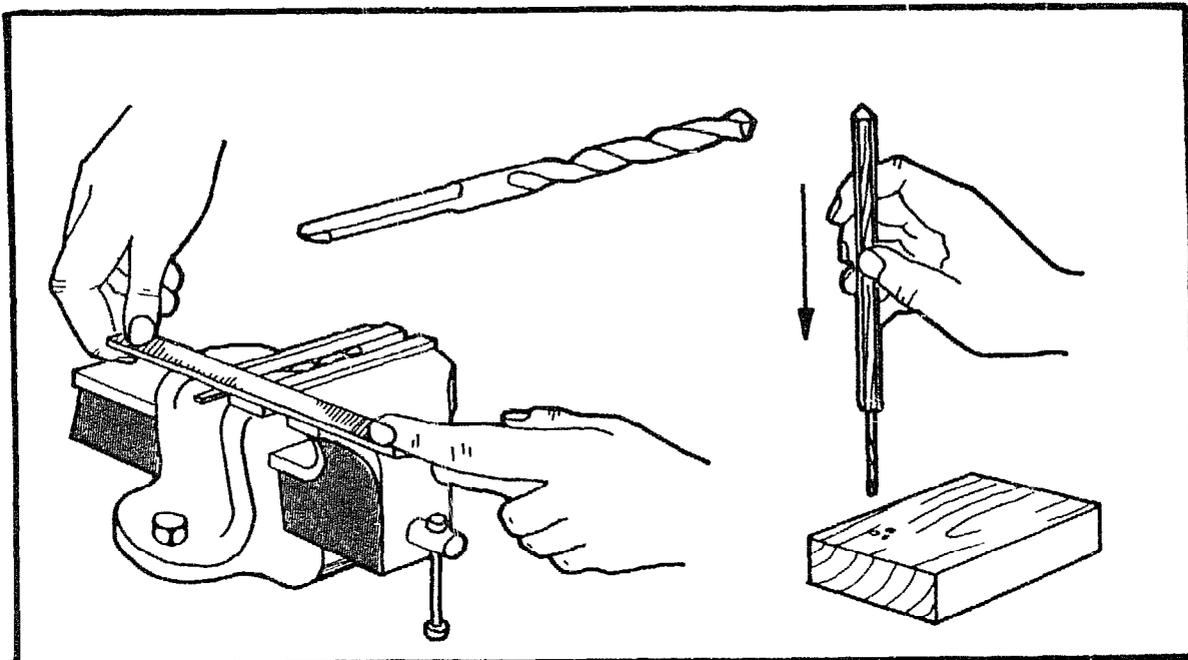
Take the drill bit and file two flats on the shank, and a point on the blunt end. Tap the bit into the stock, taking care not to blunt it. It may be necessary to use a hammer.
