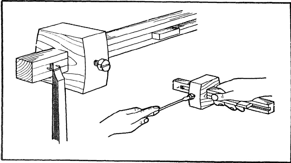
The gauge is set in the normal way by using a mortise chisel to determine the distance between the spurs.
