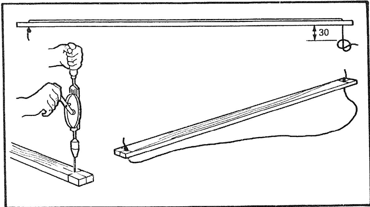
Drill two  $\text{Ø}3\text{mm}$  diameter holes, one at each end of the bow. Thread the string through one hole and tie a knot. Thread the other end of the string through the other hole, and tie a knot 30mm from the hole.
