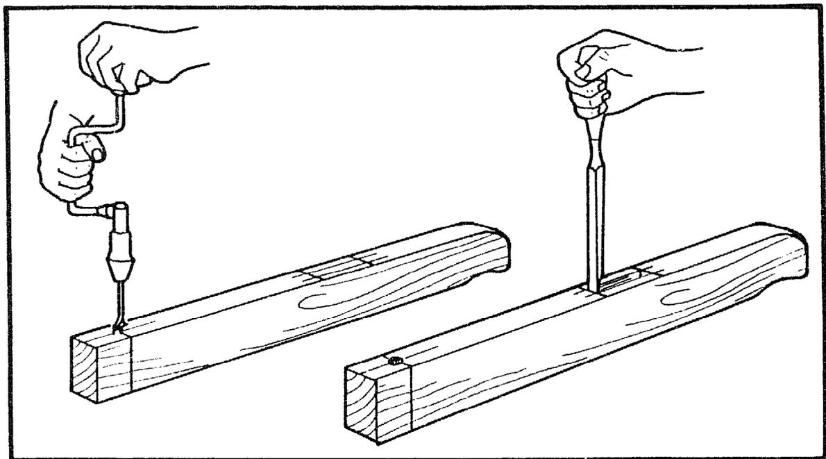
From both sides, drill a  $\varnothing 9\text{mm}$  hole, with a brace and bit. With a 6mm mortise chisel and a mallet, cut the mortise to a depth of 20mm.
