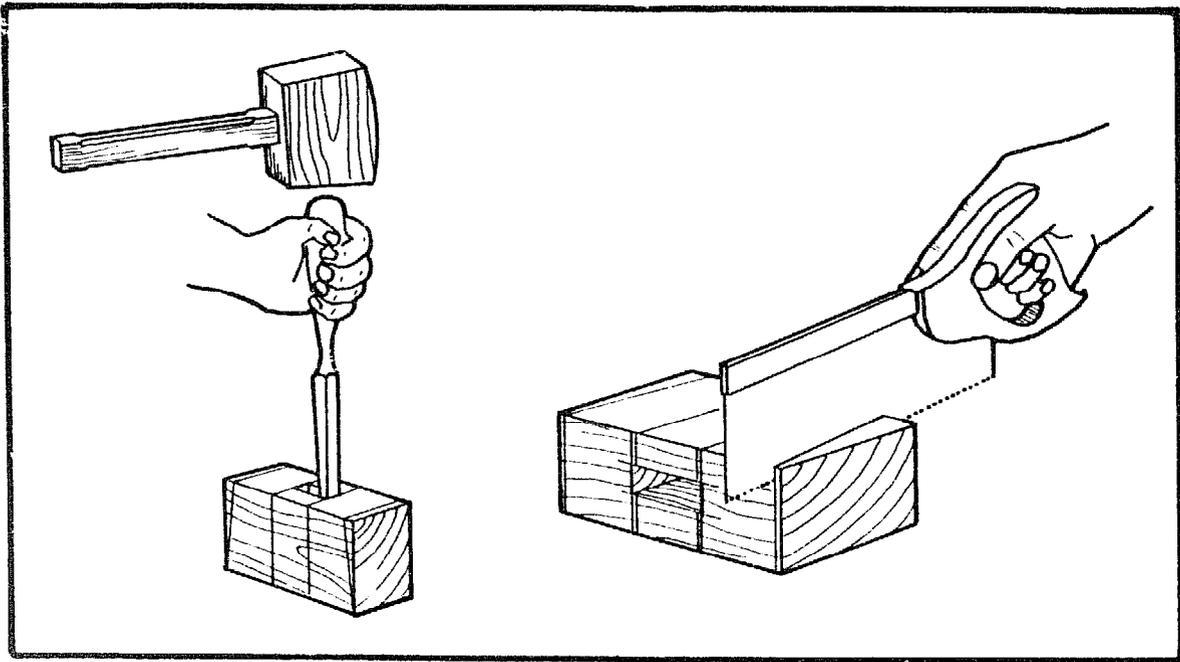
Cut the mortise with a mallet and chisel. Note how, at 34mm, the mortise is 4mm bigger at the top than the bottom. With a tenon saw cut the angled ends of the mallet head.
