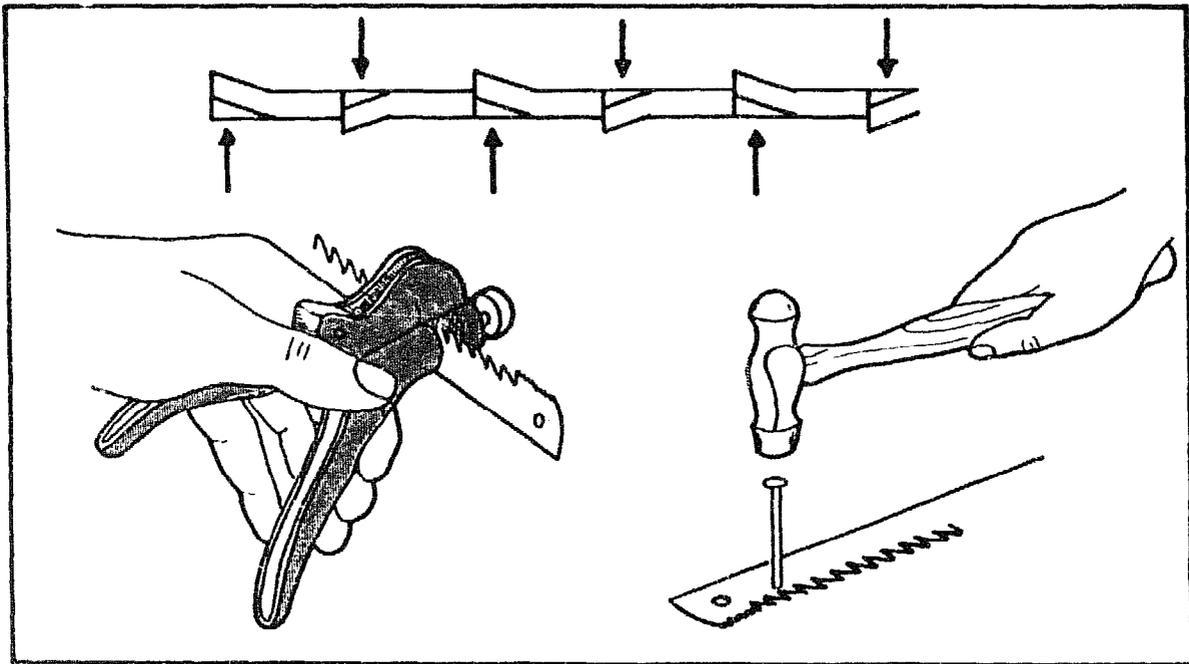
The teeth of the blade now have to be set. Use a saw set if one is available. If not a hammer and a blunt nail can be used to bend the first tooth to the left, the next to the right, and so on.
