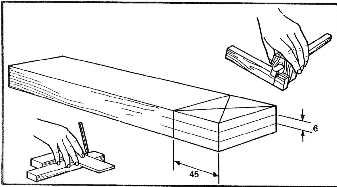
Take the timber prepared for the stock and square a line all round 45mm from one end. Gauge two lines 6mm apart in the centre of the stock. Draw diagonals to find the centre of the joint.
