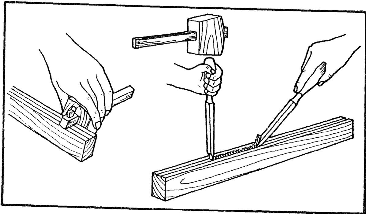
They can also be used for cutting the sides of grooves, with the grain or across it. Run the blade two or three times along the timber to make a deep cut. Remove the waste with a mallet and chisel.
