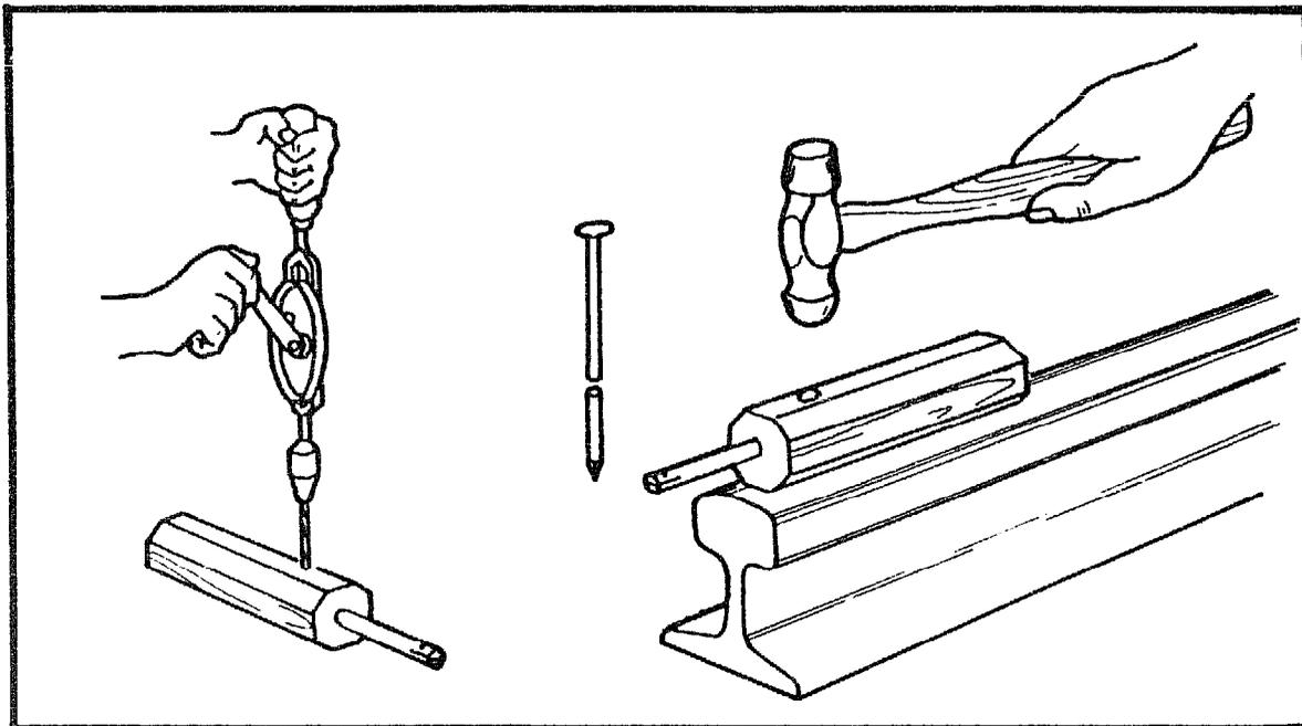
Push the 9mm bars into the handles, with the slot and the hole pointing out. 25mm in from the drilled end of the handle, drill a  $\varnothing 3\text{mm}$  hole right through. Push a 50mm (2") nail through this hole. Cut the end off and rivet the cut end of it with a hammer to hold the two pieces firmly together.
