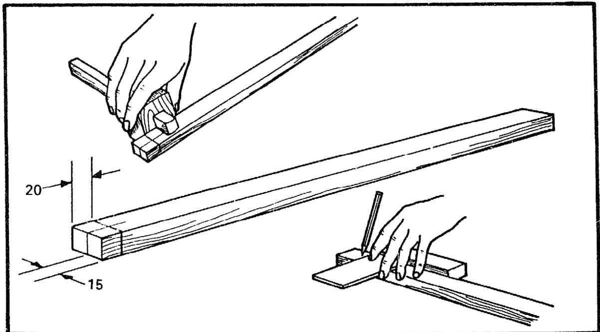
Take the timber prepared for the stem and square a line all round 20mm from the end. On top and bottom, gauge a centre line which should be 15mm from both sides.
