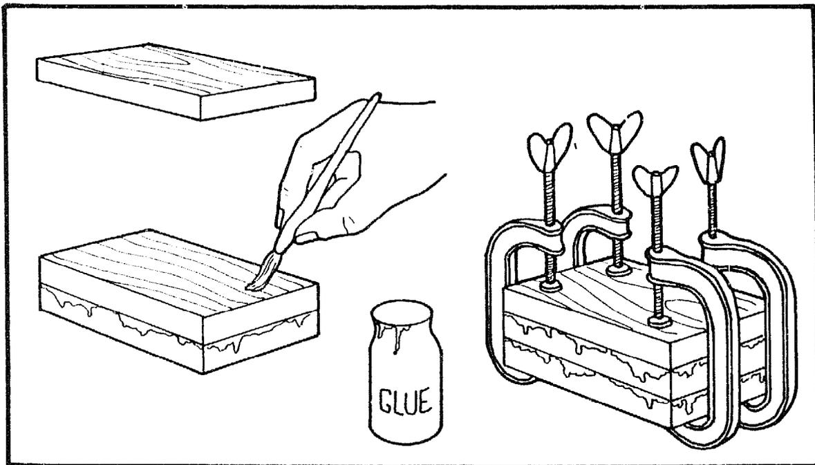
The mallet head can be made up of two or three pieces of timber, glued together. Make sure there are no gaps in the joints. Leave it clamped up for at least six hours.
