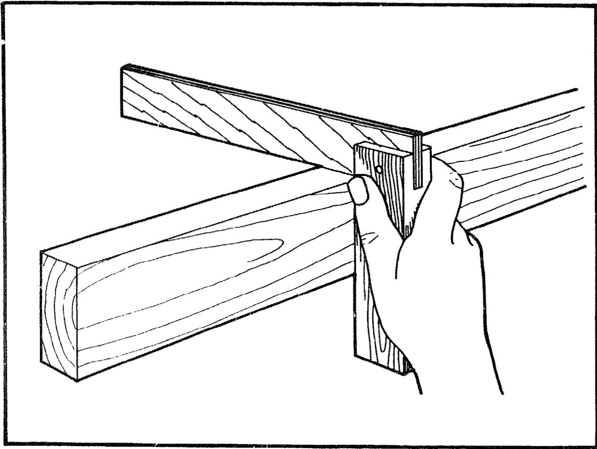
Try squares made of wood are very practical pieces of equipment, and are quick and easy to make. They can be made to any size up to a metre in length; use the dimensions given here only as a guide. When making this tool it is most important that the straight edge and the stock are glued up perfectly square, otherwise all the work done with it will be inaccurate.
