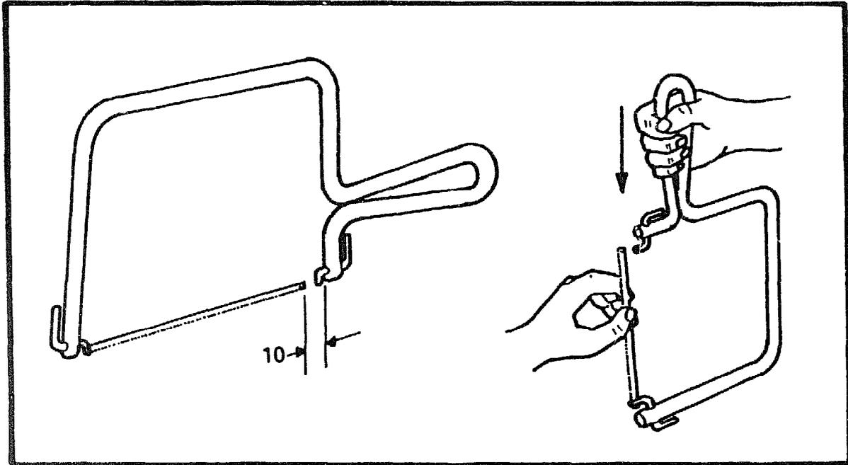
Bend the legs of the frame so that the gap between the two blade holders is 10-15mm bigger than the blade. This gives the right blade tension.
