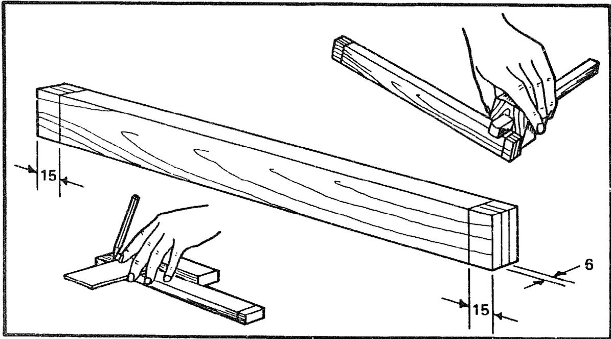
Take the crossbar and mark the shoulders of the tenons by squaring lines all round 15mm from both ends. With a mortise gauge, gauge a 6mm tenon on both ends of the crossbar.
