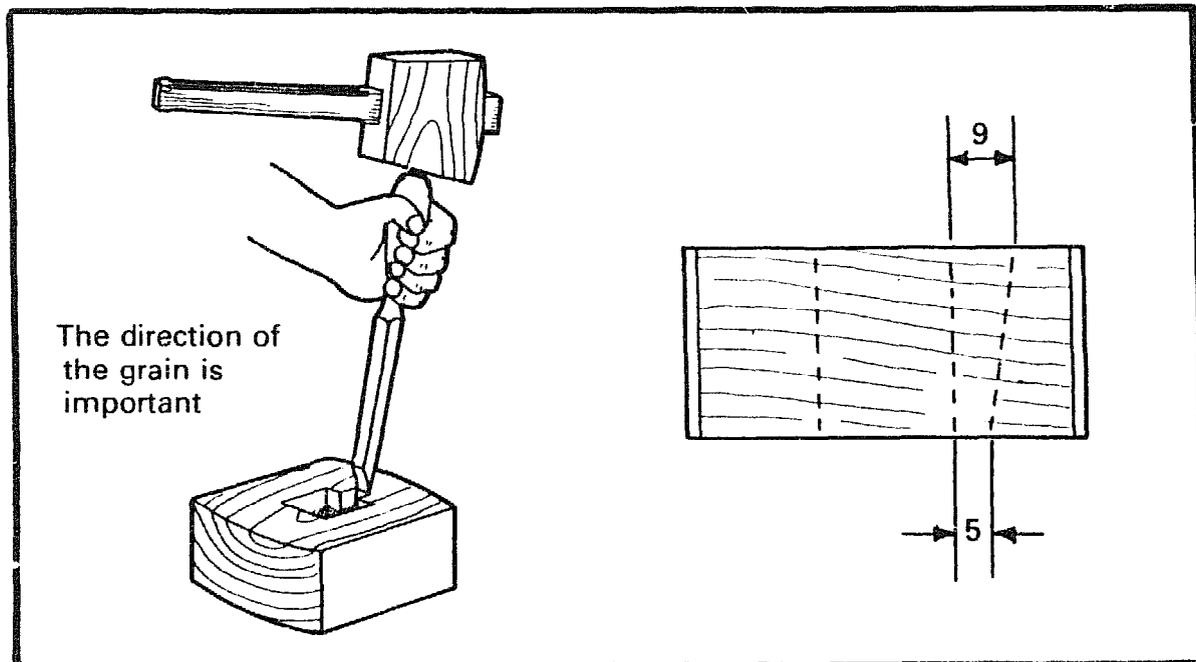
With a 6mm chisel and a mallet cut a sloping groove into the mortise of the fence. It should run from about 9mm at the big end to about 5mm at the small end.
