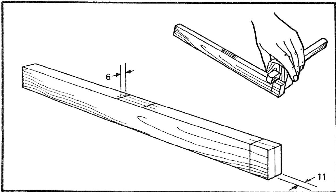
Use a mortise gauge to mark a 6mm mortise, in each of the side frames, for the crossbar. Gauge a line in the middle of both edges of each frame, to mark the points for drilling the holes to take the blade sockets.
