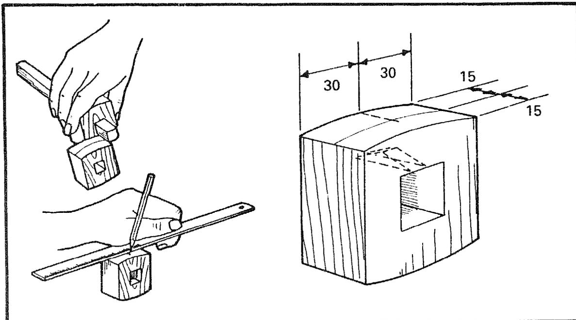
To make the fence follow the directions on pages 22 and 23, but do not cut the groove for the wedge. Instead choose one edge of the fence with end grain and gauge a centre line, which should be 15mm from each side.
