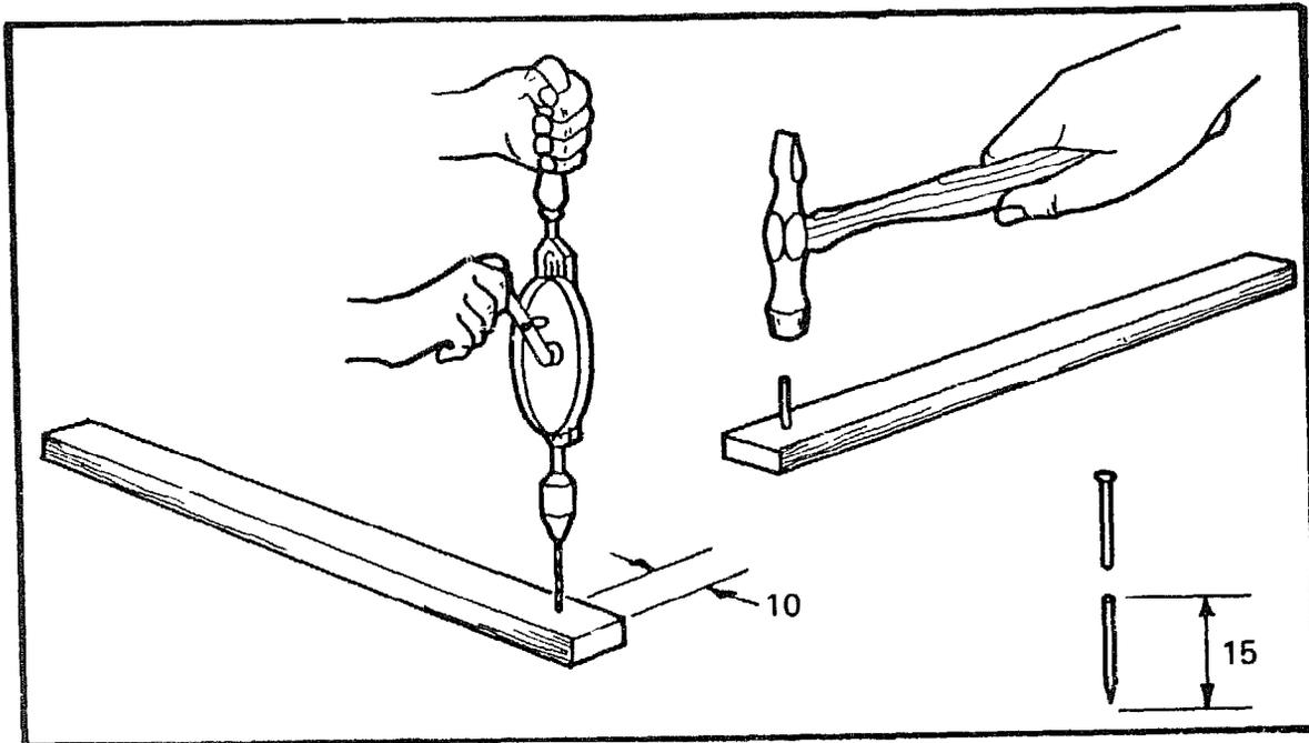
Take the timber prepared to 180mm × 10mm × 20mm, and using the same bit, drill a hole 10mm from the end of the timber. Cut a 25mm (1") nail down to 15mm.
