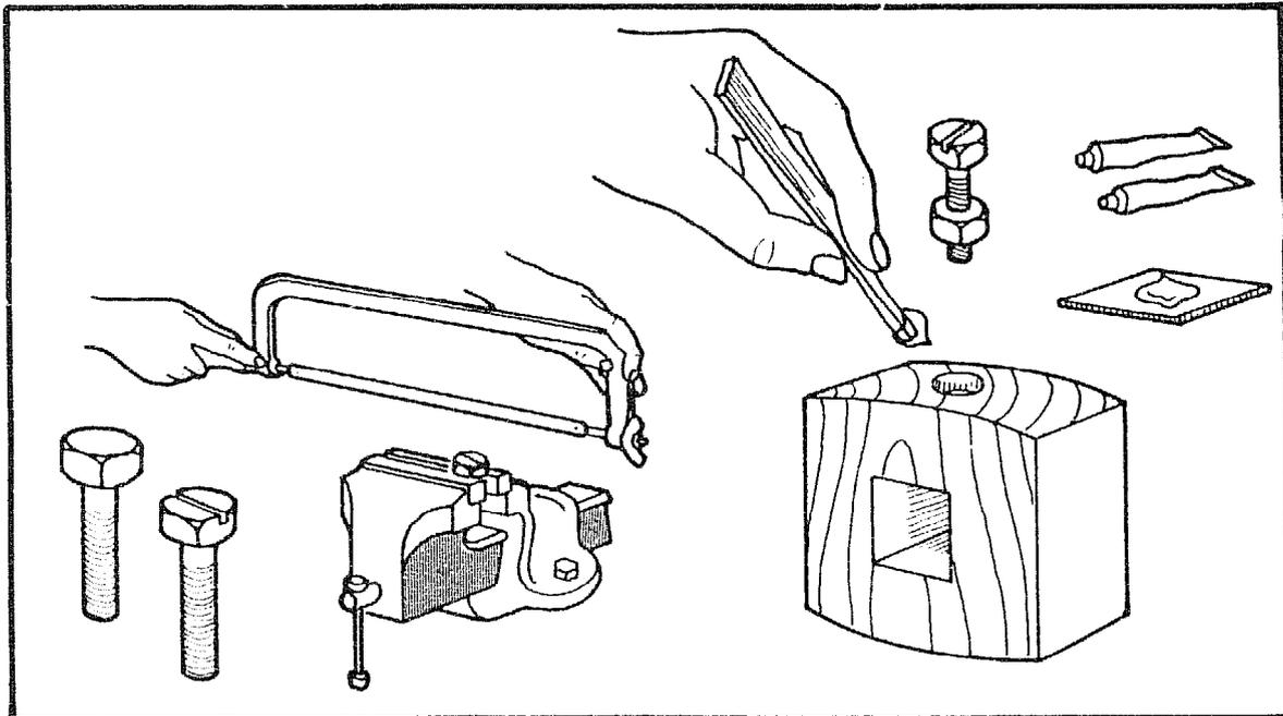
Take the 20mm  $\times$  6mm nut and bolt and saw a slot into the head for a screwdriver.
