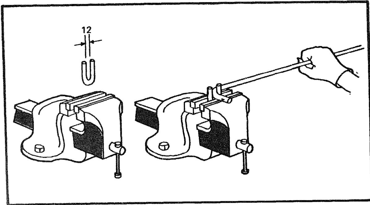
From a piece of 12mm rod make a 'U' shaped bending bar, with a 12mm gap between the uprights. Put this into a vice with about 20mm sticking out from the jaws. Heat up the end of the rod with the hole in and make a right angled bend 30mm from the end.
