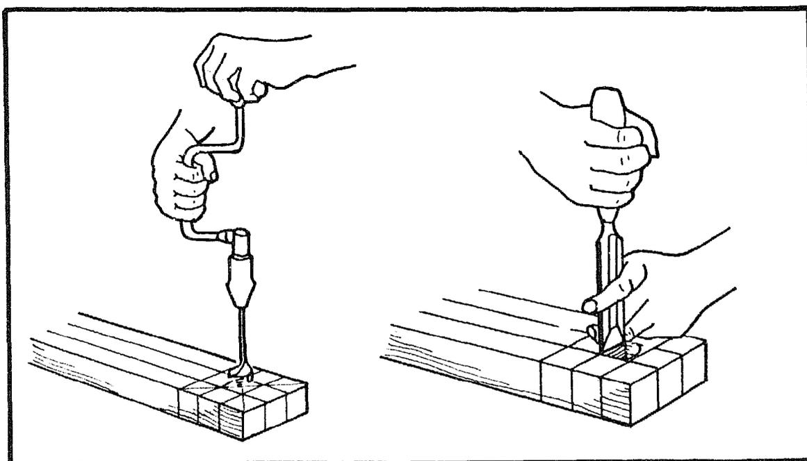
With a brace and bit, drill a  $\text{Ø}20\text{mm}$  hole exactly where the diagonals meet. Drill half way through, then turn the timber over to drill from the other side. Square the hole up to the gauge and pencil lines with a chisel.
