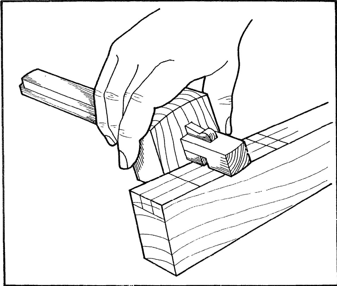
Mortise gauges are made with two spurs which mark two lines parallel to the edge of a workpiece, showing the position of a tenon or mortise or a similar joint. This avoids having to score two lines separately, and makes for greater accuracy. The spurs must be able to move independently, and be locked in any position by the fence. This makes it quite a difficult tool to construct.
