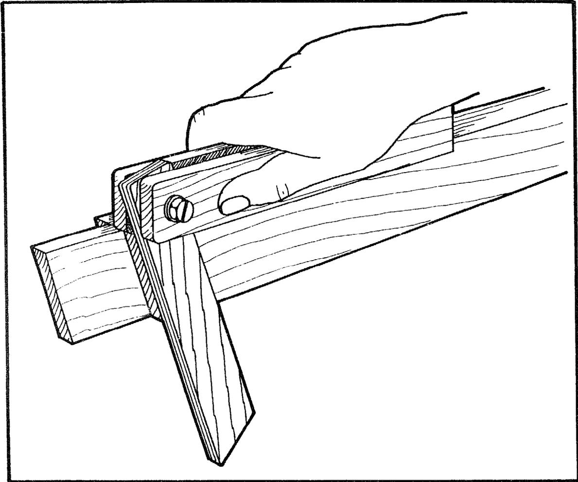
A bevel square, which is an essential tool for marking out dovetails and other joints with angles greater or smaller than 90 degrees, can be made on the same lines as the try square. Again the dimensions given are only for guidance.
