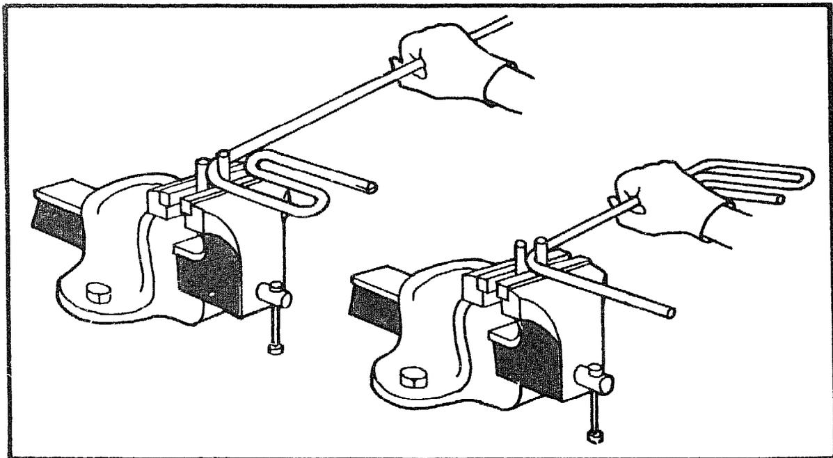
Heat the rod and make an 80 degree bend (see drawing of frame) so it just touches the first 180 degree bend. Heat the rod, measure 300m from the last bend and make one more 80 degree bend.
