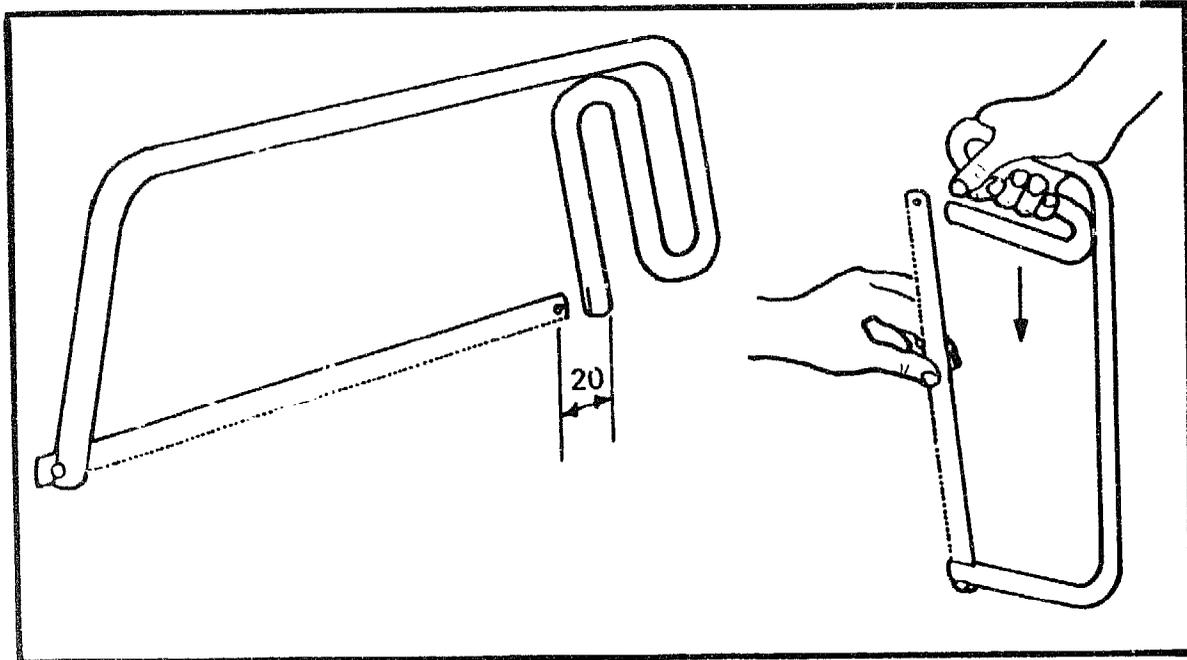
Bend the frame until the distance between the outside of the legs is 330mm. This gives the blade tension.
