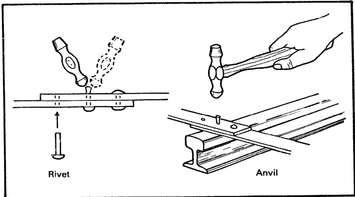
*Riveting.* This technique can be used to fix two pieces of metal, or sometimes a combination of wood and metal, together. Rivets can be bought or made from nails. They should be about 5mm longer than the thickness of the joint. Push the rivet through the hole, and spread the end by hitting it at differing angles round the head with a ball pein hammer.
