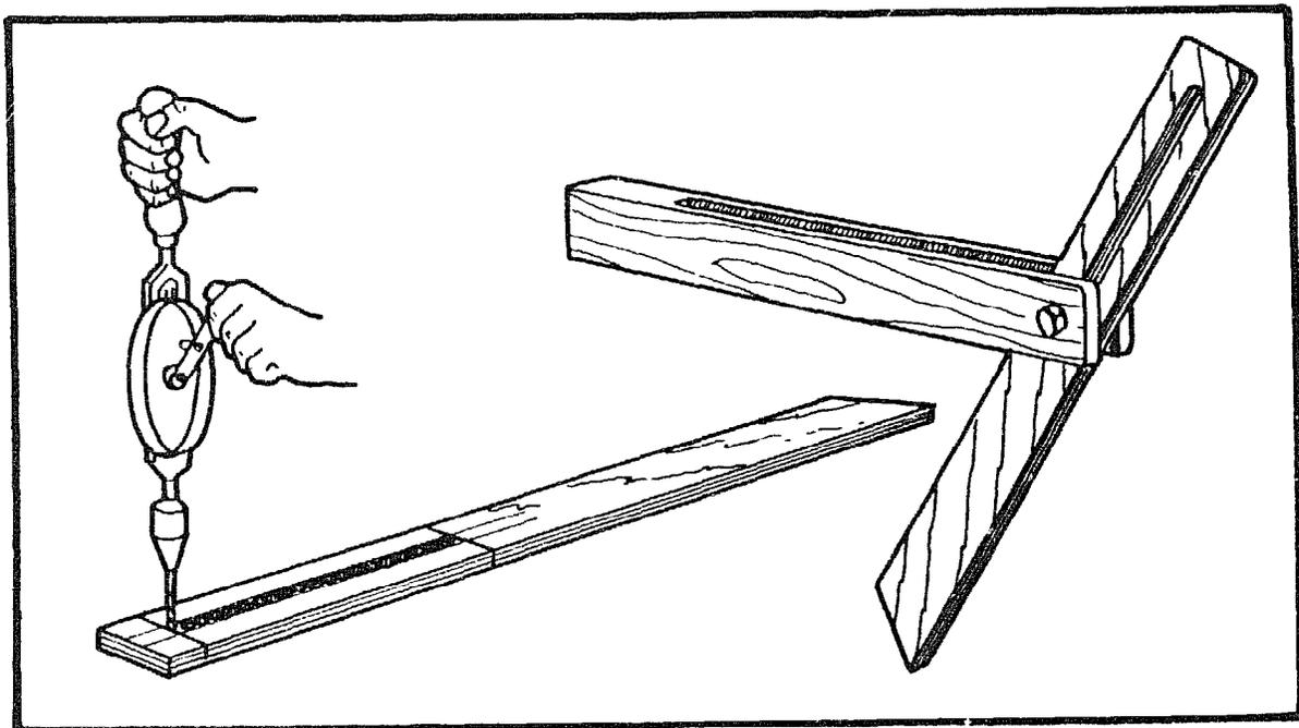
Drill a series of  $\varnothing 5\text{mm}$  holes between the gauge lines, clean out the waste with a chisel and file the slot smooth. Assemble the bevel square in the same way as shown on page 17.
