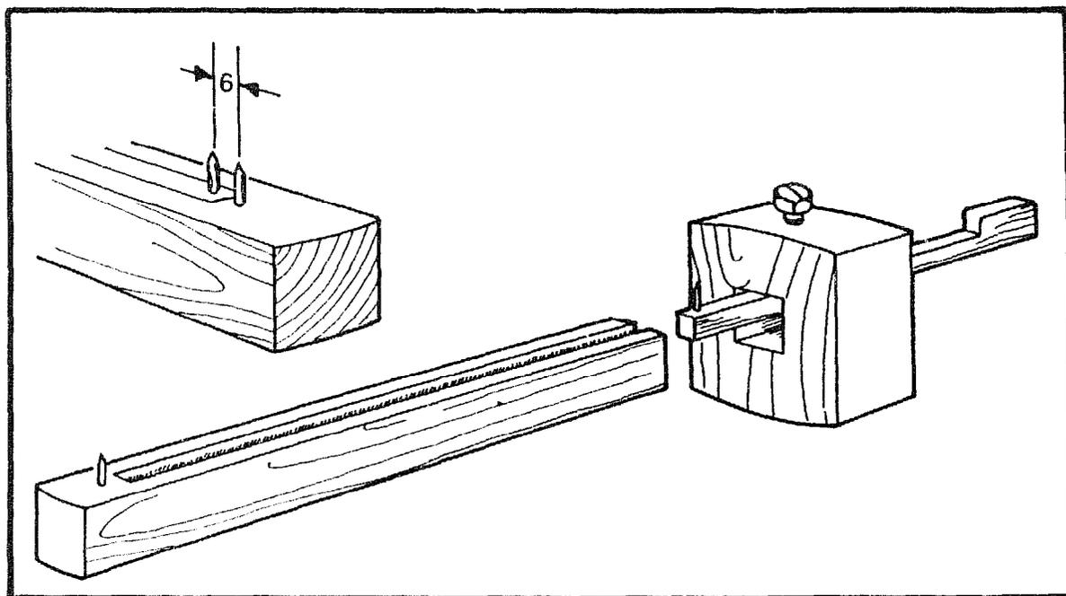
Fit the slider into the groove, so that the distance between the two spurs is 5mm. Sharpen the spurs with a file, and assemble the gauge.
