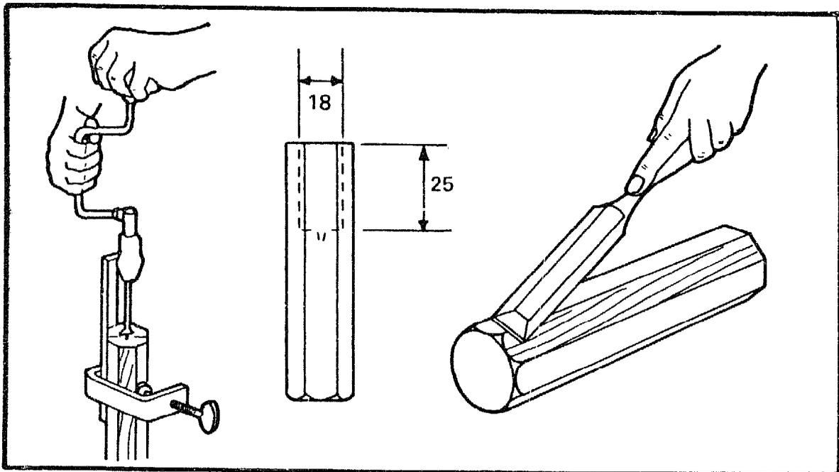
Where the diagonals meet, drill an  $\varnothing 18\text{mm}$  hole to a depth of 25mm.
