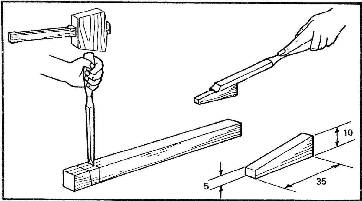
Cut the mortise between the pencil lines leaving a slope for the wedge. Make sure the ends of the mortise are straight.
