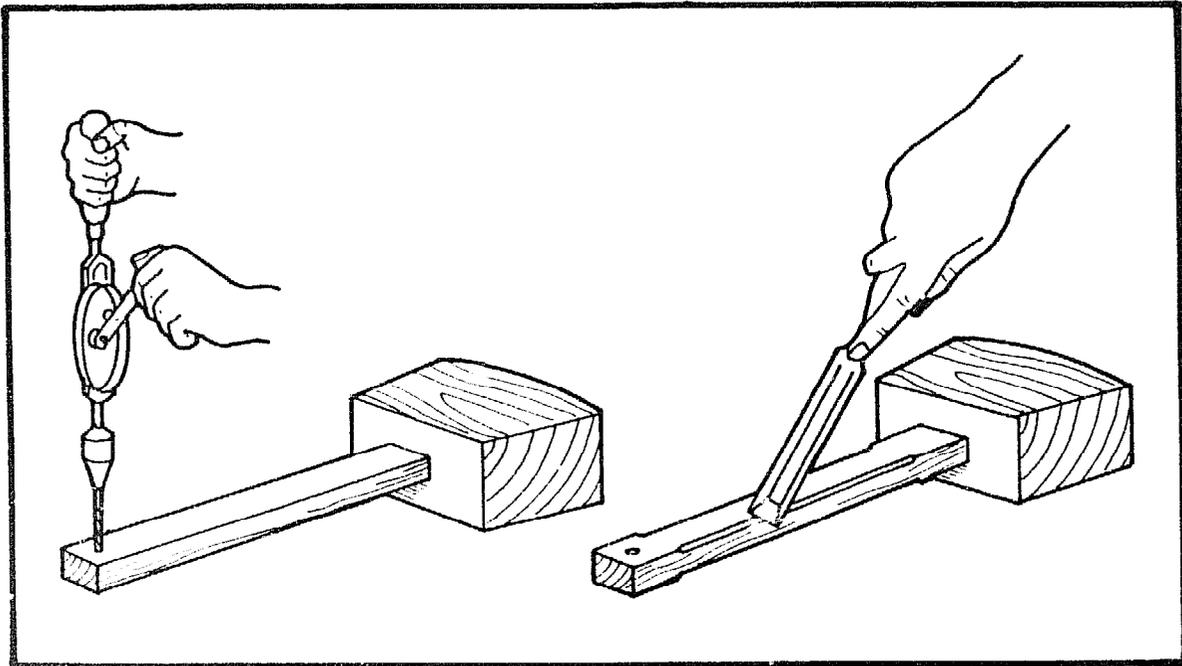
Drill a  $\varnothing 9\text{mm}$  hole in the end of the handle; this can be useful when storing the tool.
