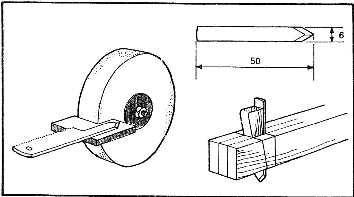
Grind a small piece of hacksaw blade to the dimensions shown, with a 'V' shaped bevel on the end. If you do not have a grinding wheel it can be filed, but first it must be heated until it is red hot, to soften the steel.
