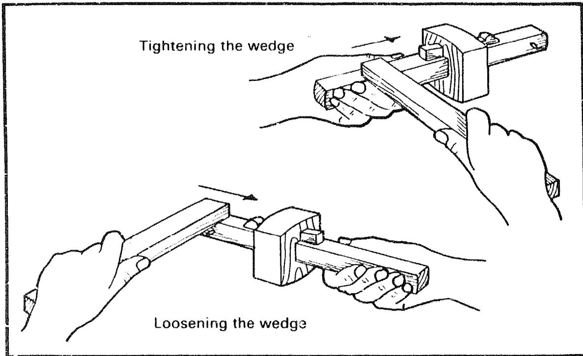
To use the gauge first set the distance from the spur to the fence. Tighten the fence to the stem by tapping the back of the wedge with a piece of wood. Check the setting and make final adjustments by tapping either end of the stem on the bench top.
