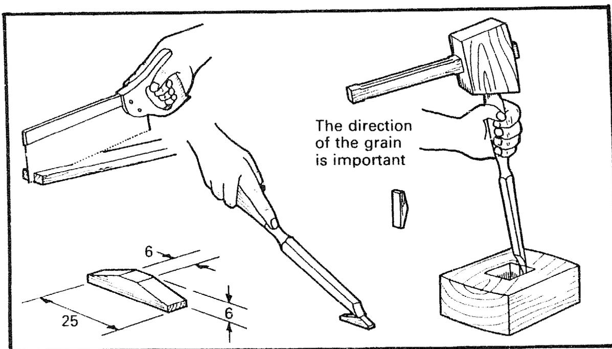
Cut and shape the shoe from the timber prepared to 200mm × 12mm × 6mm. With a mallet and 6mm chisel carefully cut a recess for the shoe in the end grain of the mortise, nearest the centre mark.
