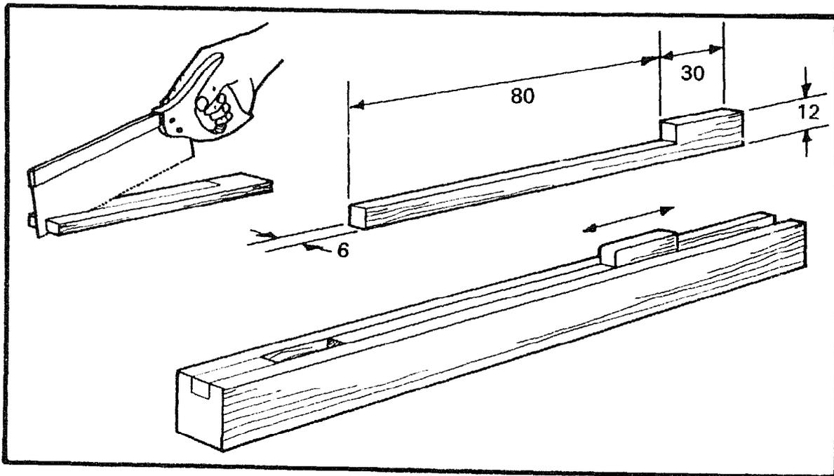
Cut the slider to the dimensions shown. Fit it into the groove. It should slide easily, but not wobble in the groove. The top of the slider can be scraped with a chisel so it is flush with the top of the stem.
