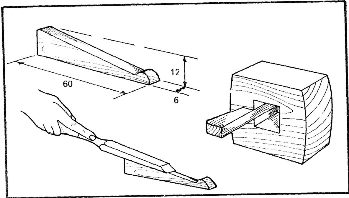
Cut the wedge to the dimensions shown; the knob at the end will stop it falling out and getting lost. Shape the wedge to fit into the groove in the fence.
