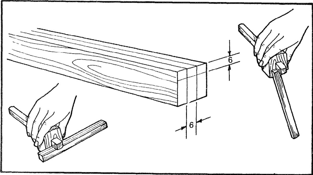
Take the timber prepared for the stem, and mark a 6mm groove down the centre of one side with a mortise gauge. Mark the depth at each end to 6mm.
