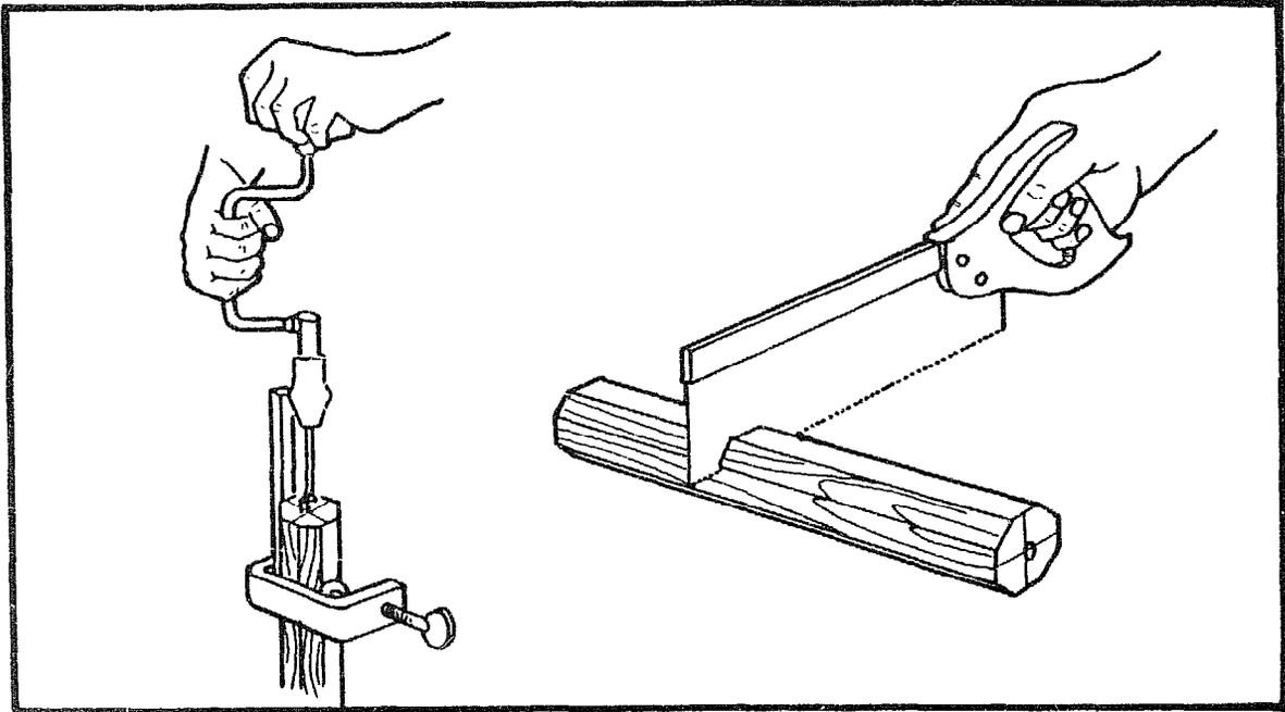
Drill a  $\text{\O}9\text{mm}$  hole in both ends, 50mm deep. Clamp a small piece of timber to the handle to help you to drill the hole straight. Saw the handle into two pieces, one 60mm long, the other 100mm long.
