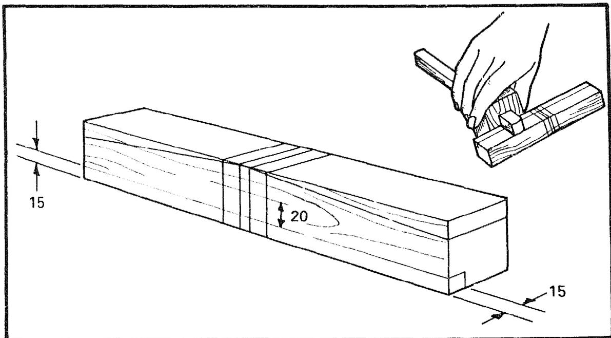
On one bottom edge gauge a 15mm × 15mm rebate. On the two sides gauge a line 35mm from the bottom edge, for the mortise.
